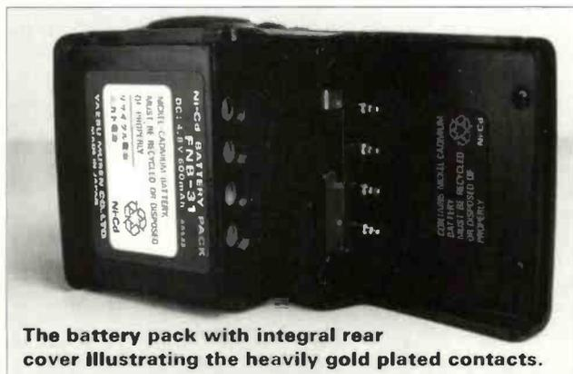
The battery pack with integral rear cover illustrating the heavily gold plated contacts.
