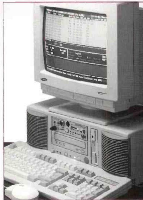
computer is fitted with some special hardware and software to customise it for amateur radio use. At the heart of this is the ShackMaster unit which is built into one of the disk drive bays on the computer front panel.
