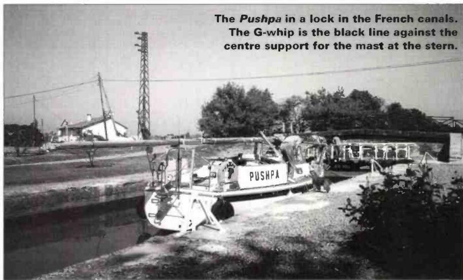
**The *Pushpa* in a lock in the French canals. The G-whip is the black line against the centre support for the mast at the stern.**
