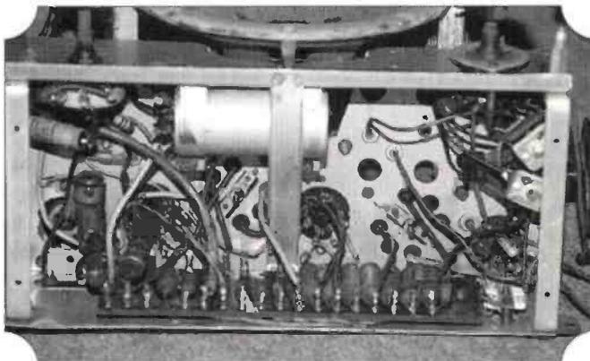
**Fig. 6: Both the Bush DAC90 and DAC10 receivers employed 'common can' electrolytic capacitors for smoothing purposes. In the DAC90, this photograph, the capacitor was mounted under the chassis (see text).**
