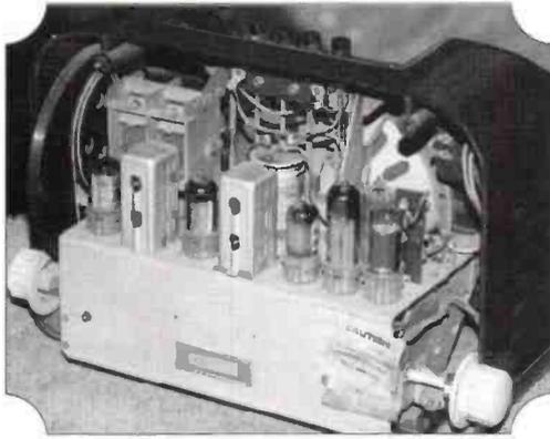
**Fig. 4: Inside view of Bush DAC10. Note the 'live chassis' warning (see text).**
