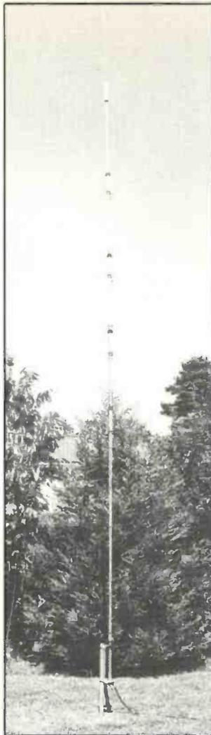
Before long, I had the RM-20S resonant on 14.160MHz, with the s.w.r. reading just above 1.1:1. This was with 360mm of tip protruding from the adjuster.
