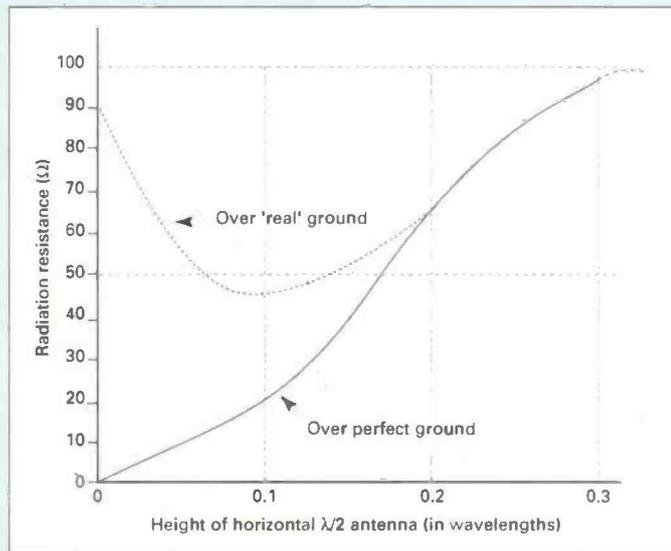
**Fig. 1: Graph showing the radiation resistance of half-wave dipoles over a perfect conductor and real ground. The actual curve of the impedance over real ground will vary from location to location, as the soil type varies. The curve shown here is only as an illustration and approximation.**
