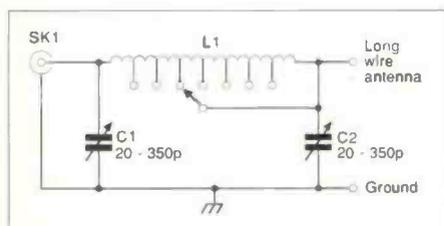
Fig. 1: Circuit of simple antenna tuning unit (a.t.u.) suitable for EC10 (see text).
