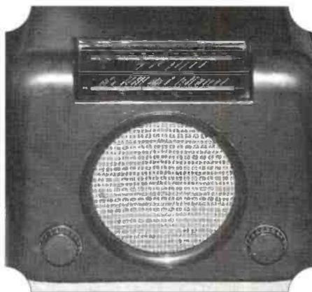
**Fig. 2: The Bush DAC10 used miniature glass-based valves (see text).**
