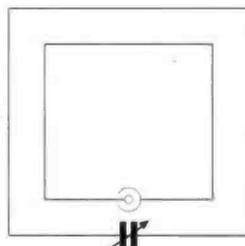
Fig. 4: A shielded small tuned loop antenna.
