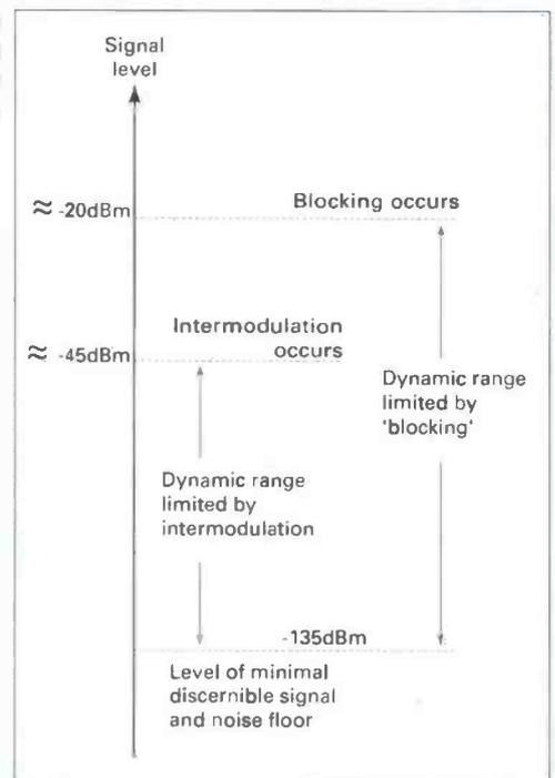
that might mask out the weak wanted ones. In this case the level of the intermodulation products must not be any greater than the m.d.s., i.e. no greater than the noise floor of the set. But again care should be taken to inspect exactly how the measurements are taken.
