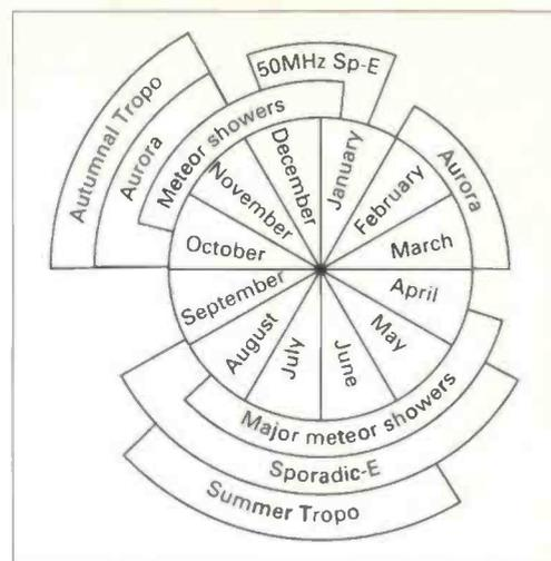
Fig. 1: Propagation modes chart by G4ASR (see text).
