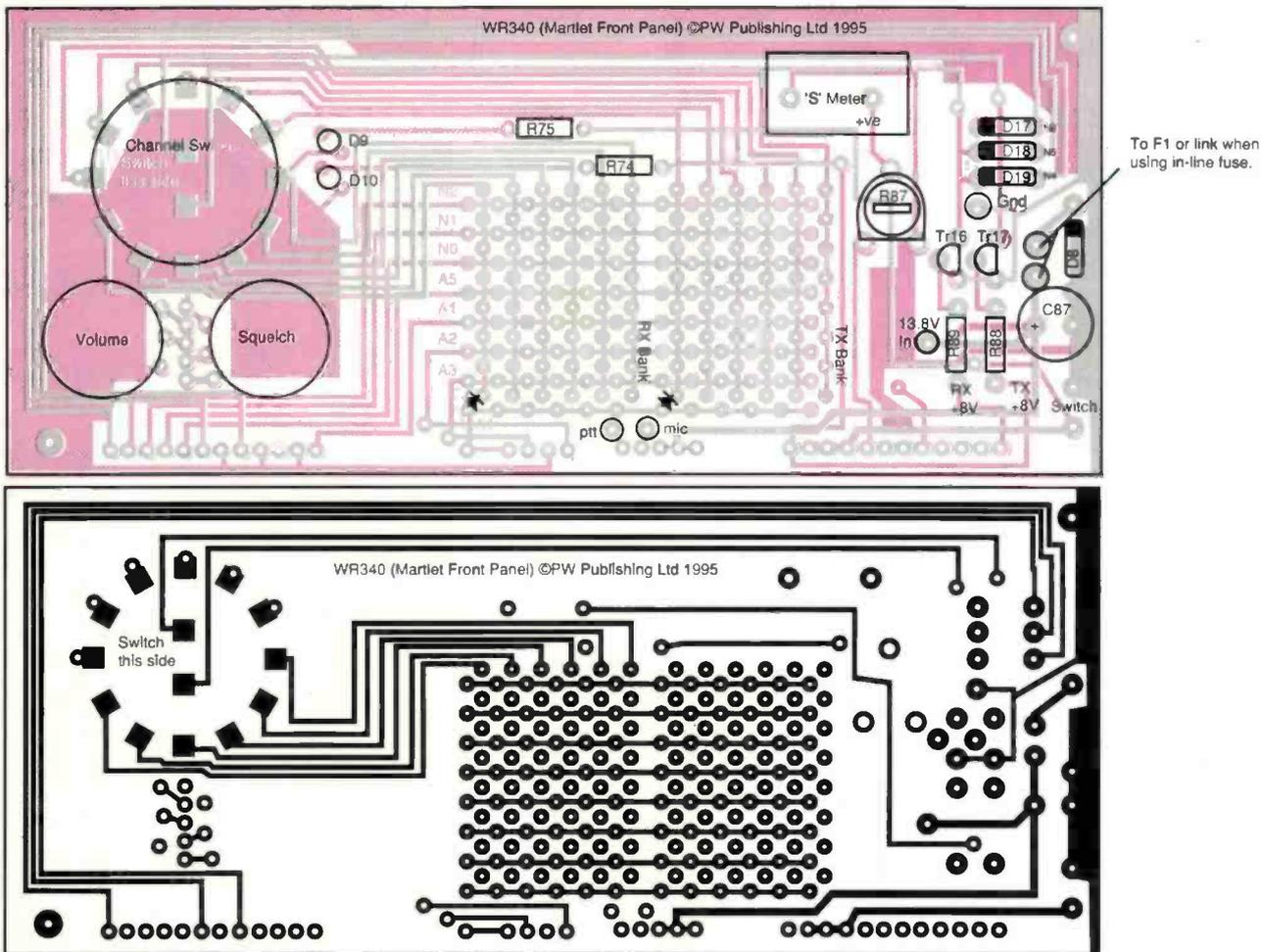
**Fig. 2: The PW Martlet front panel p.c.b. and associated component overlay. The special technique needed for installation of the channel selector switch is described in the 'Errors & Updates and Shopping List Extra' panel.**
