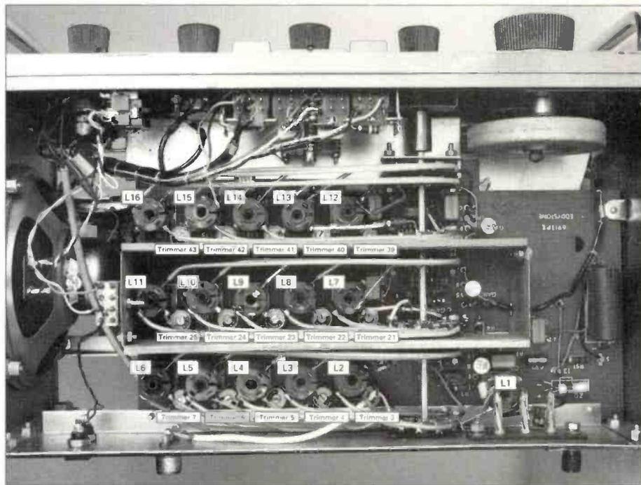
**Fig. 3: Annotated photograph showing location of inductors and trimmers for alignment purposes (see text and Table 1).**
