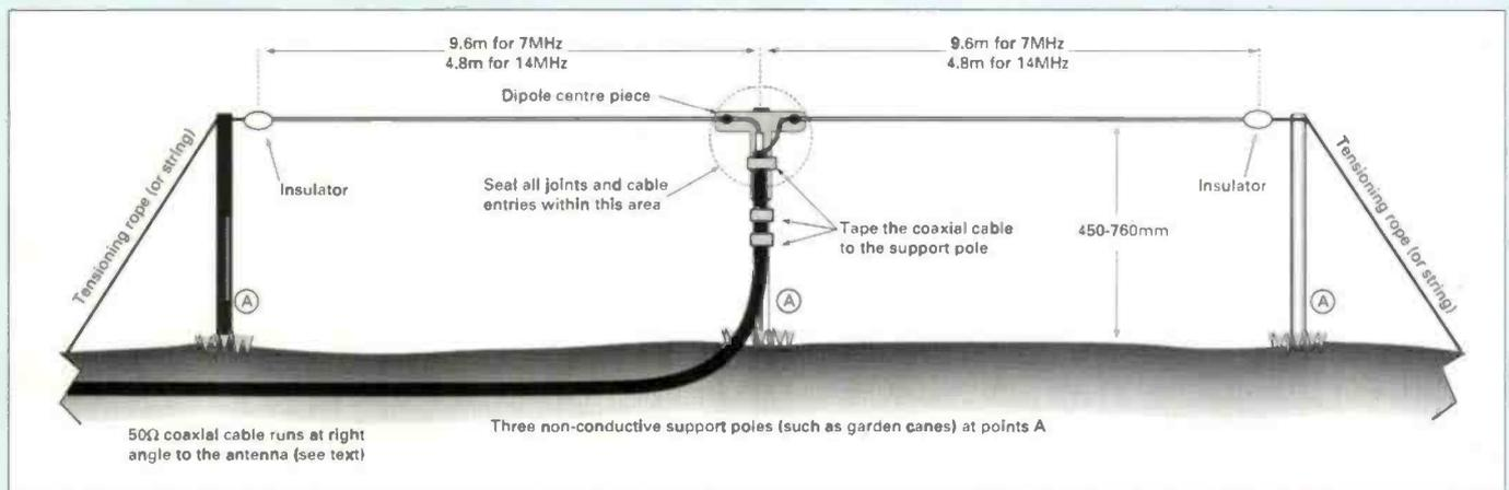
**Fig. 2: Practical arrangements for very low dipoles cut for 7 or 14MHz. The three support poles can be made from almost any non-conducting material such as garden canes, length of wooden dowelling or plastics material.**
