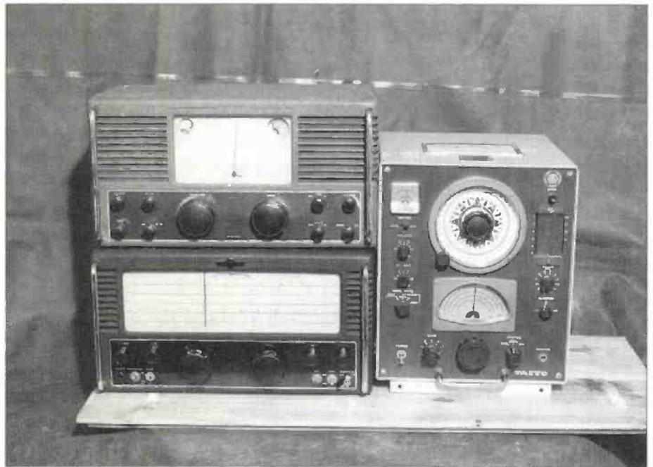
**Fig. 4: The two Eddystone receivers on the left (top to bottom) are the S504 and the S750. Pictured on the right is a marine a.d.f. receiver, which will (if supplied with the correct antenna), provide a directional bearing on the signal being received.**
