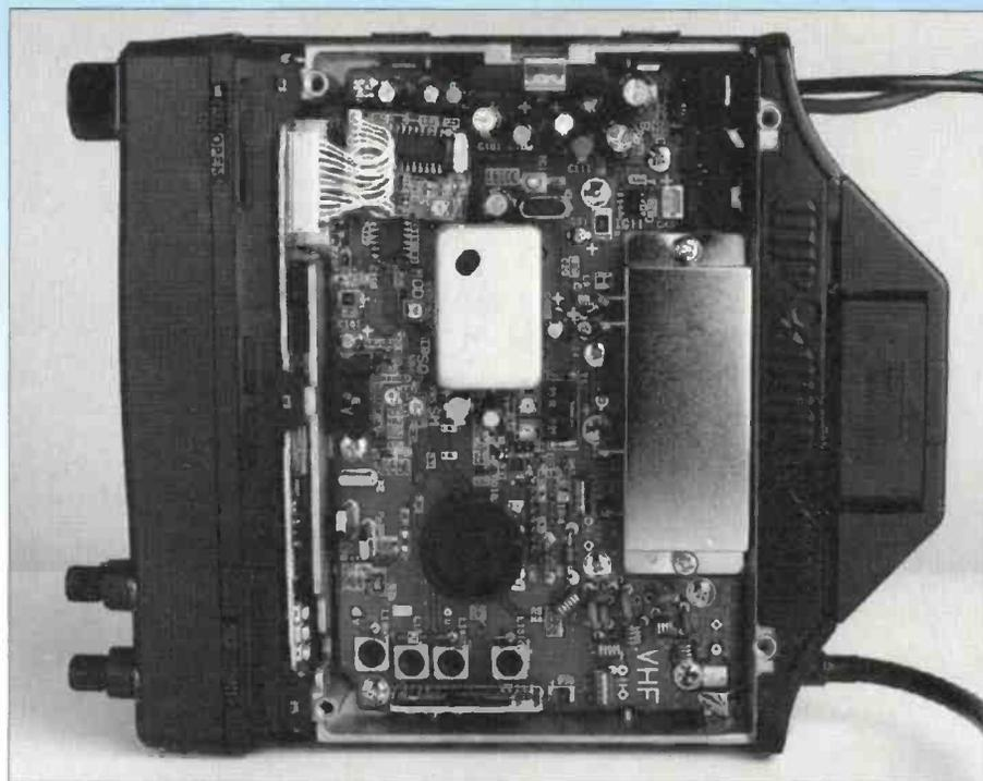
**Inside view of the v.h.f. side of the Alinco DR-610. The sloping-sided casing either side of the d.c. power input and the single antenna connection, houses the cooling fan. The u.h.f. unit is on a similar board mounted on the other side of DR-610.**
