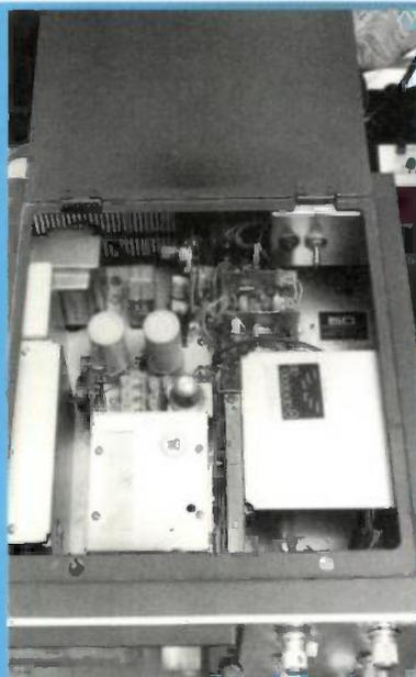
Fig. 3: Photograph illustrating the inside cabinet view of the JR-599 receiver. The built-in 144MHz converter can be seen at the top centre right, with space for the optional 50MHz converter alongside (see text).
