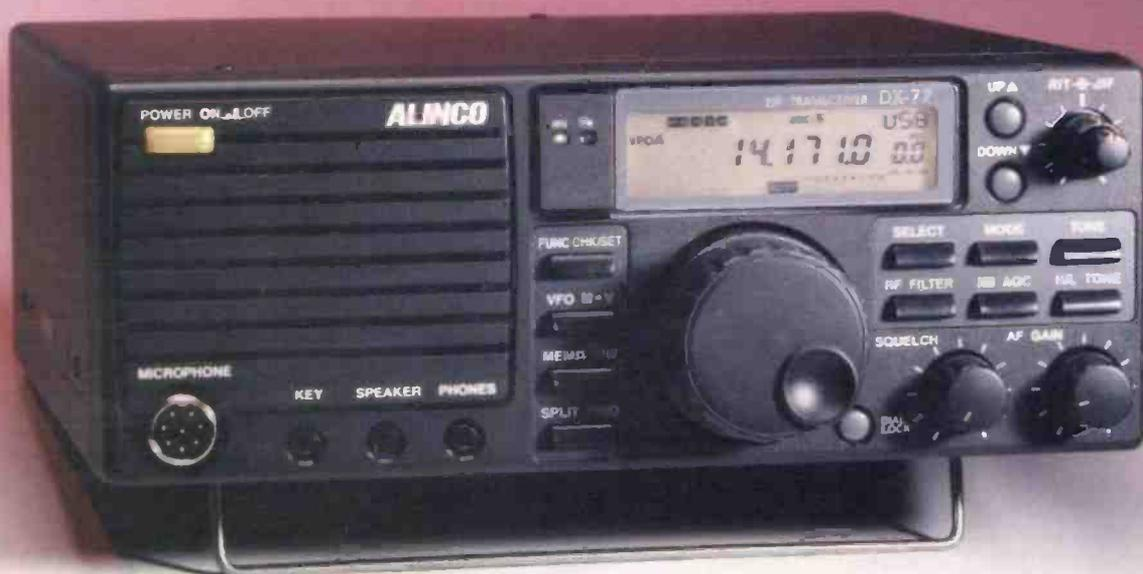
77 has a front mounted speaker with a louvered type speaker fret. The main tuning knob is slightly off-set from centre right - and this I found a delight to use. It felt very good, smooth in operation and I'm sure it will appeal to many 'natural' left-handers. (The DX-70 has a main tuning control on the far right - which makes this control one of the only awkward features for operation by G3XFD!).
