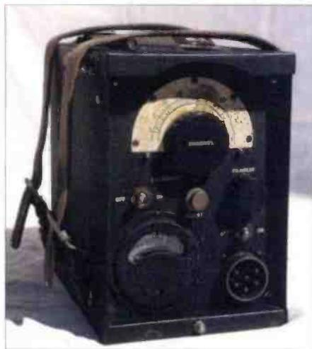
Fig. 4 (right): The French produced Second World War R30 receiver. Note the tuning dial, marked in Metres, and the antenna socket on the right (see text).
