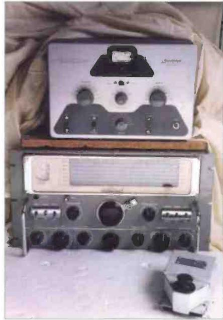
**Fig. 1: The Heathkit DX-20 transmitter photographed in place above the GEC BRT-402 receiver, with the Morse key ready for action. (see text).**
