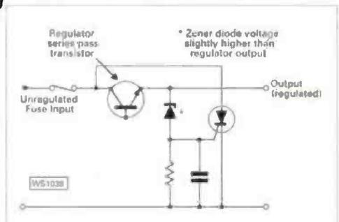
Fig. 4: A 'bare-bones' over-voltage protection circuit (see text).
