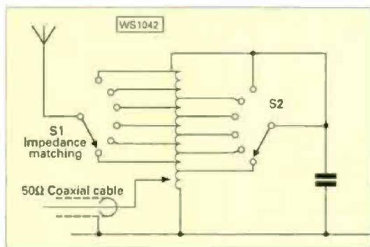
Fig. 5: A slight modification to the a.t.u. of Fig. 4, can sometimes improve the range covered,
