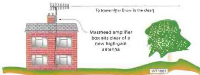
**Fig. 2:** An amplifier placed correctly, as illustrated, will optimise the incoming signal and introduce the least possible degradation to the outgoing signal to the TV receiver. Taken note that 'wideband' amplifiers in mast head applications should always be avoided because of poor EMC problems and 'channelised' amplifiers, suitable for the channel grouping being received must always be the preferred choice (see text).
