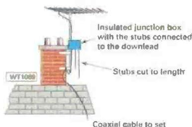
**Fig. 4:** Coaxial 'stub' filters are very easy to make and although they can take a little time to set up - can provide useful reduction of strong adjacent channel and 'out of band' transmissions such as those from the 144 and 430MHz amateur bands. The 'stubs' are shown cut to length and before the cut ends are sealed before being rolled up and secured under the junction box (see text).
