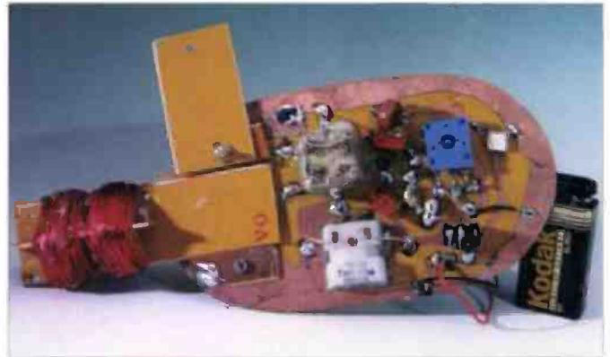
**Fig. 3: Underside view of one of the prototype 'Tinny Dippers'. See text for important instructions regarding the coil mounting 'saddle' and earthing technique.**
