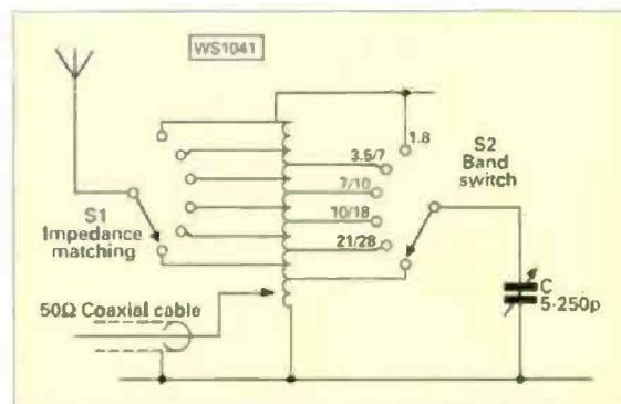
Fig. 4: Adding two multi-pole switches makes choosing the best tapping and tuning points easy.
