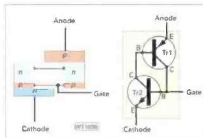
Fig. 2: The four layers may be considered as two inverse connected transistors (see text).
