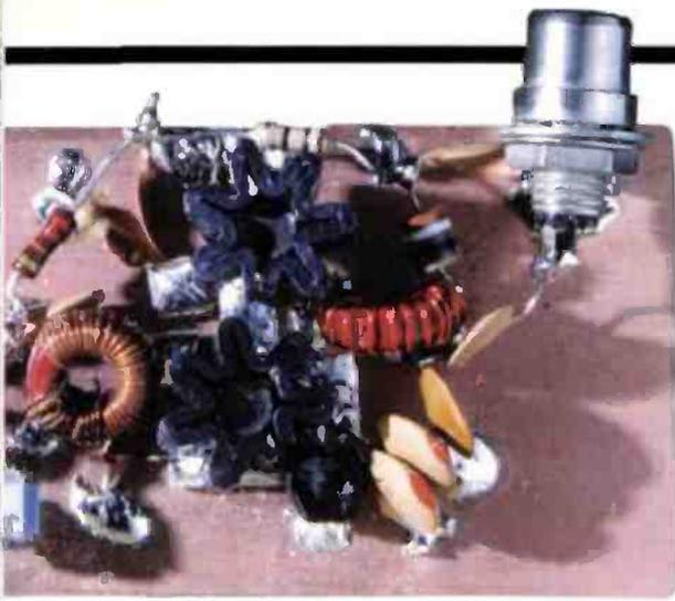
This month's project (or should it be challenge?) - features the 'mighty' 2N2222 transistor in a QRP 7MHz transmitter.
