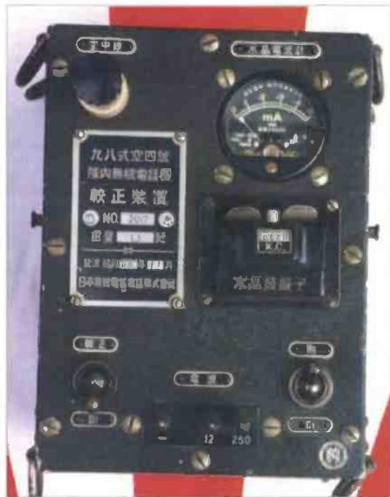
Fig. 3: The Japanese 'puzzle' (crystal checker?). The crystal plugs in just below the meter (see text).
