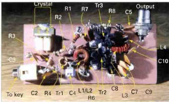
inductance value for L1 is 6μH and this resonates on 7.030MHz (the QRP Calling Frequency) with a capacitor of about 85pF. I used a trimmer I found in the junk box.
