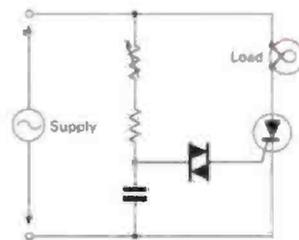
Fig. 3: The bare circuit details of a light dimmer circuit (see text).
