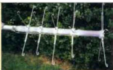
Fig. 3: The resonator adjusters: The resonator elements, showing construction of the resonators with their spokes and adjusters.
