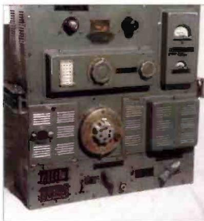
Fig. 1: The Saram 3-10 transmitter. The two doors either side of the large central tuning dial open to reveal the valves for the set.
