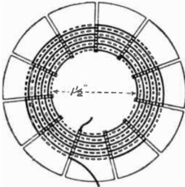
FIG. 126.—The Coil ready for mounting.
