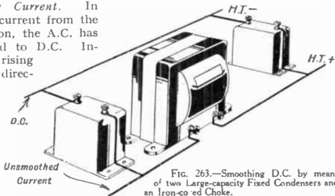
FIG. 263.—Smoothing D.C. by means of two Large-capacity Fixed Condensers and an Iron-coiled Choke.
