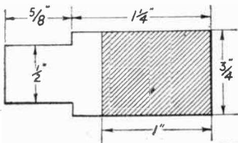
FIG. 156.—Size and shape of the copper foils. The additional area on the left enables the plates to be joined together.
