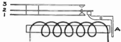
FIG. 234.—Diagram of the Switch in the relay.
