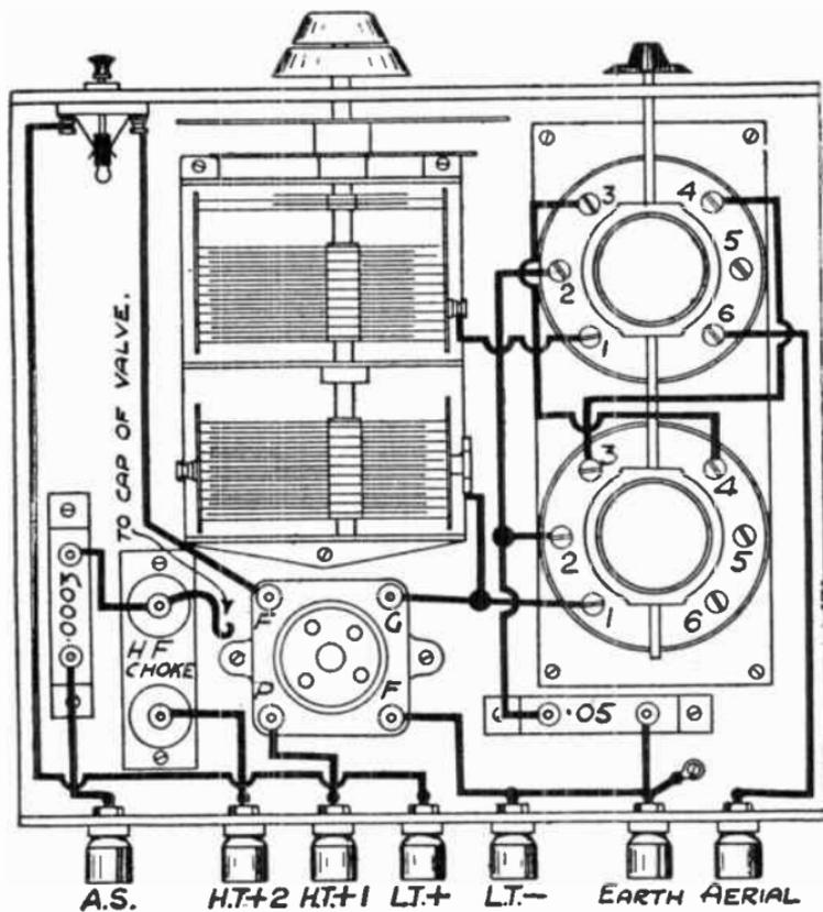
FIG. 181.—The wiring diagram of the D.X. Unit.
