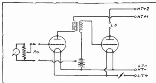
FIG. 207.—Theoretical Circuit of Two-Valve Gramophone Amplifier.
