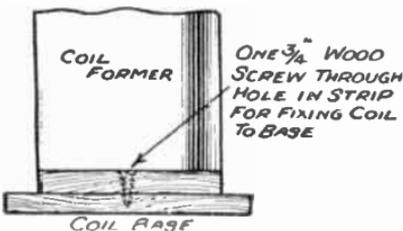
FIG. 135.—The Coil fixed to the base.
