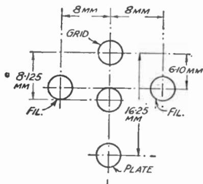
FIG. 458.—Valve-leg spacing for 4- and 5-pin valves. The diameter of the valve pins is 3.2 mm.
