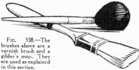
FIG. 338.—The brushes above are a varnish brush and a gilder's mop. They are used as explained in this section.
