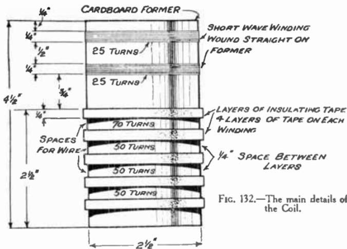
FIG. 132.—The main details of the Coil.
