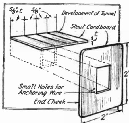
FIG. 221.—How to make the winding bobbin from paxolin sheet for chokes and transformers.
