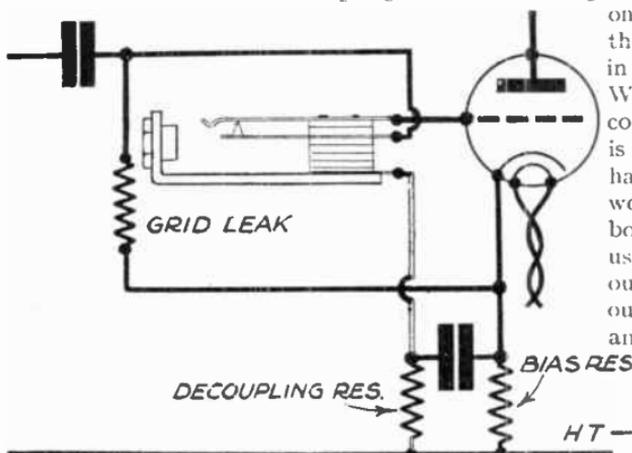
FIG. 336.—The mains version of Fig. 335. Note grid bias is cut out when the radio is in use.
