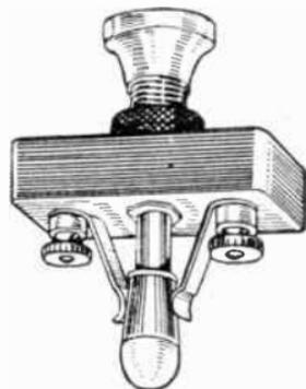
FIG. 376.—On-off Switch.
