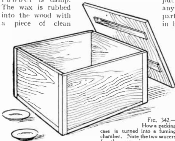
FIG. 342.—How a packing case is turned into a fuming chamber. Note the two saucers for the ammonia.
