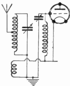
FIG. 450.—Inductive Band-pass Coupling.
