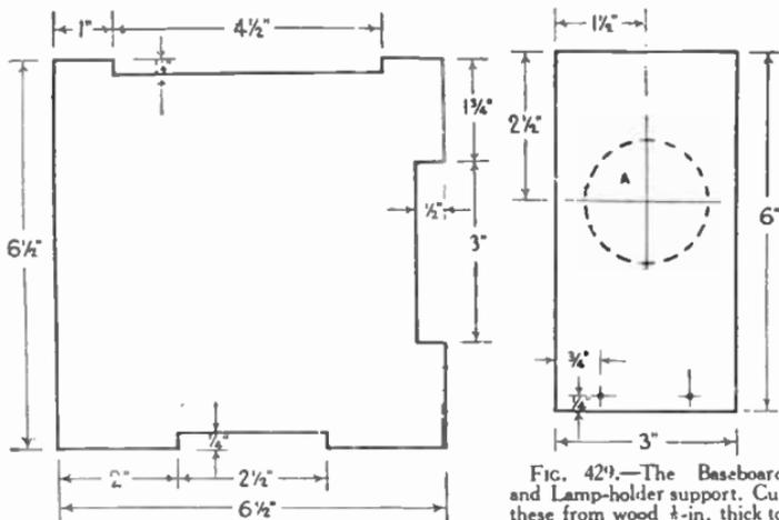
FIG. 429.—The Baseboard and Lamp-holder support. Cut these from wood  $\frac{1}{8}$ -in. thick to the dimensions given in the diagram. The position of the lamp-holder is shown at A.
