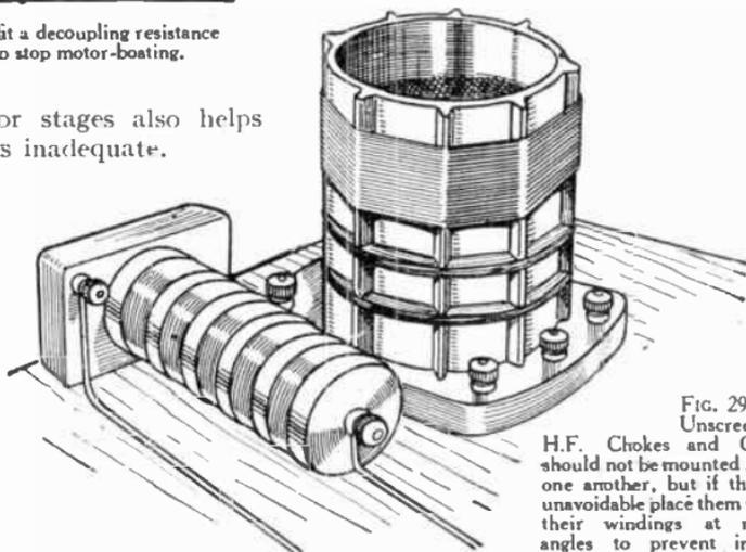
FIG. 298.—Unscreened H.F. Chokes and Coils should not be mounted near one another, but if this is unavoidable place them with their windings at right angles to prevent interaction and H.F. howling.
