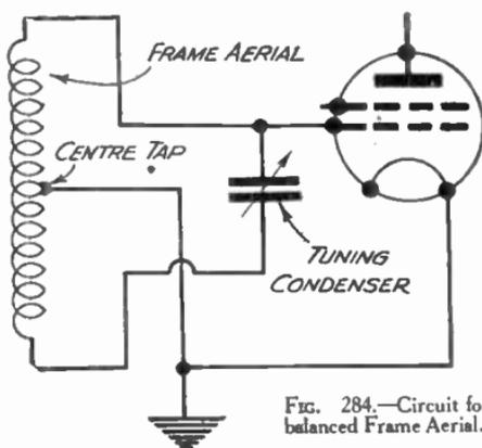
FIG. 284.—Circuit for balanced Frame Aerial.
