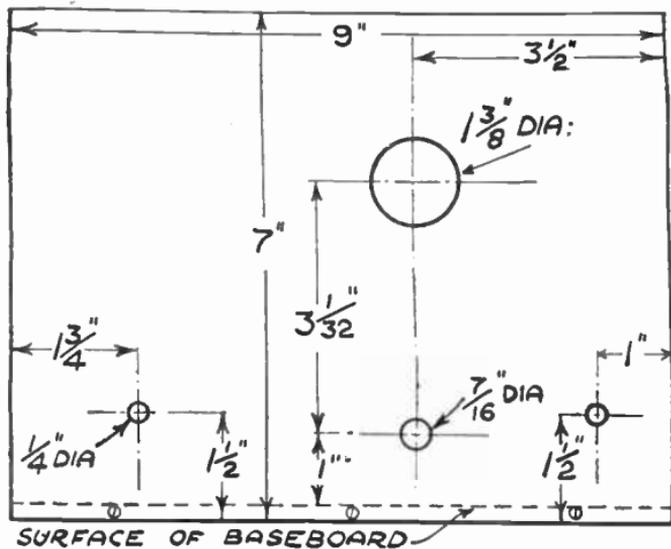
FIG. 182.—The Panel Layout for the D.X. Unit.
