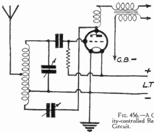
FIG. 456.—A Capacity-controlled Reaction Circuit.
