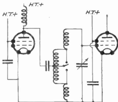
FIG. 452.—Wave-change Switching of Parallel-fed Tuned Grid Circuit.
