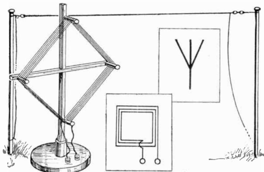
FIG. 40.—Conventional signs for outdoor and frame aerials, shown also pictorially.
