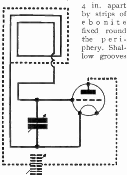
FIG. 196.—The Connections for a Frame Aerial: the dotted lines show the additional connections for capacity-controlled reaction.
