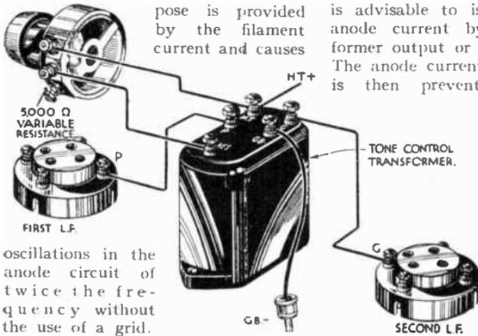
FIG. 261.—Tone-control Transformer Coupling.
