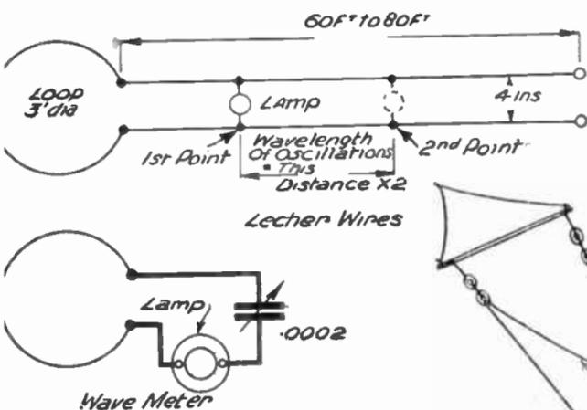
FIG. 198.—The Lecher-wire circuit used for calibration purposes. The upper loop is connected to the oscillator, whilst the lower one is in circuit with a lamp which glows to indicate resonance. (See Lecher Wires.)
