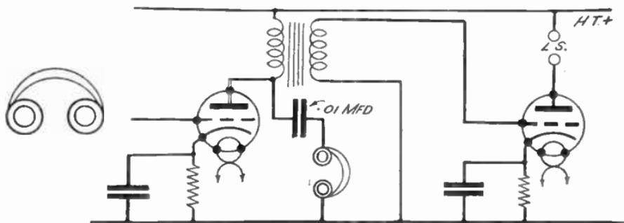
FIG. 404.—Theoretical illustration of Headphones and method of using phones with a mains set.
