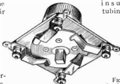
FIG. 391.—Another form of Rotary Switch.
