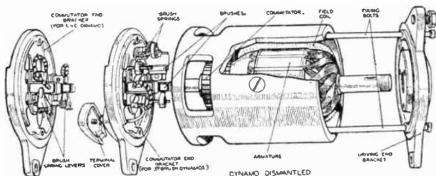
FIG. 12.—A car lighting dynamo, showing construction.
