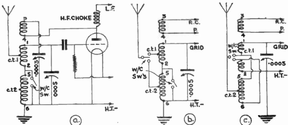
FIG. 435.—Three methods of connecting the Tuner shown in Fig. 434 into a Detector Circuit.
