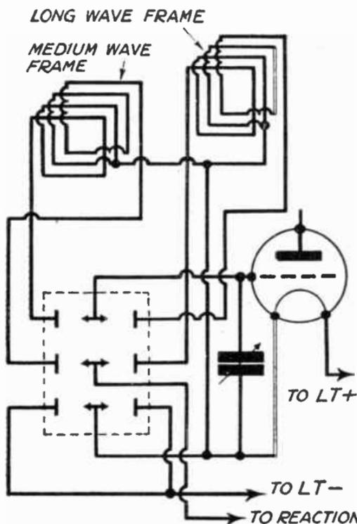
FIG. 384.—Three-pole change-over Switch used for wave changing with Frame Aerials.
