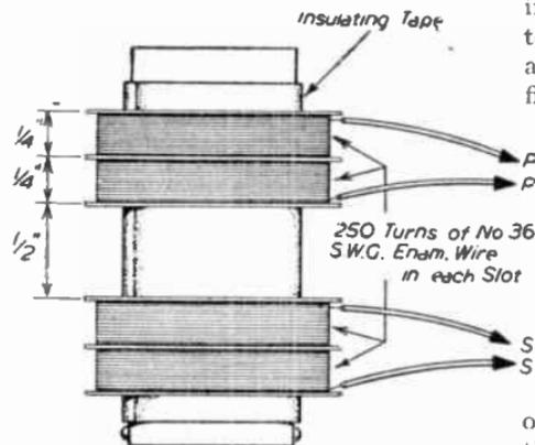
FIG. 150.—Constructional details of an I.F. transformer for 110 kc/s.
