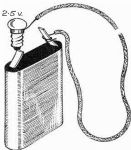
FIG. 187.—The simplest form of Tester.
