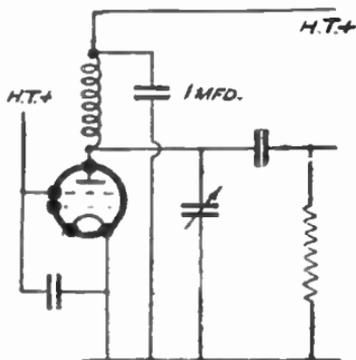
FIG. 446.—Another form of Tuned Anode Coupling.
