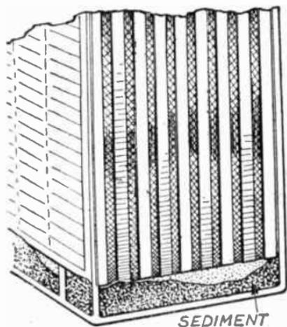
FIG. 22.—Sediment should be removed periodically, to prevent short-circuiting of plates.
