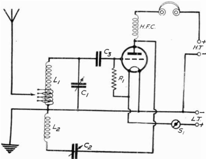
FIG. 100.—Circuit No. 3: Another simple One-valve Set.
