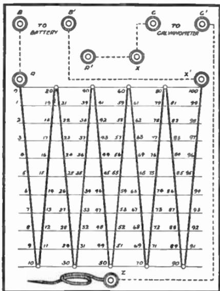
FIG. 483.—A detailed sketch of the Wheatstone Bridge, showing its construction.
