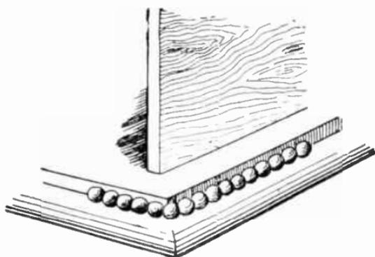
FIG. 74.—The base is improved by the addition of beading glued in the corner angle of the two parts.
