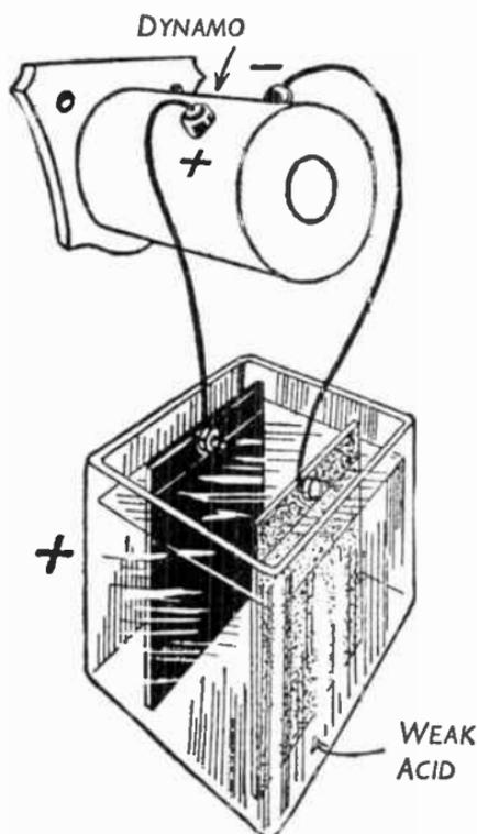
FIG. 26.—Method of testing a Dynamo for Polarity.
