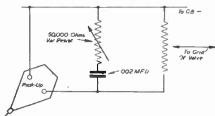
FIG. 360.—Circuit for Eliminating Scratch.
