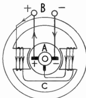
FIG. 15.—A constant voltage dynamo.
