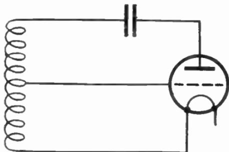
FIG. 55.—Autodyne Circuit.
