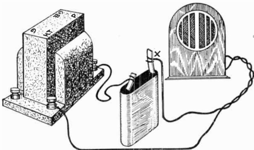
FIG. 188.—The way to test a Transformer Winding.
