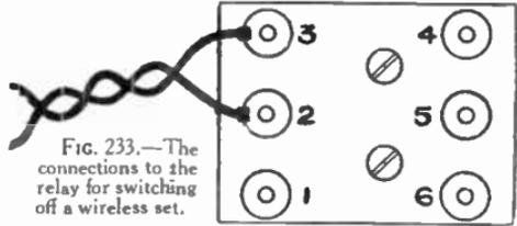
FIG. 233.—The connections to the relay for switching off a wireless set.
