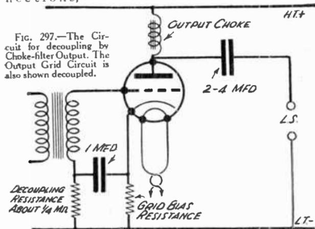
FIG. 297.—The Circuit for decoupling by Choke-filter Output. The Output Grid Circuit is also shown decoupled.
