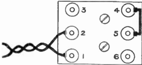
FIG. 232.—The connections to the relay for a burglar alarm.
