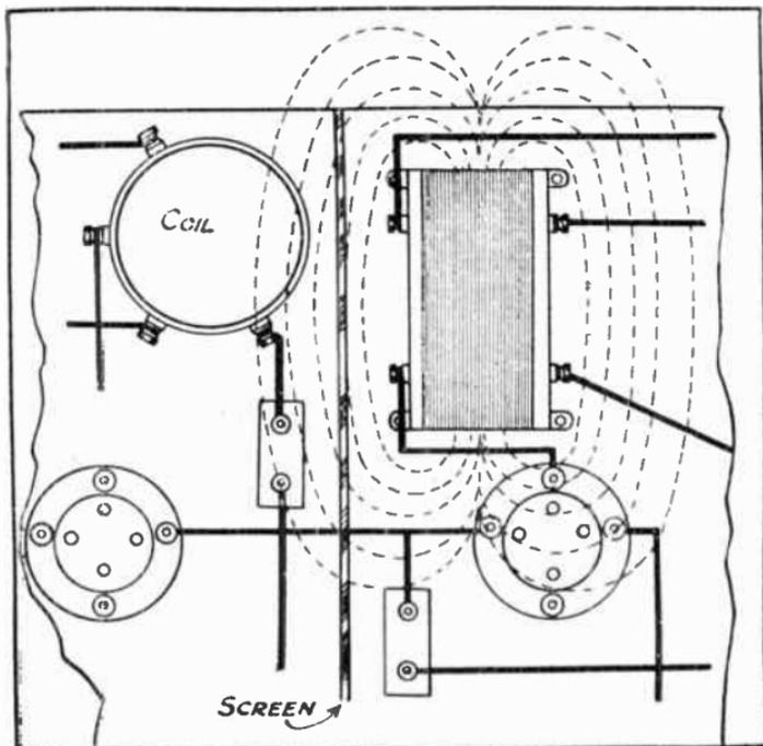
FIG. 226D.—The placing of a Transformer near a Coil (even if there is a Screen) is bad.
