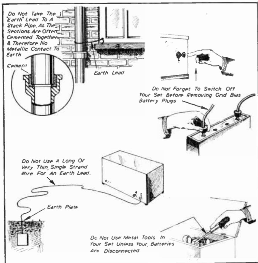
FIG. 302.—Various simple tests to apply, and causes of trouble.
