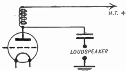
FIG. 191.—The Filter Circuit. (See also Fig. 354.)
