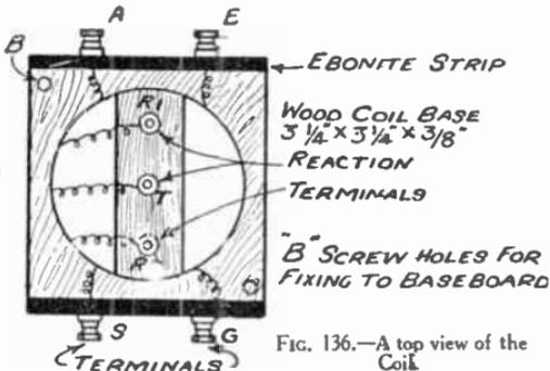
FIG. 136.—A top view of the Coil.
