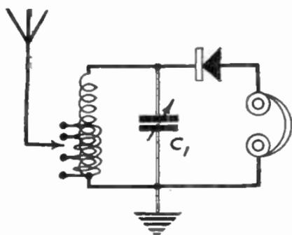
FIG. 96.—Crystal Circuit using tapped coil.
