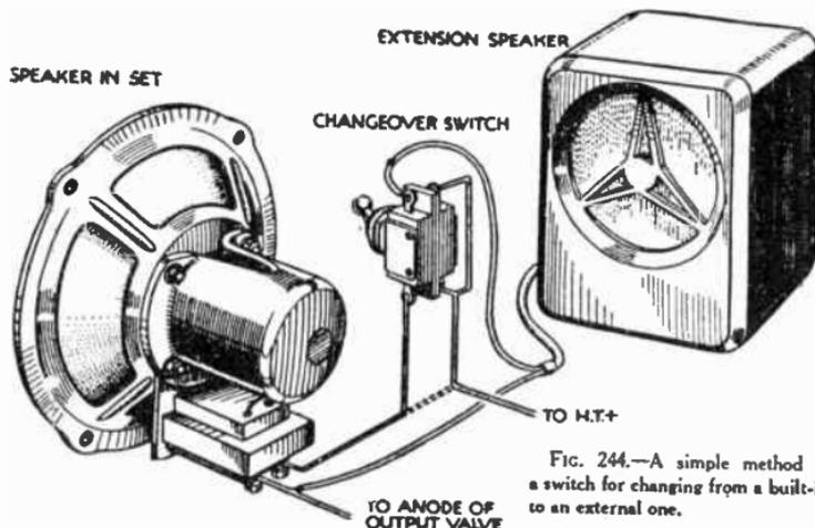
FIG. 244.—A simple method of fitting a switch for changing from a built-in speaker to an external one.
