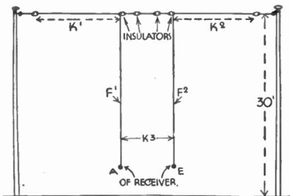
FIG. 197B.—A divided aerial:  $K^1$  and  $K^2$  are equal in length to half the wavelength.  $K^3=4\frac{1}{2}$  inches.
