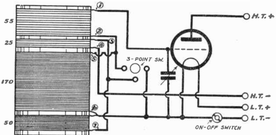
FIG. 480.—Diagram of coil connections for the Heterodyne Wavemeter shown in Fig. 481.
