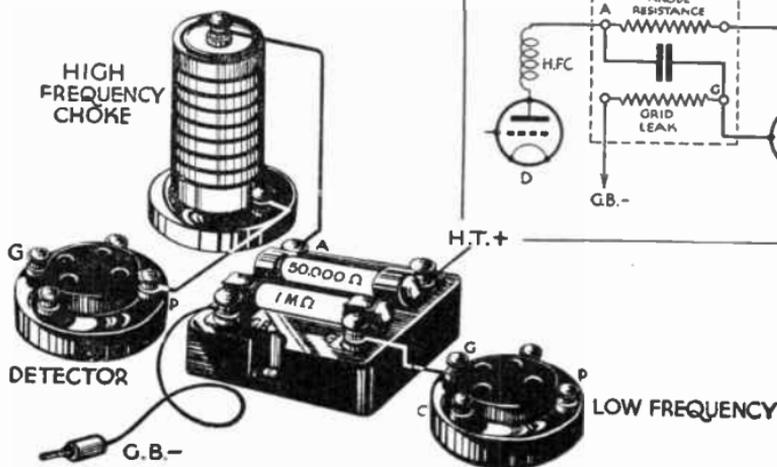
FIG. 256.—Resistance-capacity Coupling.
