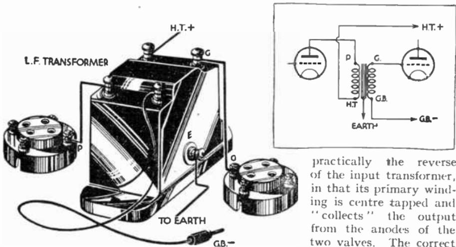
FIG. 258.—L.F. Transformer Coupling.
