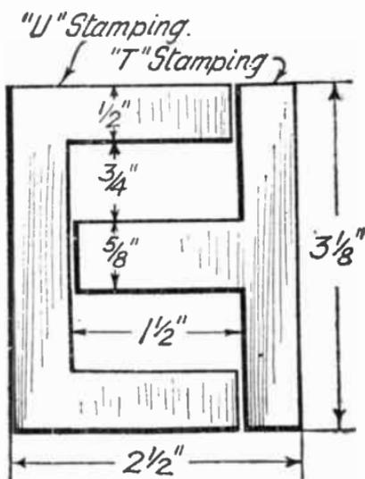
FIG. 220.—Standard "U" and "T" stampings, with dimensions, for use in L.F. chokes and various transformers.
