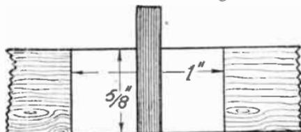
FIG. 323.—The Mould for casting the weights.
