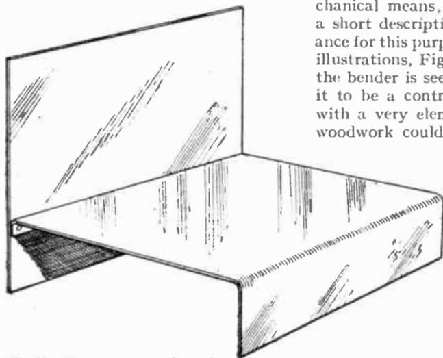
FIG. 89.—The most common form of metal Chassis. Note how the panel is bolted to the front.
