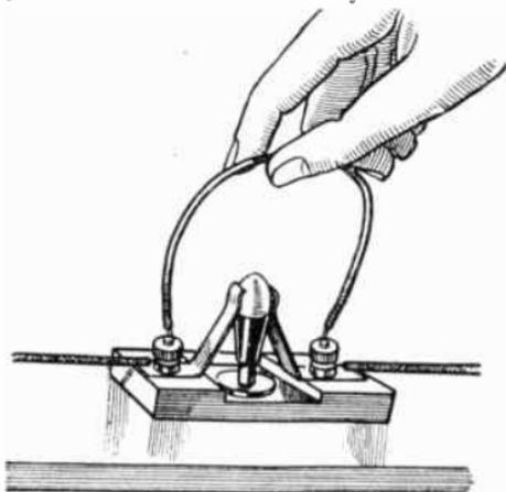
FIG. 301.—Shorting a Switch in this manner will indicate whether crackling noises are due to faulty contact.
