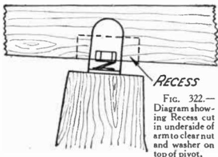
FIG. 322.—Diagram showing Recess cut in underside of arm to clear nut and washer on top of pivot.
