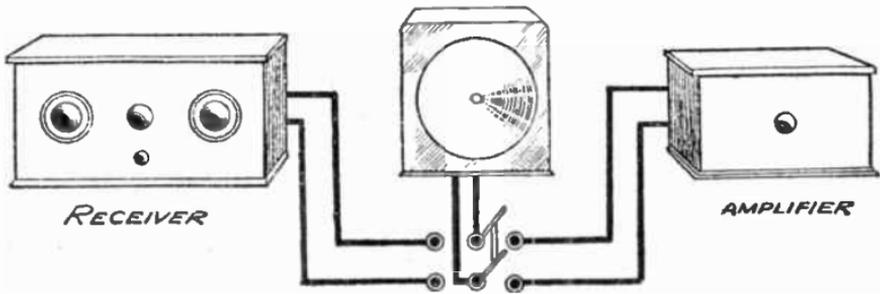
FIG. 206.—How the Gramophone Amplifying Apparatus is connected.
