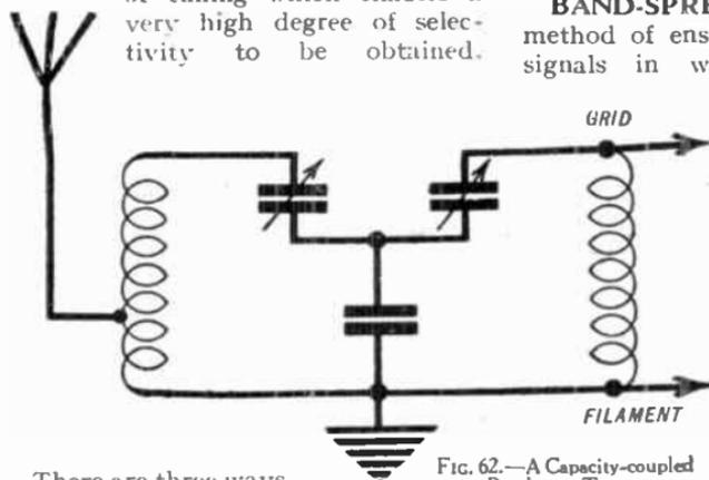
FIG. 62.—A Capacity-coupled Band-pass Tuner.
