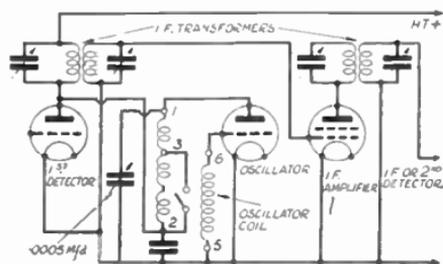
FIG. 152.—Connections for an oscillator coil in a standard circuit.
