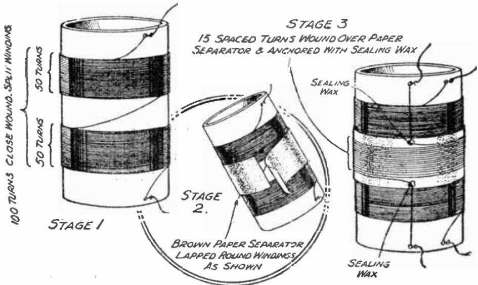
FIG. 49A.—Constructional details of the transformers for anti-interference aerials.
