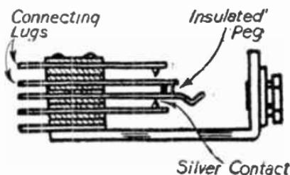
FIG. 388.—Contact points of a Jack.
