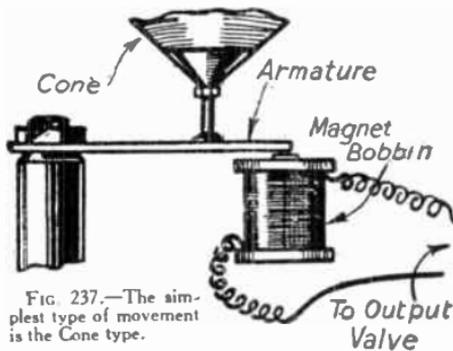
FIG. 237.—The simplest type of movement is the Cone type.
