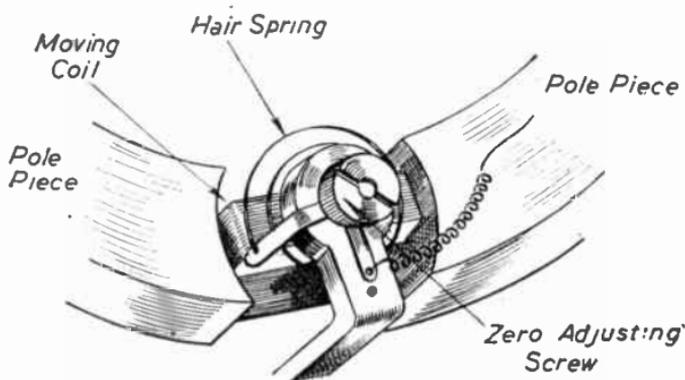
FIG. 269.—Perspective view of the active elements of a moving-coil instrument.
