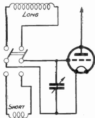
FIG. 440.—A simple method of fitting a Switch for wave-changing.
