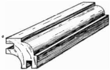
FIG. 79.—The shape and grooves of the corner moulding are clearly seen here.
