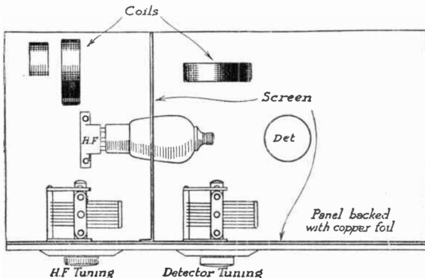
FIG. 226.—A Screen the same depth as the Baseboard is used for "partitioning off" the H.F. stage.
