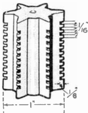
FIG. 215.—Method of cutting ebonite former for the H.F. Choke.
