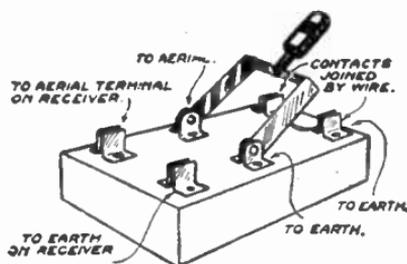
FIG. 35.—The method of connecting up the Lightning Switch.
