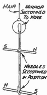
FIG. 204.—Details of the Hair, Magnetic Needles, and Mirror.
