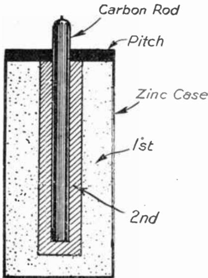
FIG. 470.—Section of a Dry Cell.
