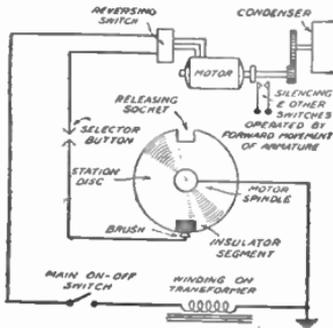
FIG. 349c.—Some forms of automatic tuners are motor driven, the basic principle being as shown here.
