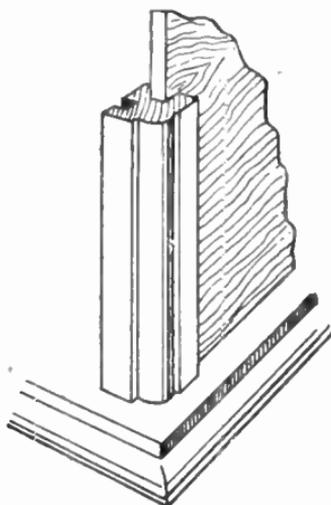
FIG. 77.—This shows plainly how corner moulding simplifies the construction.
