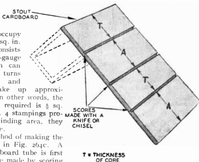
Fig. 264c.—Method of marking out and folding the Winding Spool.
