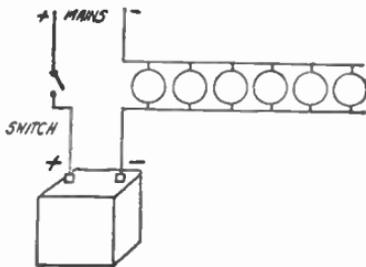
FIG. 20a.—A typical arrangement of Lamp Resistances.
