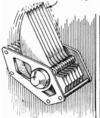
FIG. 293.—Vibrating condenser vanes may cause a microphonic howl.
