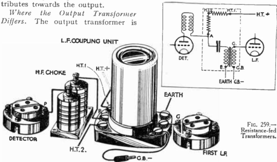
FIG. 259.—Resistance-fed Transformers.
