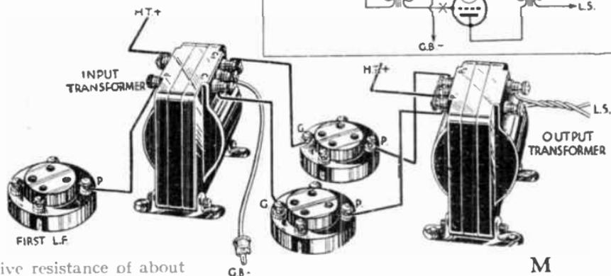
FIG. 260.—Push-pull system of L.F. Coupling.
