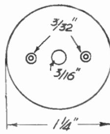
Fig. 314.—Bearing Discs for the pick-up.
