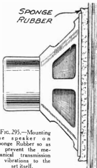
FIG. 295.—Mounting the speaker on Sponge Rubber so as to prevent the mechanical transmission of vibrations to the set itself.
