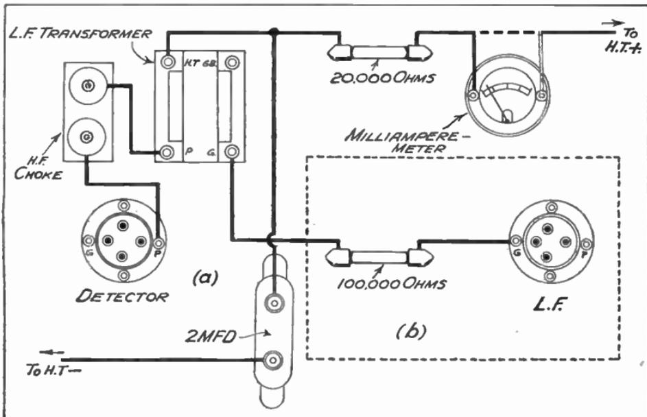
FIG. 189.—A decoupling resistance in the anode lead, and a resistance in the grid lead to cure instability.
