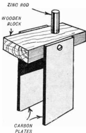
FIG. 227A.—The Carbon Plates for a Leclanché Cell.
