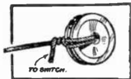
FIG. 33.—The wire passed through the insulator to form a double bight.
