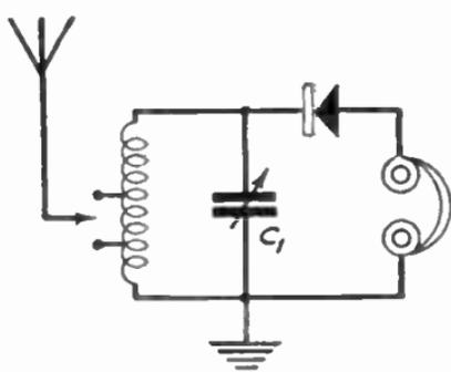
FIG. 97.—The very simplest Crystal Circuit.
