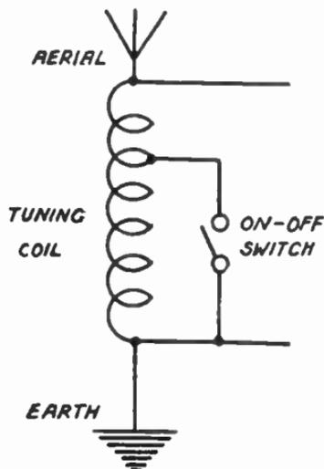
FIG. 377.—On-off Switch used for wave changing.
