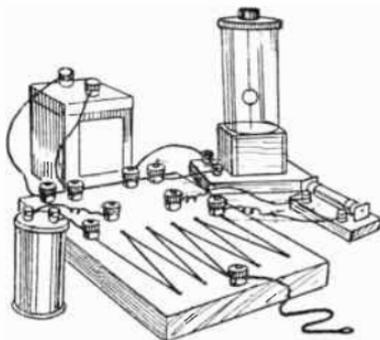
FIG. 482.—The Wheatstone Bridge and its associated apparatus.
