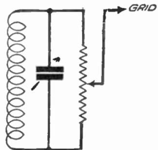
FIG. 478.—A Potentiometer across the Grid Coil.
