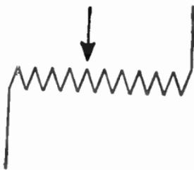
FIG. 348.—A Potentiometer shown theoretically
