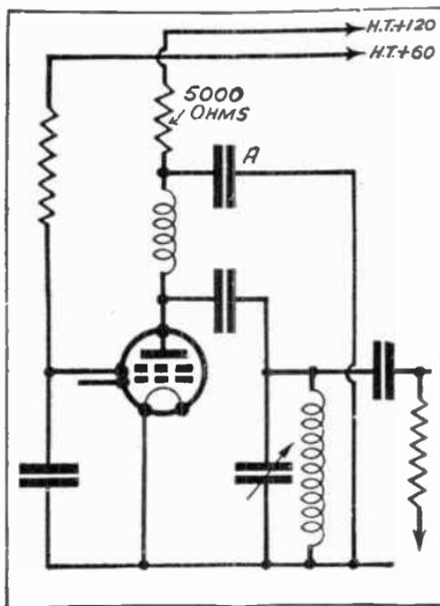
FIG. 166.—S.G. stage decoupled.
