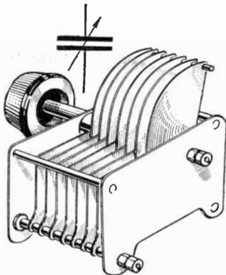
FIG. 50.—Variable condenser with air dielectric.
