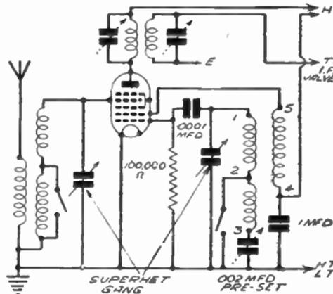
FIG. 149.—Here is the circuit of the frequency changer stage of a superhet employing an I.F. of 110 kc/s.
