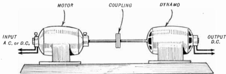
FIG. 7.—Diagram showing the principle of the Rotary Converter and Rotary Transformer. A motor, either A.C. or D.C., is driven from the mains and coupled to a D.C. generator which charges the accumulators. In practice one machine acts both as motor and dynamo.
