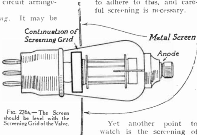
FIG. 226A.—The Screen should be level with the Screening Grid of the Valve.
