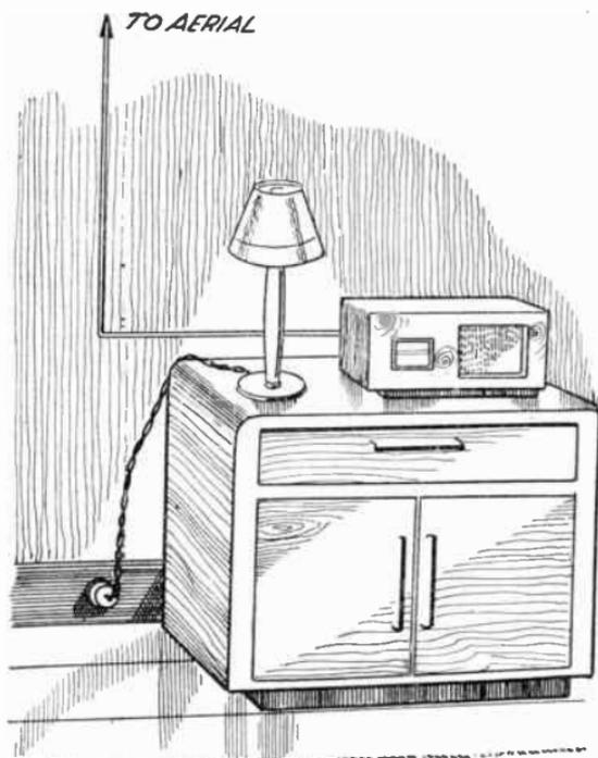
FIG. 289.—One cause of Hum is the Aerial, Earth or Speaker Leads running parallel to the Supply Mains.
