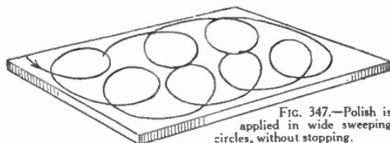
FIG. 347.—Polish is applied in wide sweeping circles, without stopping.
