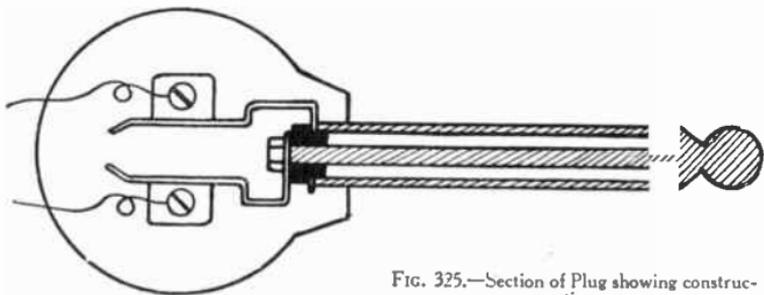
FIG. 325.—Section of Plug showing construction.
