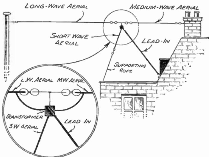
FIG. 48.—All-wave anti-interference aerial.
