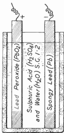
FIG. 19.—State of cell when charged.
