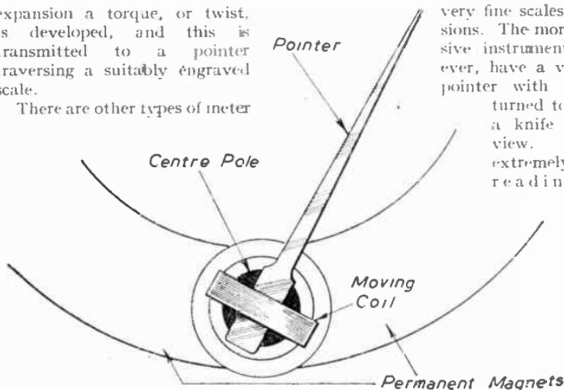
FIG. 267.—A Moving-coil Instrument with the hair spring and bearings, etc., removed to show assembly details.
