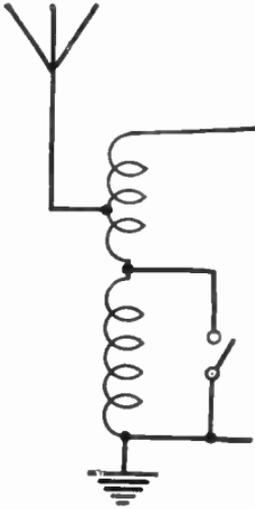
FIG. 70.—A very common circuit employed in commercial coils. Break through does not occur, but it is unselective on the long waves.
