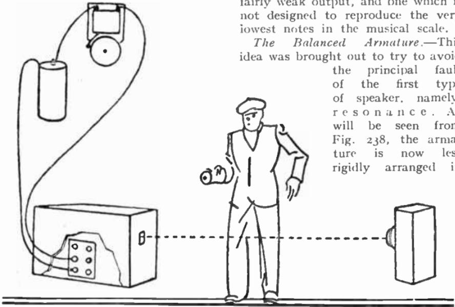
FIG. 235.—The connections for the invisible-ray burglar alarm.
