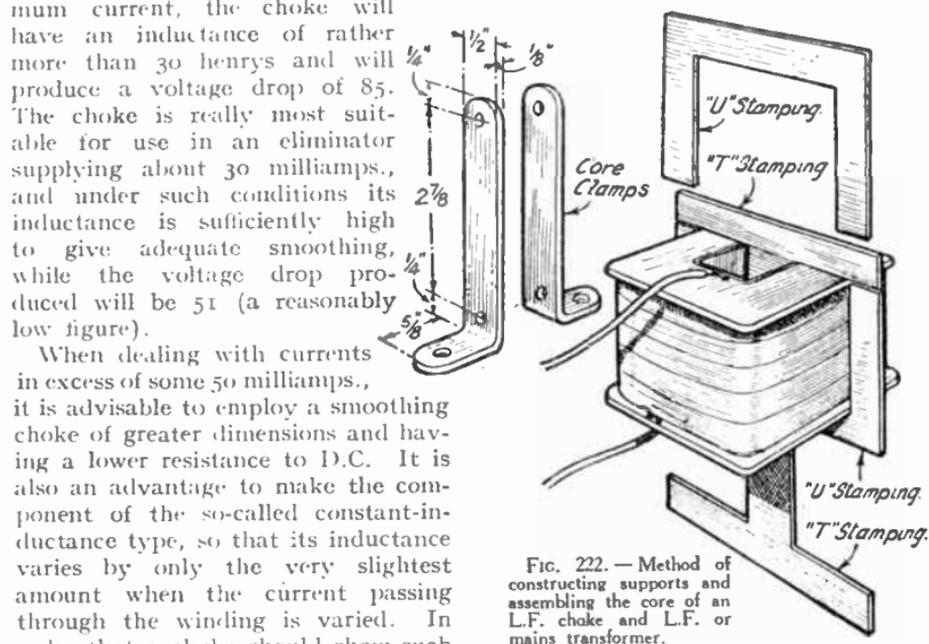
FIG. 222.—Method of constructing supports and assembling the core of an L.F. choke and L.F. or mains transformer.
