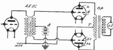
FIG. 349d.—Diagram explaining the Push-pull Circuit.
