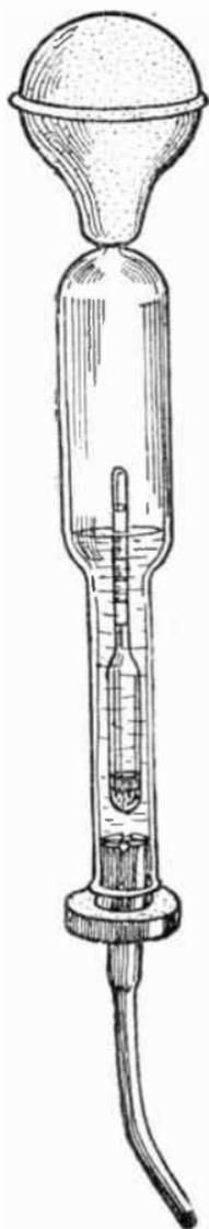
FIG 54.—Another type of Hydrometer.
