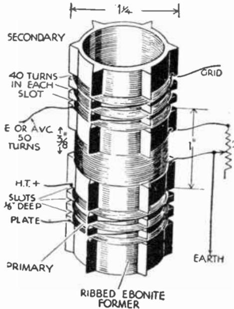
FIG. 146.—A third winding is used in this I.F. Transformer to control the degree of selectivity.
