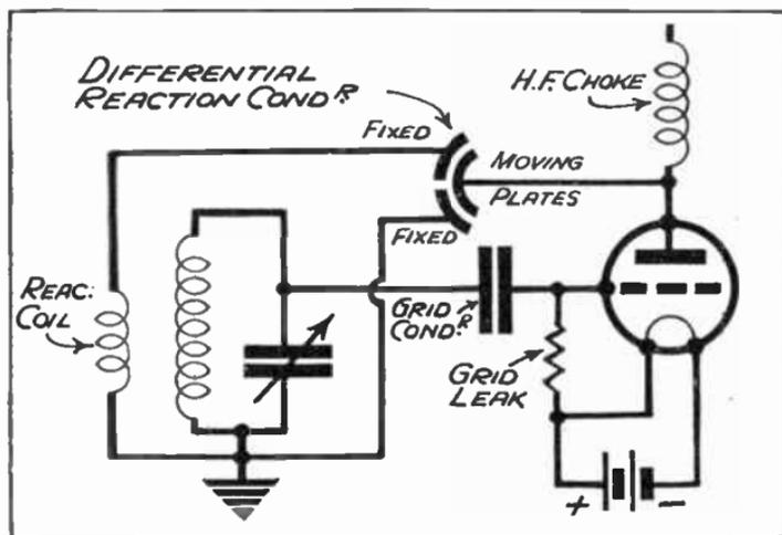
FIG. 171.—The method of connecting a differential condenser when the reaction coil is joined to the earth line. The connections to the reaction coil govern the differential condenser connections.
