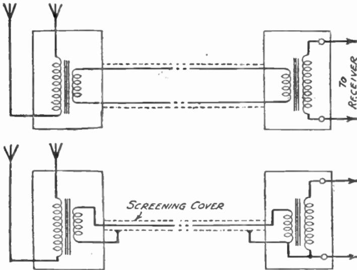
FIG. 49.—Connections for two types of impedance-matching transformer for anti-interference aerials.
