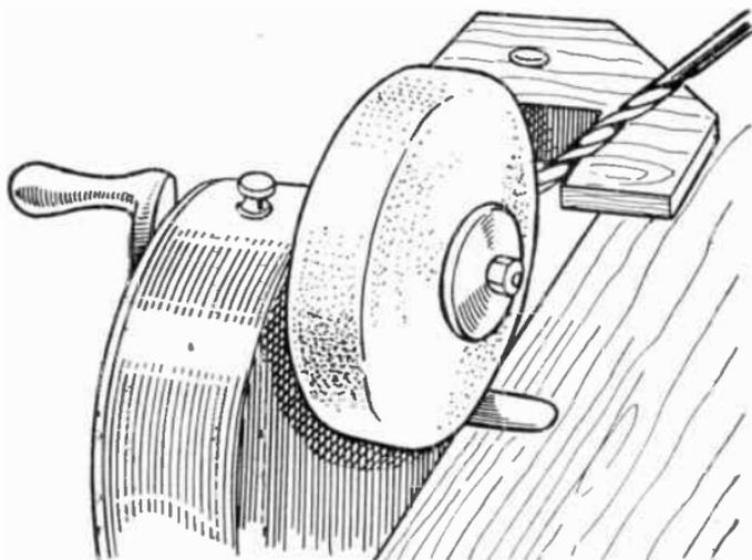
FIG. 177.—The correct angle at which to hold the Drill—and a Drill Rest.
