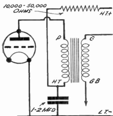
FIG. 296.—How to fit a decoupling resistance and condenser to stop motor-boating.
