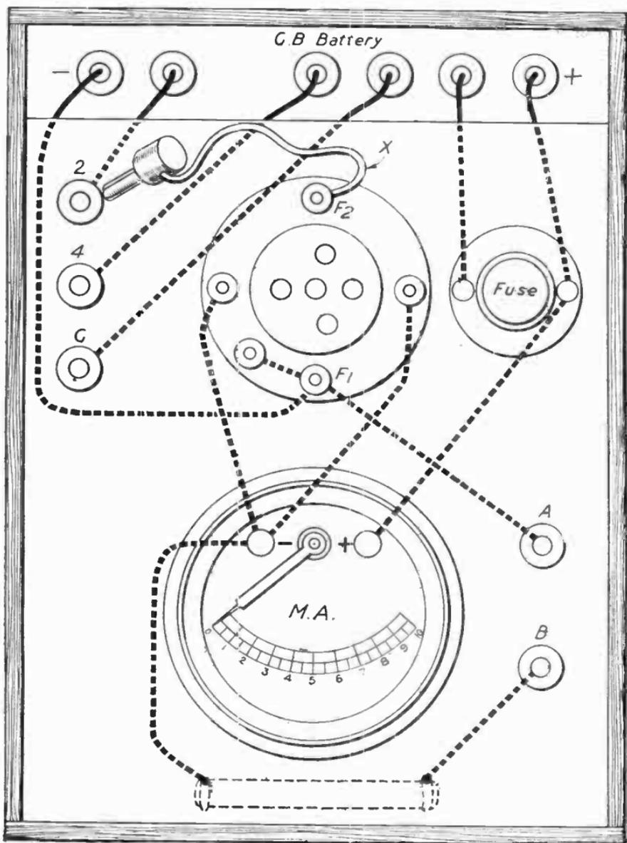
FIG. 468.—Wiring diagram of the Valve Tester.
