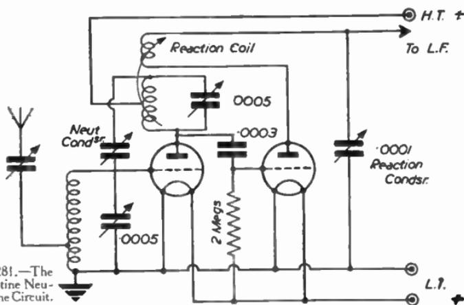
FIG. 281.—The Hazeltine Neutrodyne Circuit.
