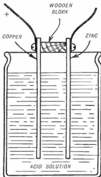
FIG. 227b.—A Voltaic Cell.
