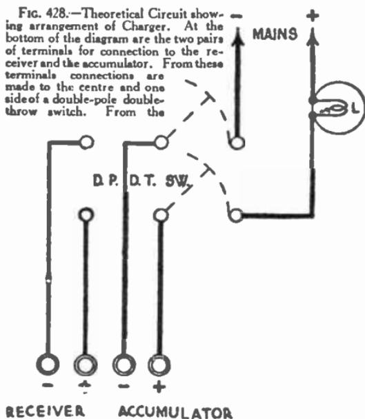
FIG. 428.—Theoretical Circuit showing arrangement of Charger. At the bottom of the diagram are the two pairs of terminals for connection to the receiver and the accumulator. From these terminals connections are made to the centre and one side of a double-pole double-throw switch. From the other side of the switch connection is made with the mains plug by means of a flex lead, in the positive leg of which the lamp L is inserted.
