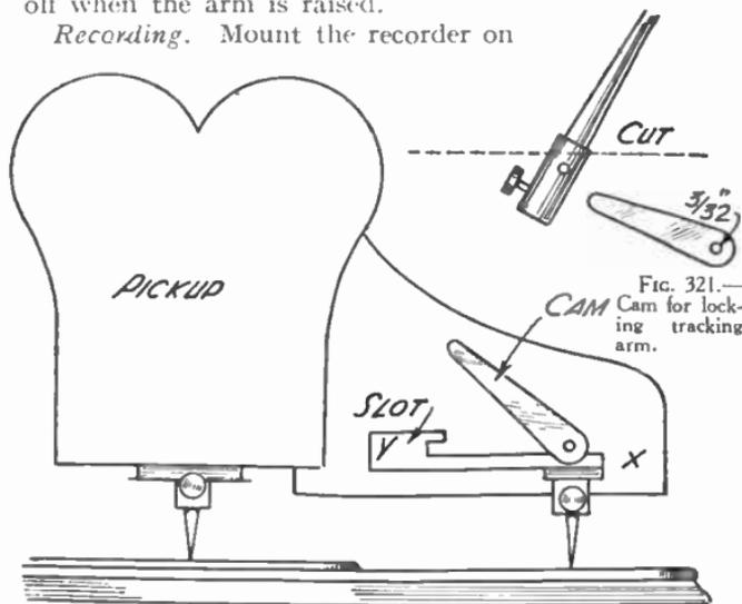
FIG. 320.—Diagram showing relative positions of Cutting and Tracking Needles.
