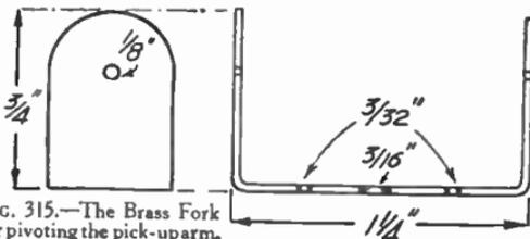
FIG. 315.—The Brass Fork for pivoting the pick-up arm.
