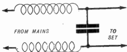
FIG. 285.—A Cure for H.F. Interference via the Mains.
