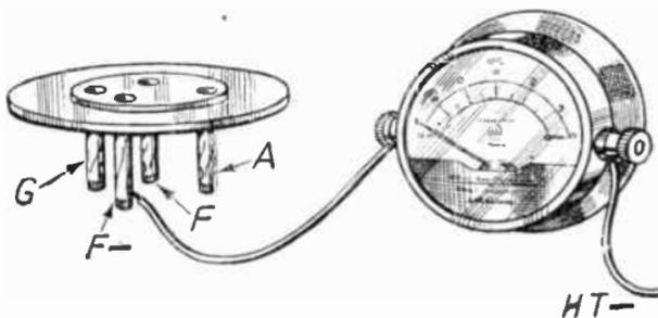
FIG. 272.—Reading the Anode Consumption of the Set in Milliamps.
