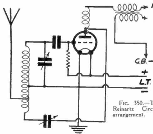
FIG. 350.—The Reinartz Circuit arrangement.
