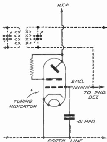
FIG. 469.—Connections for cathode-ray tuning indicator.
