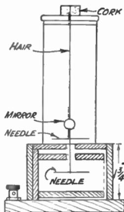
FIG. 201.—A sectional view of the completed instrument.
