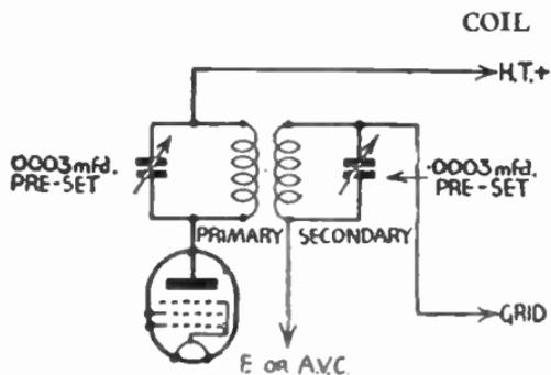
FIG. 142.—In this HF. Transformer coupling between the two windings is carried out inductively.
