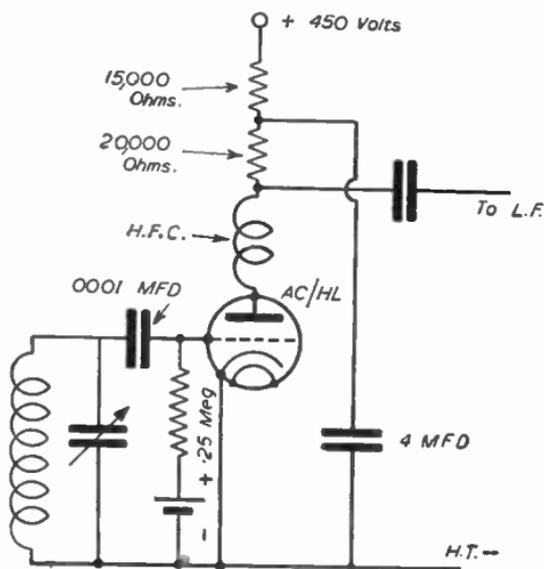
FIG. 358.—The Resistance necessary in a Power Grid Rectifier which is also decoupled.
