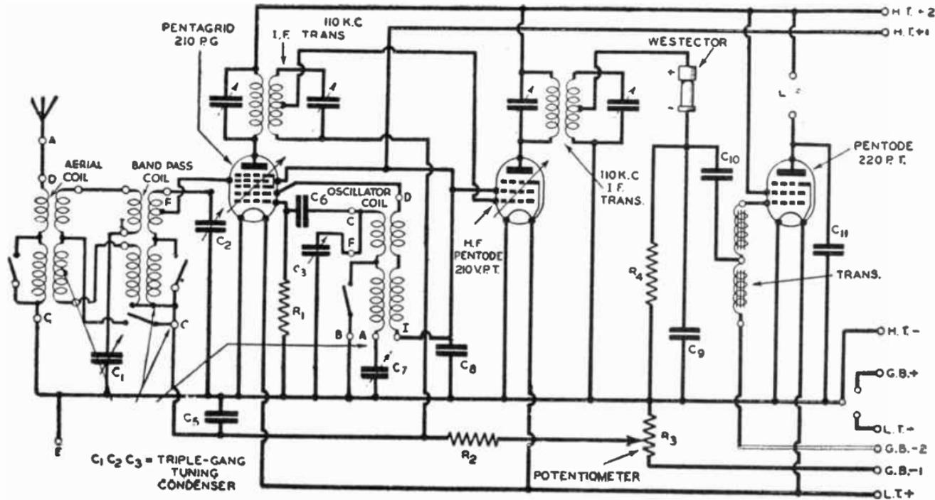
FIG. 108.—Circuit No. 11 : A Three-valve Battery-operated Superhet.
