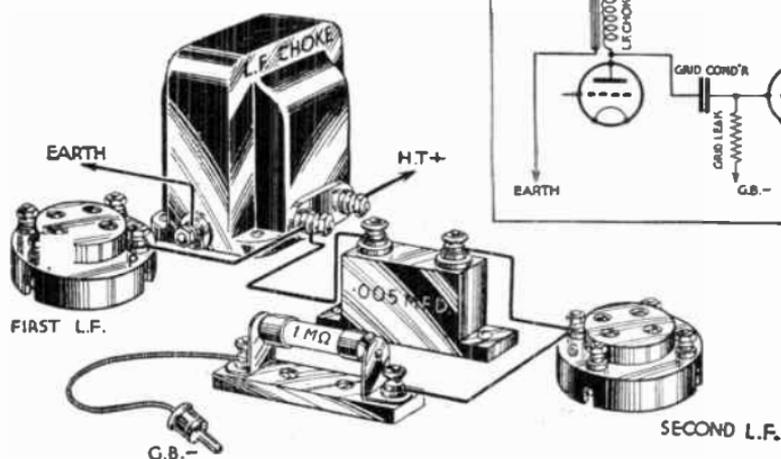
FIG. 257.—Choke-capacity Coupling.
