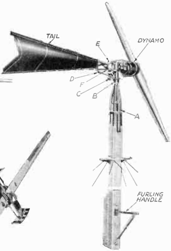
FIG. 11.—A Commercial Wind-Charger, with furling tail.
