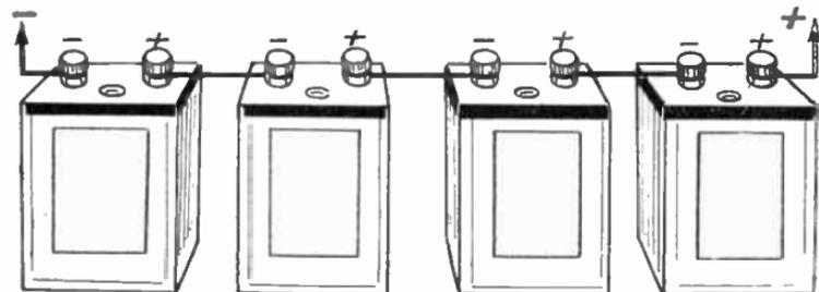
FIG. 4.—Accumulators connected in Series.
