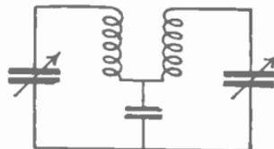
FIG. 175c.—Capacity-coupled Circuit.
