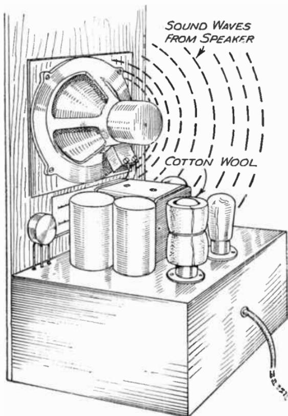
FIG. 292.—A jacket of cotton-wool round the detector valve, so as to prevent sound waves from the speaker impinging on it, will often stop a microphonic howl.
