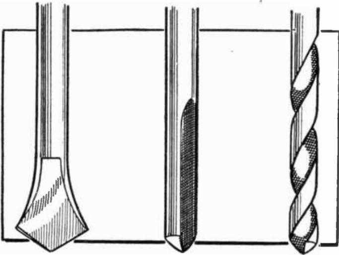
FIG. 180.—Three types of Drill—the Diamond, Straight Flute, and Twist.
