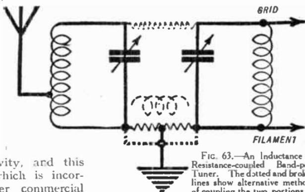
FIG. 63.—An Inductance or Resistance-coupled Band-pass Tuner. The dotted and broken lines show alternative methods of coupling the two portions of a Band-pass Tuner.
