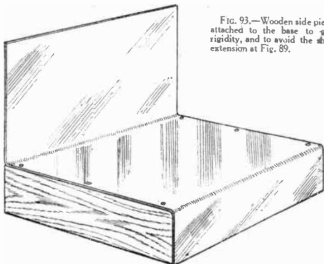
FIG. 93.—Wooden side pieces attached to the base to give rigidity, and to avoid the short extension at Fig. 89.
