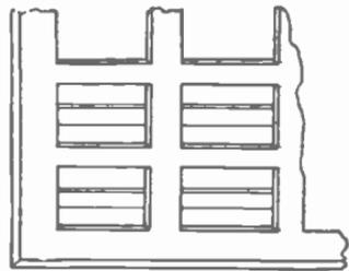
FIG. 31.—The Grid ready for pasting.
