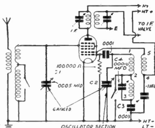
FIG. 147.—Theoretical circuit of the frequency-changing stage of a superhet receiver.
