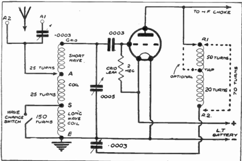
FIG. 140.—A circuit diagram showing the Coil fitted in the set.
