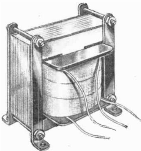
FIG. 265B.—One method of finishing off. Flexible leading-out wires are used.
