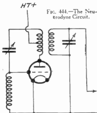
FIG. 444.—The Neutrodyne Circuit.
