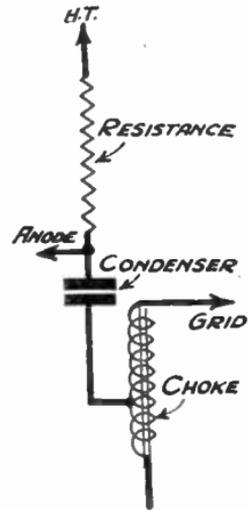
FIG. 254.—The Resistance-fed Auto-transformer arrangement.
