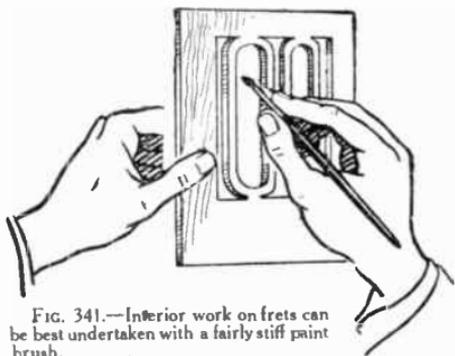
FIG. 341.—Interior work on frets can be best undertaken with a fairly stiff paint brush.
