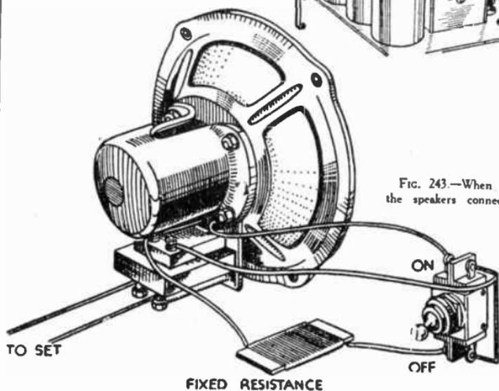
FIG. 243.—When switching out one of the speakers connected in parallel it is sometimes an advantage to leave the primary winding of the output transformer in circuit. In that case it is well to replace the speech coil by a fixed resistance of similar value.
