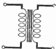
FIG. 226c.—Theoretical diagram of an L.F. Transformer.
