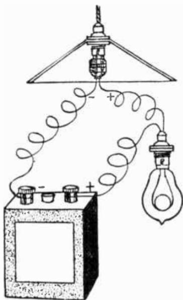
FIG. 20B.—Simple Charging Arrangement from D.C. Mains.
