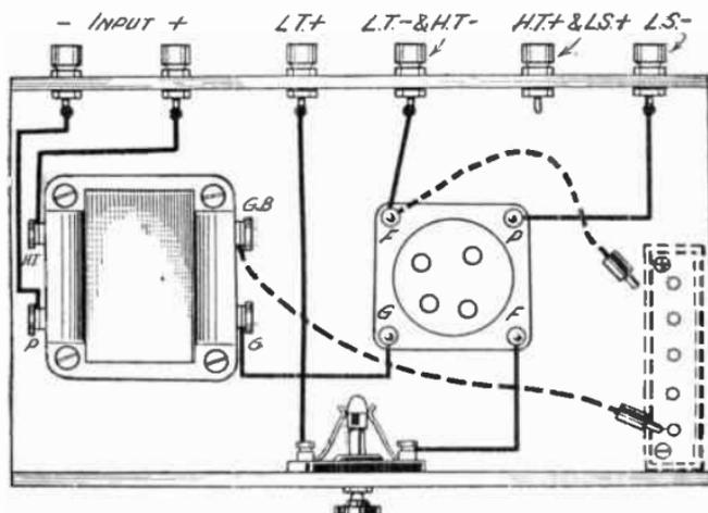
FIG. 121.—A One-valve Amplifier.
