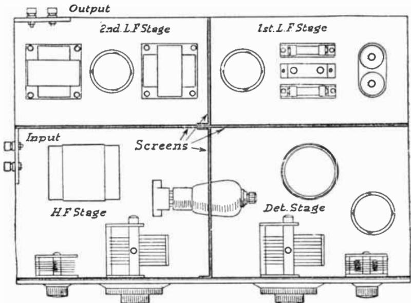
FIG. 226B.—When the Input and Output ends of the receiver come close together the set should be screened as shown.
