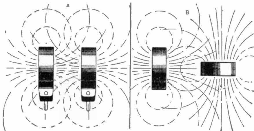
FIG. 225.—Showing the shape of the electro-magnetic field of coils of the usual plug-in type.
