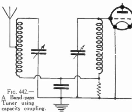
FIG. 442.—A Band-pass Tuner using capacity coupling.
