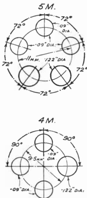
FIGS. 461 and 462.—The two diagrams above show the valve-leg spacing of the Hivac midjet valves (see table on page 369).
