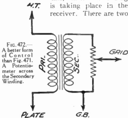
FIG. 472.—A better form of Control than Fig. 471. A Potentiometer across the Secondary Winding.
