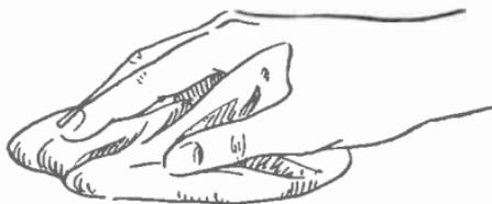
FIG. 345.—How to hold the polishing rubber.
