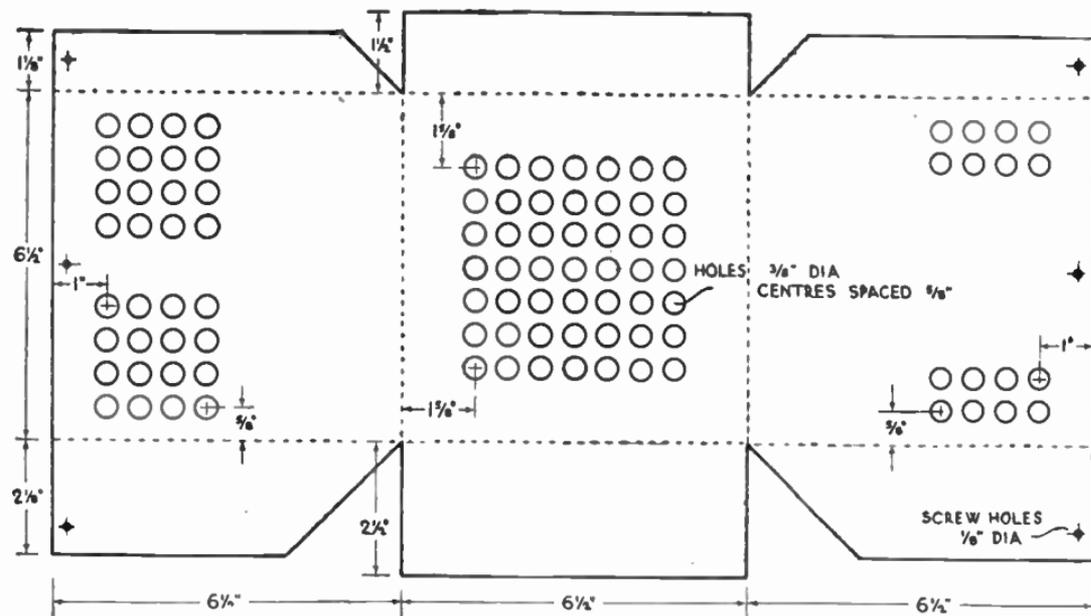
FIG. 433.—The Sheet-metal Cover. Cut out and drill as shown then bend along the dotted lines.
