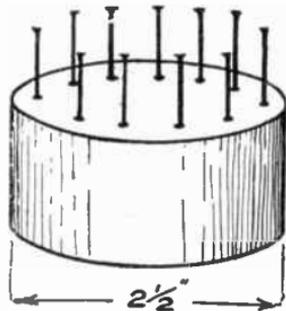
FIG. 123.—The wooden block and nails for making a Basket-weave Coil.
