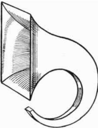
FIG. 248.—A method of curving which avoids bends.
