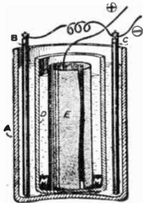
FIG. 65.—Section of the Bichromate Cell. A, glass jar; B and C, carbon rods; D, porous pot; E, zinc; M, mercury.
