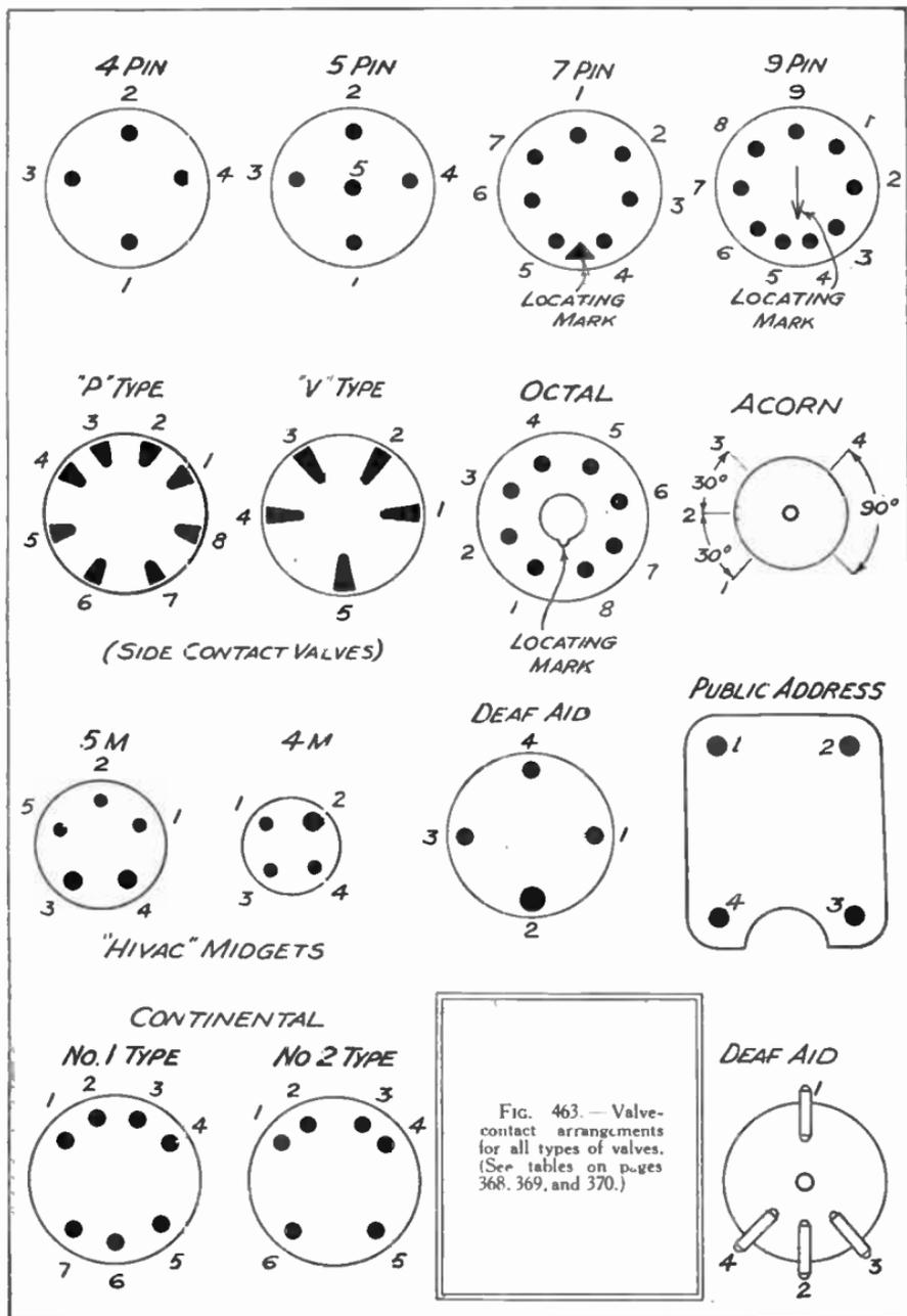
FIG. 463.— Valve-contact arrangements for all types of valves. (See tables on pages 368, 369, and 370.)
