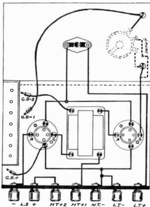
FIG. 209.—Wiring diagram of Gramophone Amplifier shown in Fig. 207.
