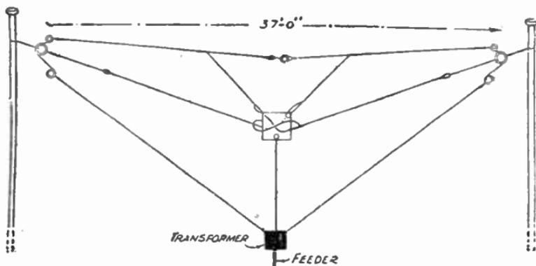
FIG. 47.—The Spider-web anti-interference aerial.
