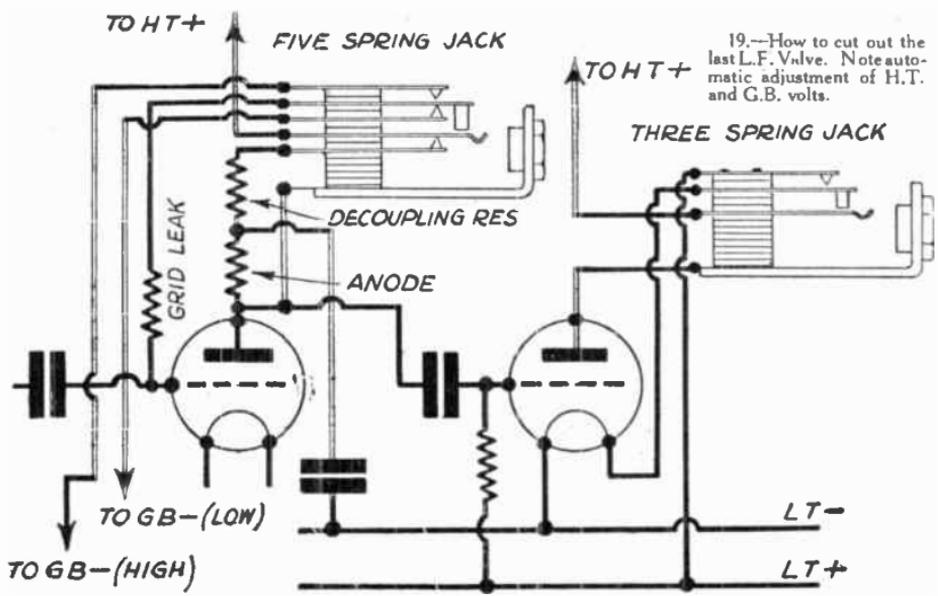
19.—How to cut out the last L.F. Valve. Note automatic adjustment of H.T. and G.B. volts.
