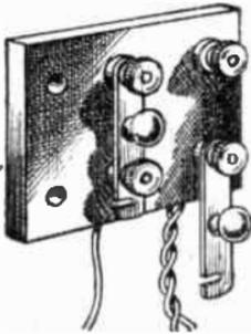
FIG. 42.—The Switch in earthed position.
