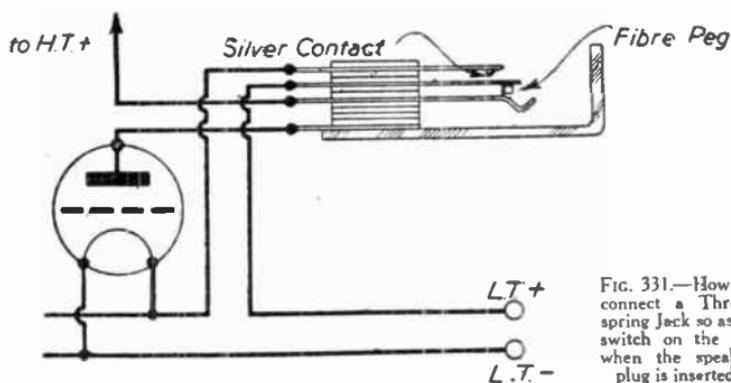
FIG. 331.—How to connect a Three-spring Jack so as to switch on the set when the speaker plug is inserted.
