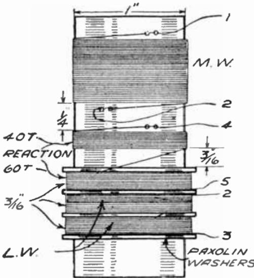
FIG. 148.—Constructional details of an efficient oscillator coil.
