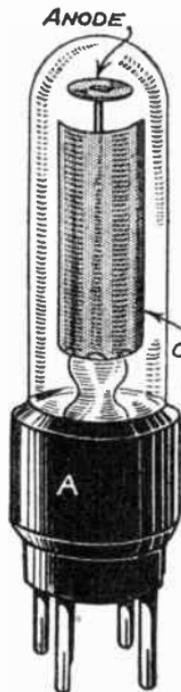
FIG. 308.—The Photo-electric Cell, showing the shape of the Electrodes.
