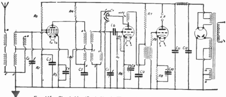
FIG. 115.—Circuit No. 17: A Simple Three-valve A.C. mains receiver.
