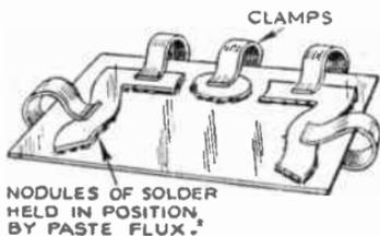
FIG. 367.—Strips held in position by spring Clamps.
