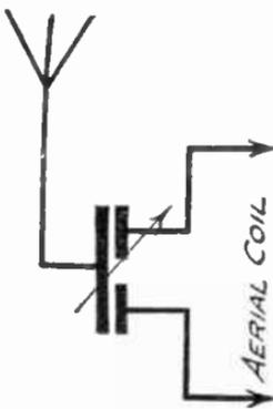
FIG. 475.—A Differential Condenser in the Aerial Circuit.
