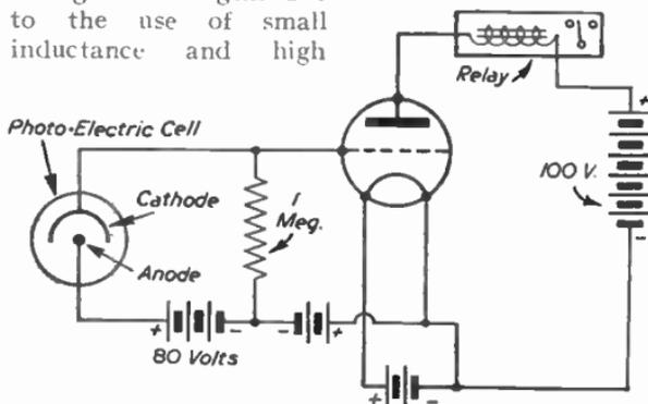
FIG. 307.—The standard method of connecting the Photo-electric Cell.
