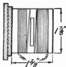
FIG. 203.—The Former for winding the Coil.
