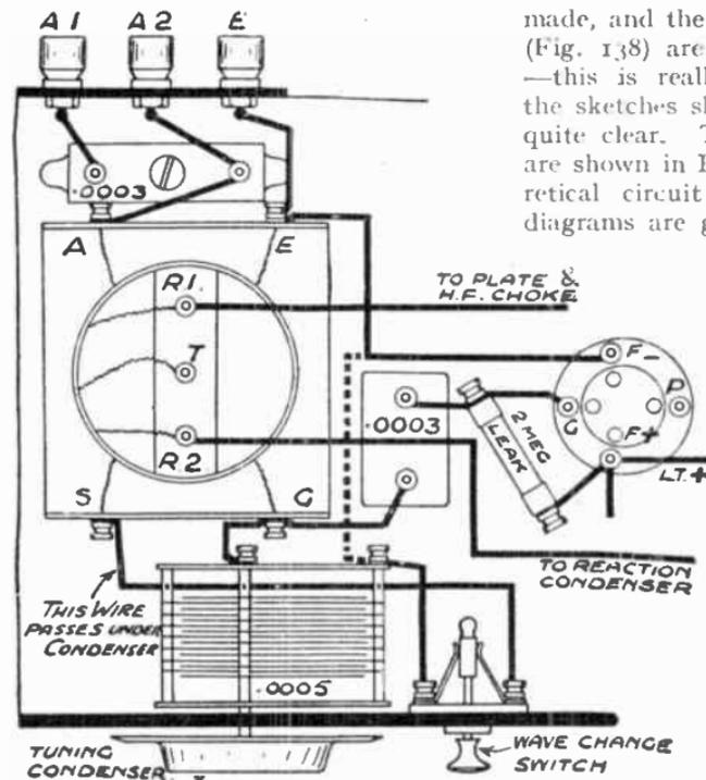
FIG. 141.—How the Coil is fitted in the set.
