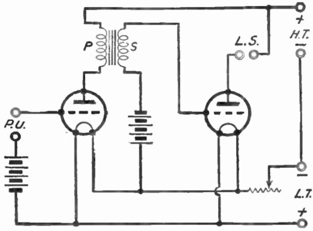
FIG. 205.—Circuit Diagram for a Two-Valve Gramophone Amplifier
