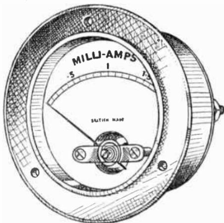
FIG. 280.—A panel-mounting Milliammeter.
