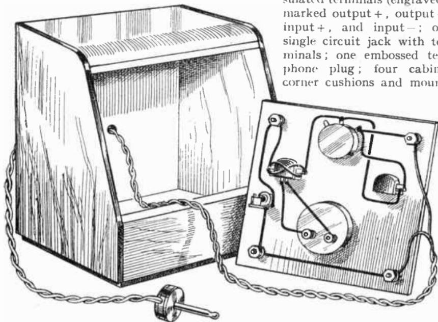
FIG. 278.—A view of the Tester with the front Panel removed to show the Wiring.
