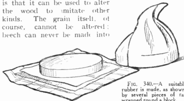
FIG. 340.—A suitable rubber is made, as shown, by several pieces of rag wrapped round a block.
