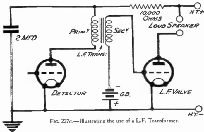
FIG. 227C.—Illustrating the use of a L.F. Transformer.
