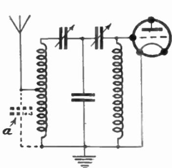
FIG. 438.—The Circuit arrangement of the Band-pass Scheme.
