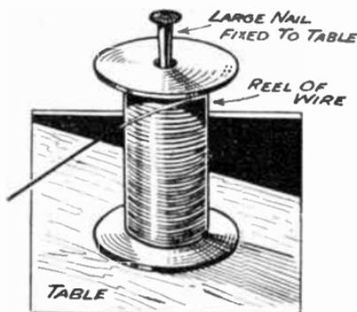
FIG. 131.—A nail driven in the bench to hold the reel while the wire is wound on the coil.
