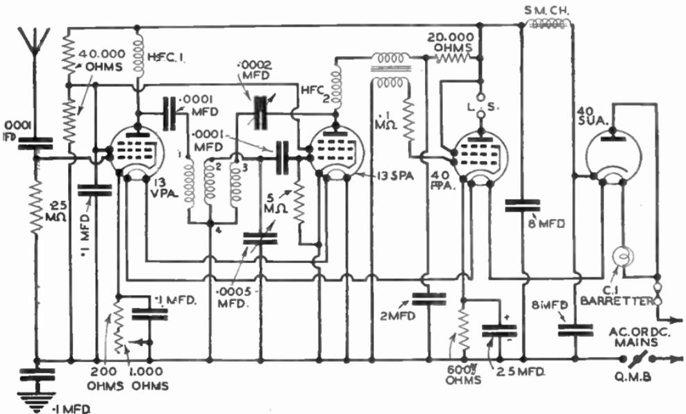
FIG. 116.—Circuit No. 18: A Universal (A.C./D.C.) Mains Three-valver.
