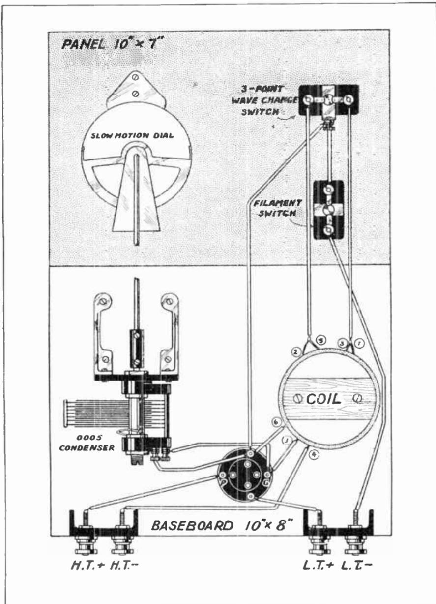
FIG. 481.—Wiring diagram for the Heterodyne Wavemeter.
