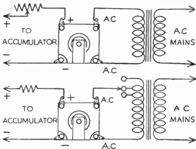
FIG. 16.—Two standard methods of employing a metal rectifier for charging accumulators.
