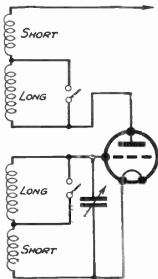
FIG. 445.—A Single-pole Single-throw Switch for wave-changing.
