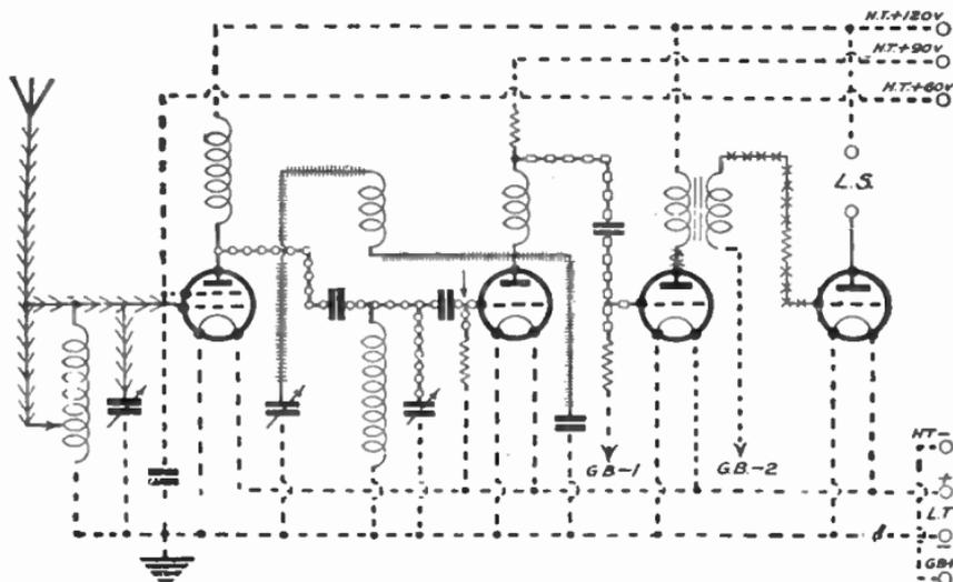
FIG. 226E.—A Circuit with the various Circuits indicated by different types of lines.
