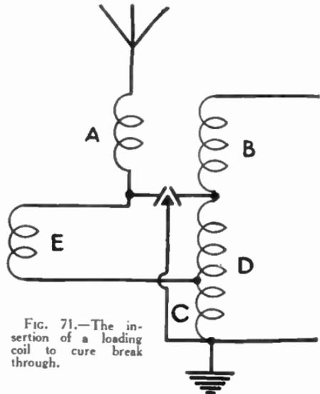
FIG. 71.—The insertion of a loading coil to cure break through.
