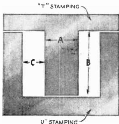
FIG. 264B.—Illustration of the Transformer Stampings to be used in conjunction with the table on p. 238.
