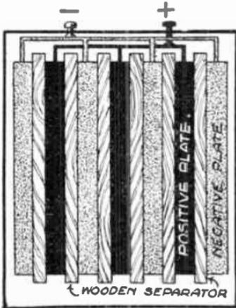
FIG. 28.—Section of a Heavy-duty type of Accumulator
