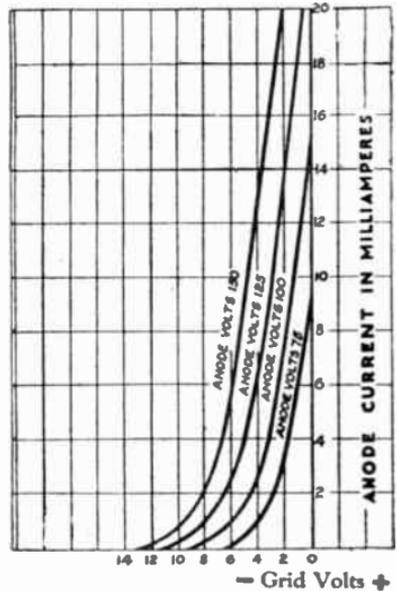
FIG. 467.—A Steep Slope Valve Curve.
