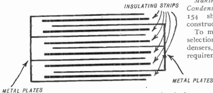
FIG. 154.—The plates in a condenser, shown on an enlarged scale.
