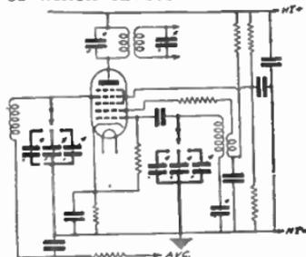
FIG. 349B.—In a modern superhet two tuned circuits may be automatically switched by using two or more presets on the lines shown in Fig. 349A.
