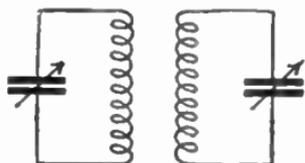
FIG. 175A.—Inductively coupled coils.
