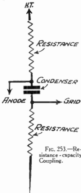
FIG. 253.—Resistance-capacity Coupling.
