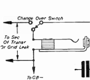
17.—A useful Pick-up Circuit using a Panel Switch in conjunction with the Plug and Jack.
