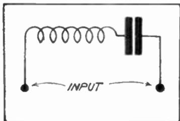
FIG. 2.—Acceptor Circuit.
