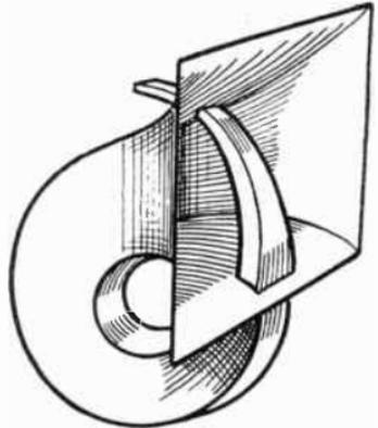
FIG. 249.—How the very large Cinema Horns are formed.
