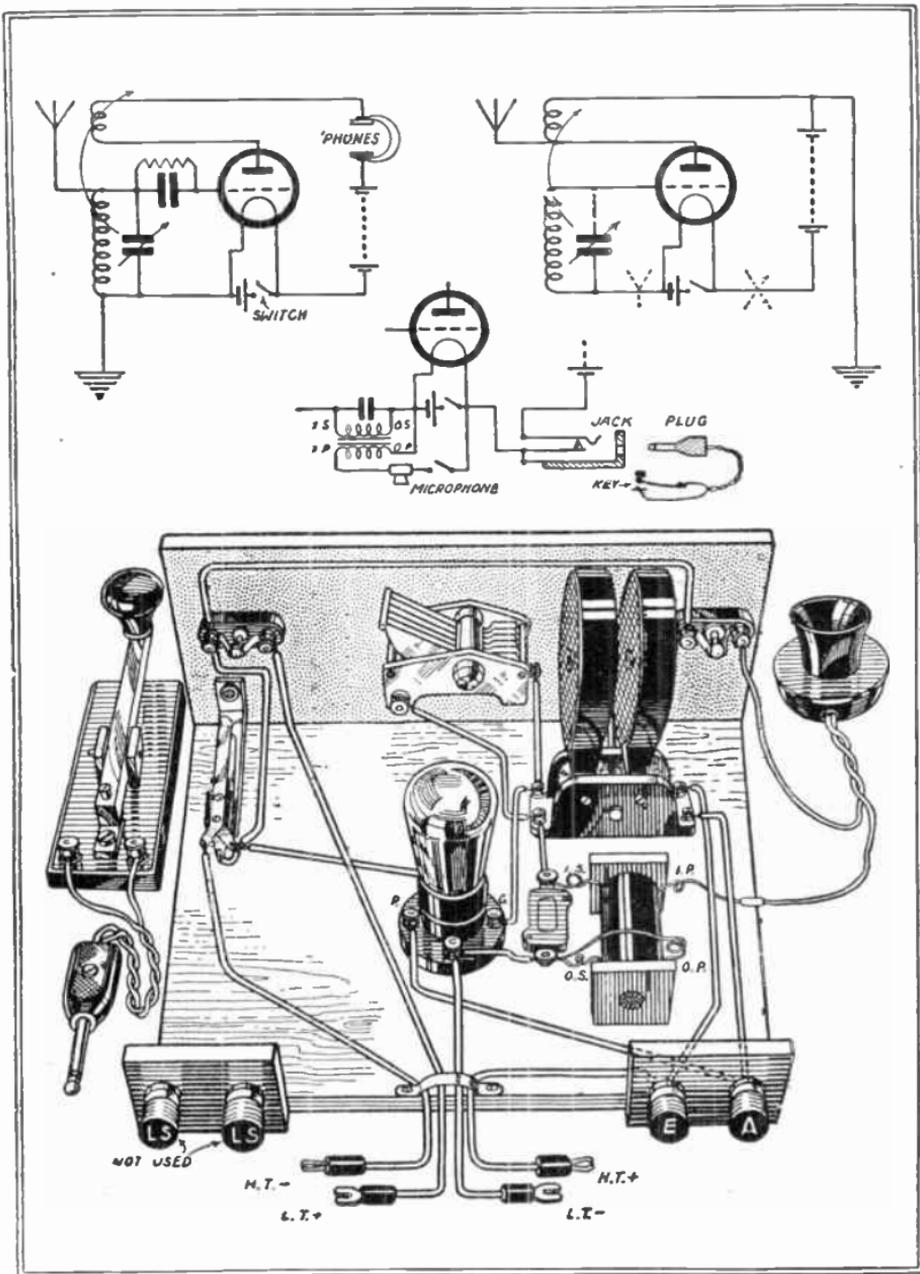
FIGS. 426 and 427.—A 1-Valve Transmitter, with circuit showing how it differs from a 1-Valve Receiver.
