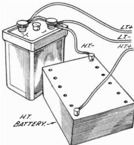
FIG. 230.—The Battery Connections.
