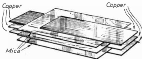
FIG. 155.—Pictorial diagram of the Copper and Mica Layers.
