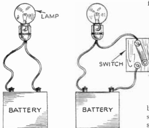
FIG. 390.—How the on-off Switch functions.
