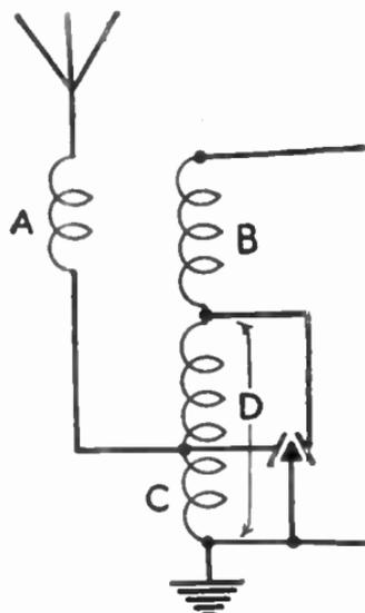
FIG. 69.—Another typical Dual-range Circuit.
