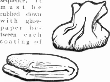
FIG. 339.—The pad below is of wadding or similar absorbent substance—to be used as a polisher. It is wrapped in linen to the shape shown by the upper drawing.
