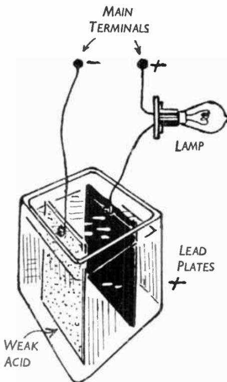
FIG. 27.—Method of testing Mains for Polarity.
