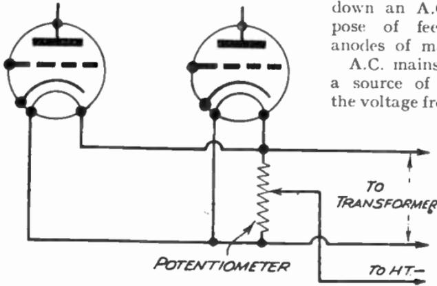
FIG. 264.—A cure for Mains Hum—a Potentiometer is connected across the Heater Supply Wiring.
