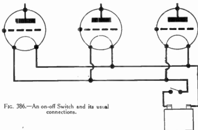
FIG. 386.—An on-off Switch and its usual connections.
