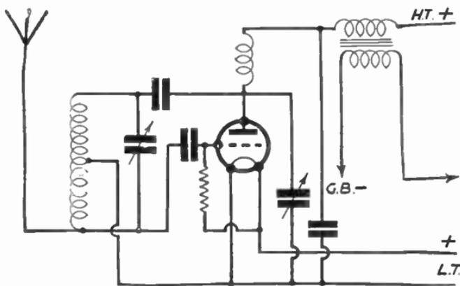
FIG. 213.—The Hartley Circuit.
