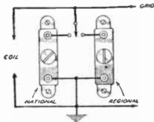
FIG. 349A.—Selecting preset condensers, by means of a change-over switch, for automatic tuning.
