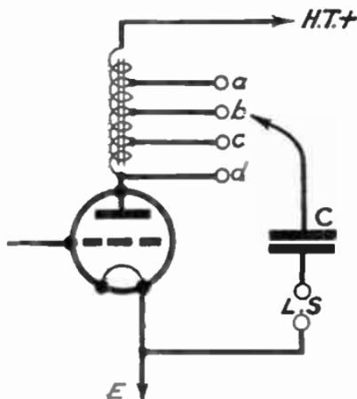
FIG. 306.—Choke-capacity Output.
