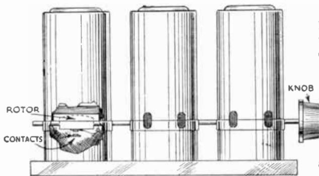
FIG. 389.—Three-gang Tuning Coil with self-contained Switch.
