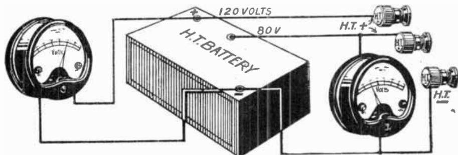
FIG. 270.—Voltmeters for checking different values of high tension.
