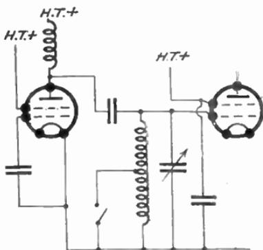
FIG. 451.—The Tuned Grid system.
