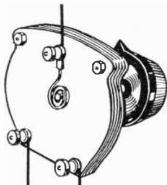
FIG. 170.—A Differential Condenser of the solid Dielectric type.
