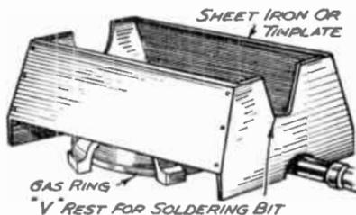
FIG. 371.—An easily-made Cowl that can be fitted over the gas ring.
