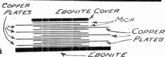
FIG. 160.—Diagram of the complete assembly.
