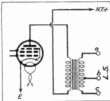
FIG. 305.—Transformer Output.
