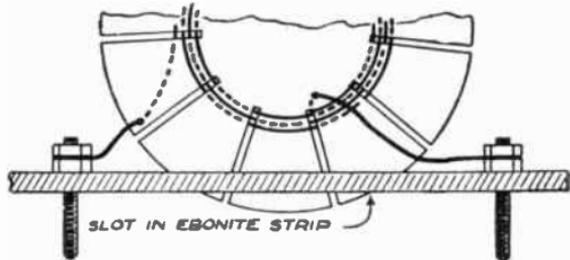
FIG. 127.—How the Coil is mounted.
