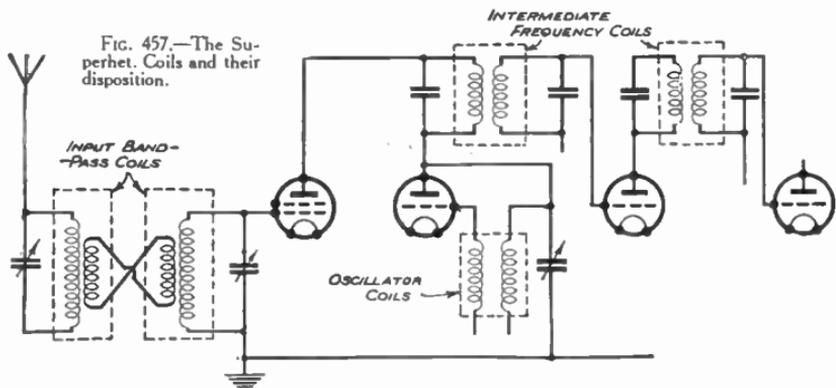
FIG. 457.—The Superhet. Coils and their disposition.
