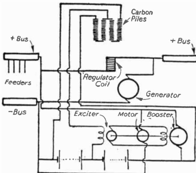
FIG. 67.—Arrangement of Automatic Reversible Booster.
