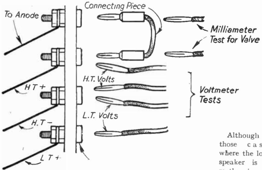
FIG. 273.—Fitting Sockets on the Panel enabling the milliameter and voltmeter tests to be made from the exterior of the set.
