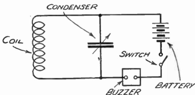
FIG. 479.—A Buzzer Wavemeter.
