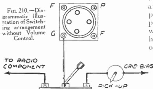
FIG. 210.—Diagrammatic illustration of Switching arrangement without Volume Control.
