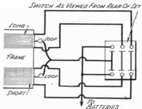
FIG. 111.—The Switch Connection to the Aerial of Circuit No. 13.
