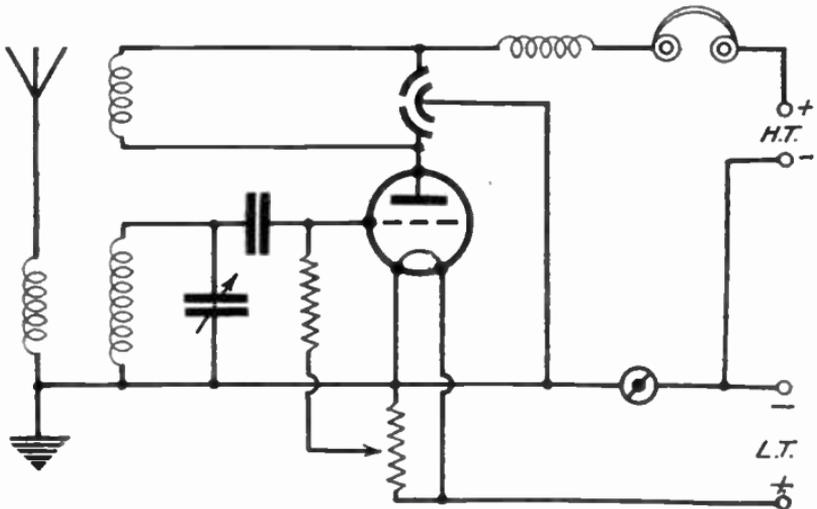
FIG. 99.—Circuit No. 2: a similar circuit to Fig. 98, employing a different system of reaction control.
