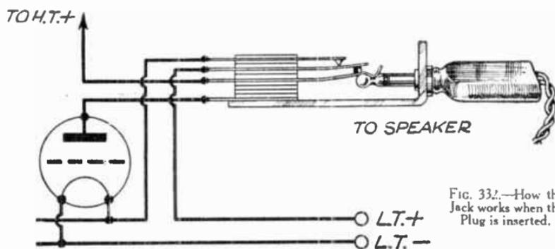
FIG. 332.—How the Jack works when the Plug is inserted.
