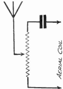
FIG. 477.—A Resistance instead of a differential Condenser in the Aerial Circuit.
