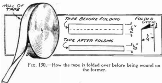
FIG. 130.—How the tape is folded over before being wound on the former.
