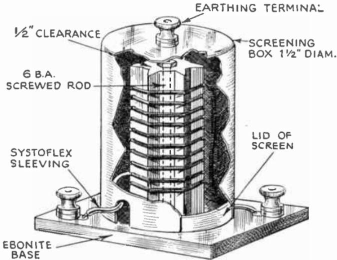
FIG. 217.—Complete assembling details of a screened H.F. Choke.
