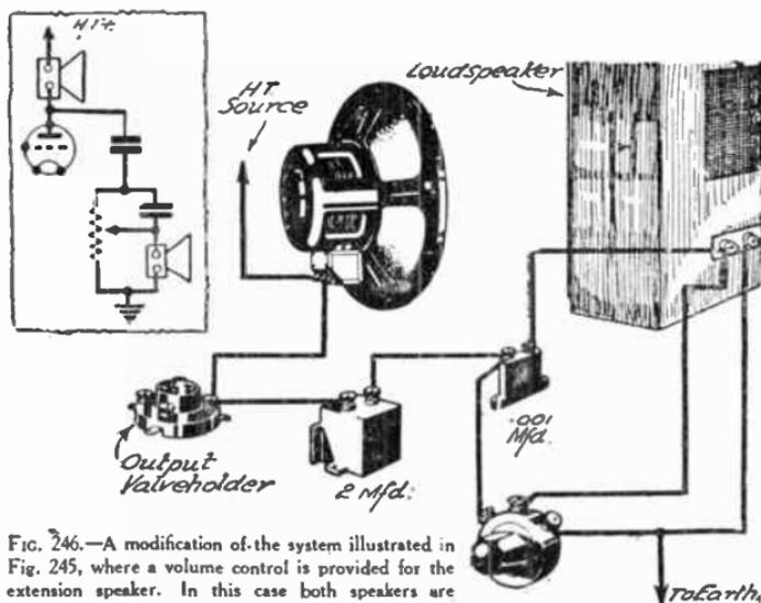
FIG. 246.—A modification of the system illustrated in Fig. 245, where a volume control is provided for the extension speaker. In this case both speakers are always kept in circuit.
