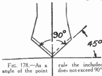
FIG. 178.—As a rule the included angle does not exceed  $90^\circ$ .
