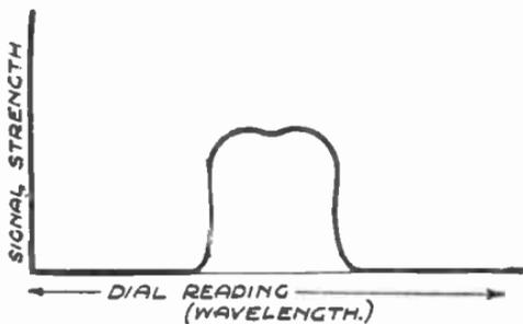
FIG. 449.—Band-pass Wave Form..
