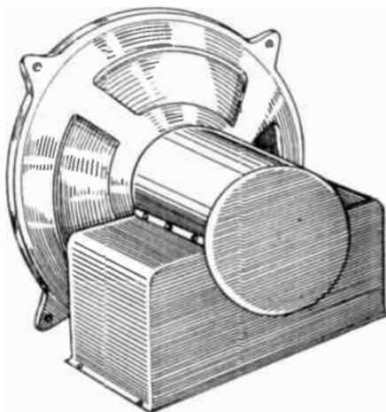
FIG. 241.—A mains energised Moving-coil Loudspeaker.
