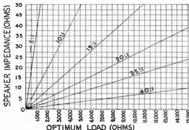
FIG. 303.—Graph for Moving-coil Speaker.
