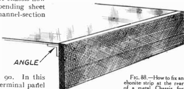
FIG. 88.—How to fix an ebonite strip at the rear of a metal Chassis for terminal connections.
