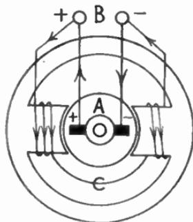
FIG. 14.—A shunt-wound 2-pole dynamo.
