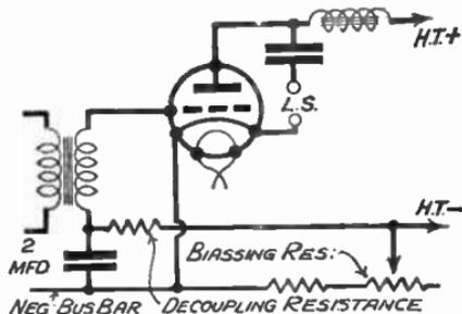
FIG. 58.—An alternative arrangement of Fig. 57, in which the cathode is maintained at the normal negative potential.
