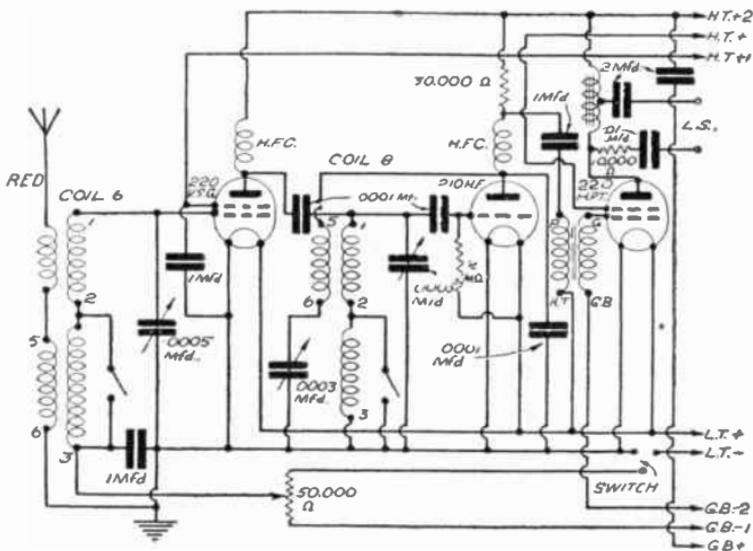
FIG. 113.—Circuit No. 15: A Three-valve Set with Variable-mu Volume Control.
