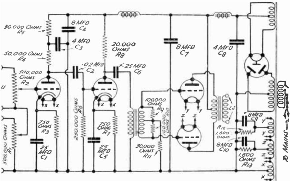
FIG. 120.—Circuit No. 22: A 12-watt Amplifier.
