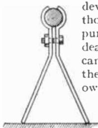
FIG. 365.—How to make a permanent fixing for the foot of the stand.
