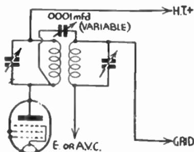
FIG. 144.—In this arrangement a small variable condenser provides the coupling and thus the selectivity may be varied.
