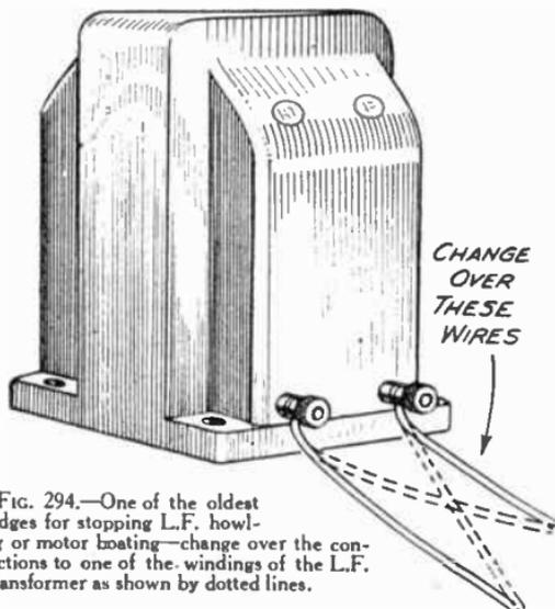
FIG. 294.—One of the oldest dodges for stopping L.F. howling or motor boating—change over the connections to one of the windings of the L.F. Transformer as shown by dotted lines.
