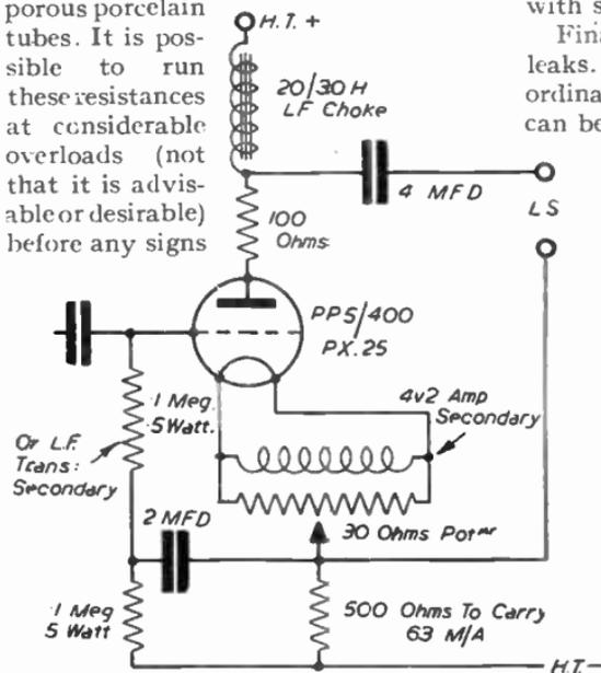
FIG. 359.—An Output Valve which is Mains Operated, and the Power Rating of all Resistances which are included in the Circuit.
