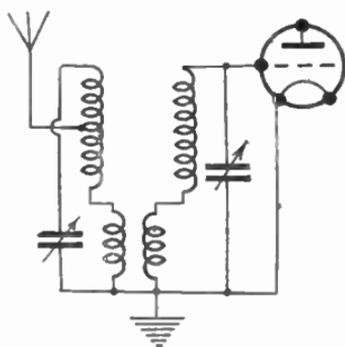
FIG. 454.—A Band-pass Tuner with common Coupling Coil.
