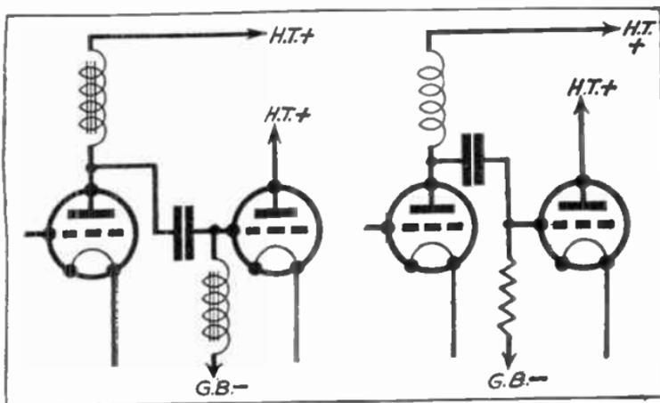
FIG. 164.—Two forms of Choke Coupling.
