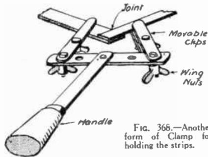
FIG. 368.—Another form of Clamp for holding the strips.
