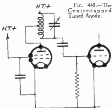
FIG. 448.—The Centre-tapped Tuned Anode.
