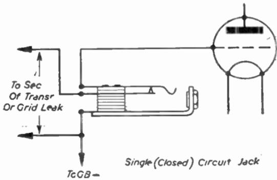
15.—A Jack arranged for plugging in Pick-up to one of the L.F. stages.
