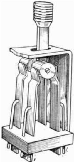
FIG. 380.—Anti-capacity Switch.
