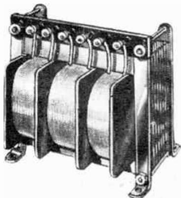
FIG. 265c.—In this method the windings are brought out to a terminal strip.
