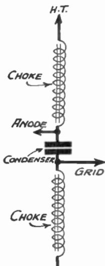
FIG. 255.—Choke Impedance Coupling.
