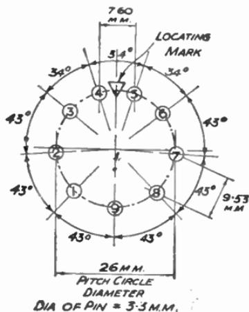
FIG. 460.—Valve-leg spacing for 9-pin valves.
