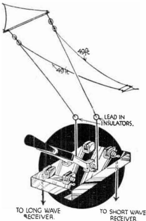
FIG. 198A.—A duplex aerial arrangement for long and short waves.
