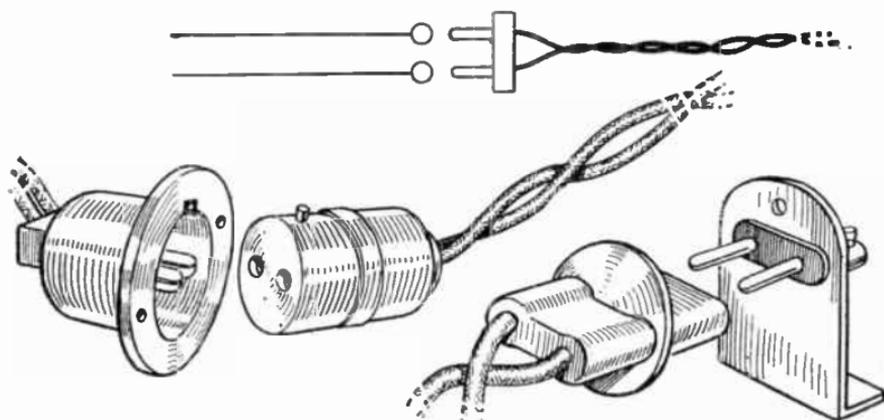
FIG. 375.—Theoretical and actual diagrams of a plug-in Connector.
