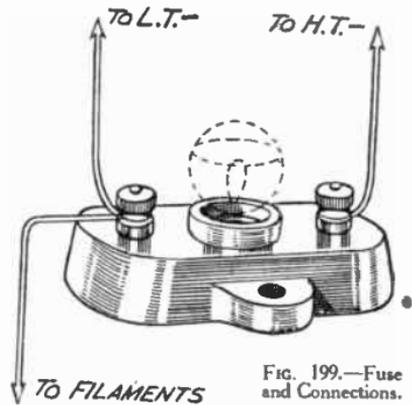
FIG. 199.—Fuse and Connections.
