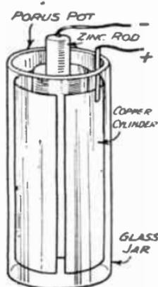
FIG. 165.—Constructional details of Daniell Cell.
