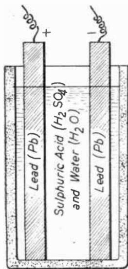
FIG. 18.—Simple cell ready for charging.
