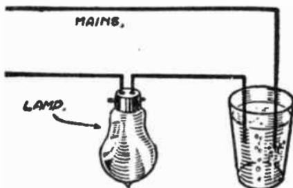
FIG. 17.—Dissolve a teaspoonful of salt in a glass of water and dip the ends of the charging wires in the solution. Bubbles of gas will form on the negative wire. (See also Figs. 26 and 27.) Take care that the two wires do not touch one another.
