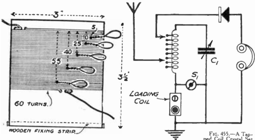
FIG. 455.—A Tapped Coil Crystal Set showing (left) details of the coil winding with 26 gauge D.C.C. wire.
