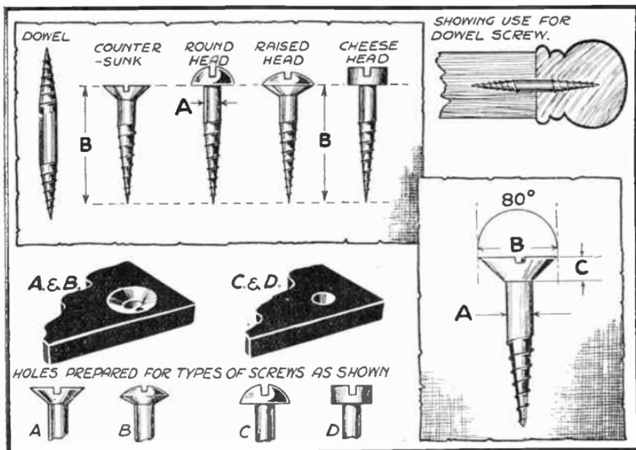
FIG. 484.—Wood Screw proportions and types.
