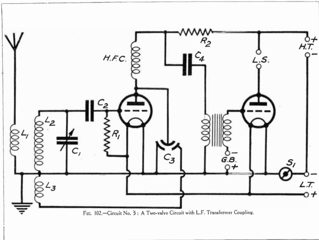
FIG. 102.—Circuit No. 5: A Two-valve Circuit with L.F. Transformer Coupling.
