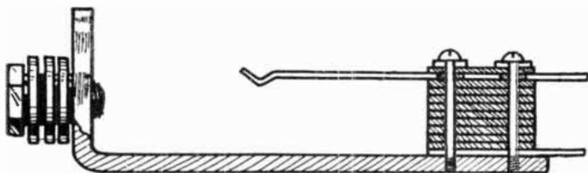
FIG. 326.—Details of Single-circuit Jack.
