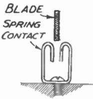
FIG. 381.—Double-pole Knife Switch.
