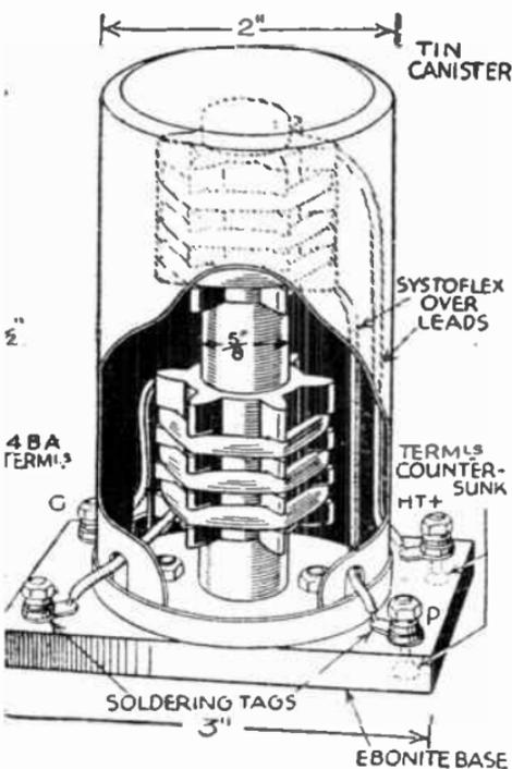
FIG. 143.—A simple form of I.F. Transformer in which variable coupling can be introduced.
