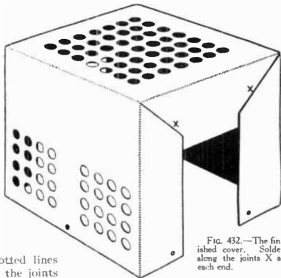
FIG. 432.—The finished cover. Solder along the joints X at each end.
