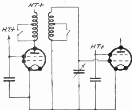
FIG. 453.—A H.F. Transformer with wave-switching.
