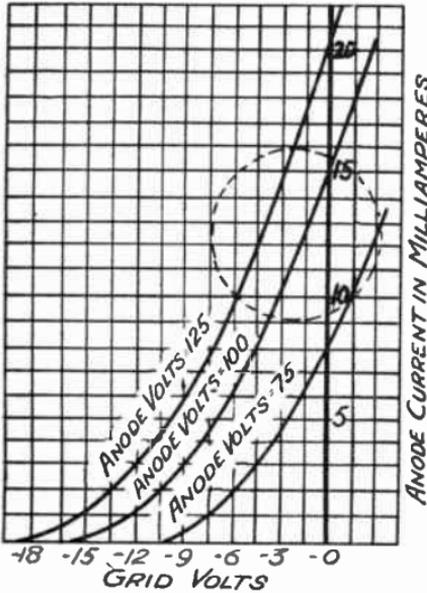
FIG. 80.—The ordinary grid-volts anode current curves.
