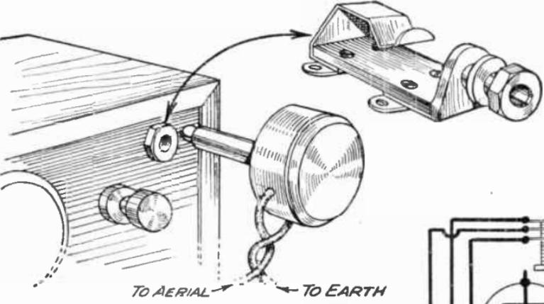
21.—A portable set may be quickly attached to an outside aerial by using a Plug and Jack. Inset: details of the Jack.
