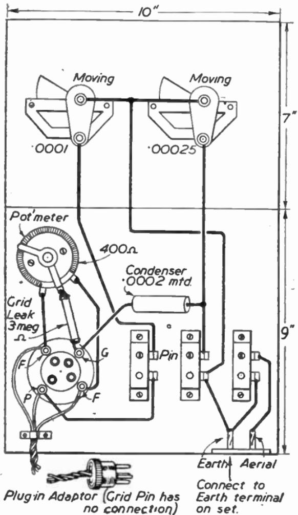
FIG. 104.—Circuit No. 7: Wiring Diagram for Short-wave Adapter Unit.
