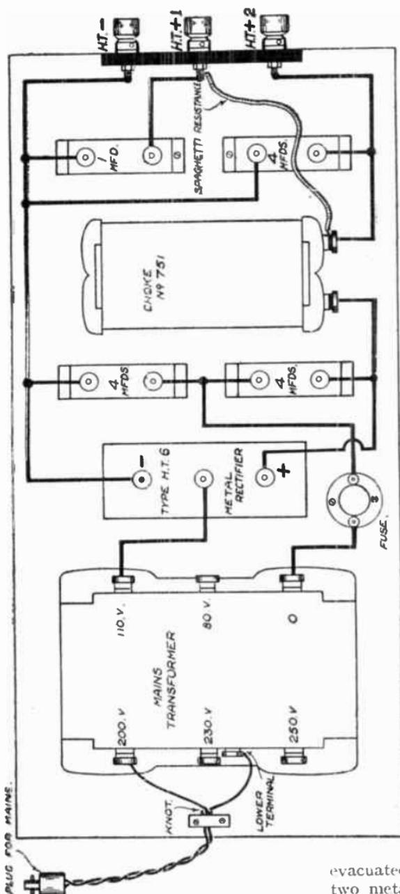
FIG. 183.—The Wiring Diagram of the A.C. Mains Unit.
