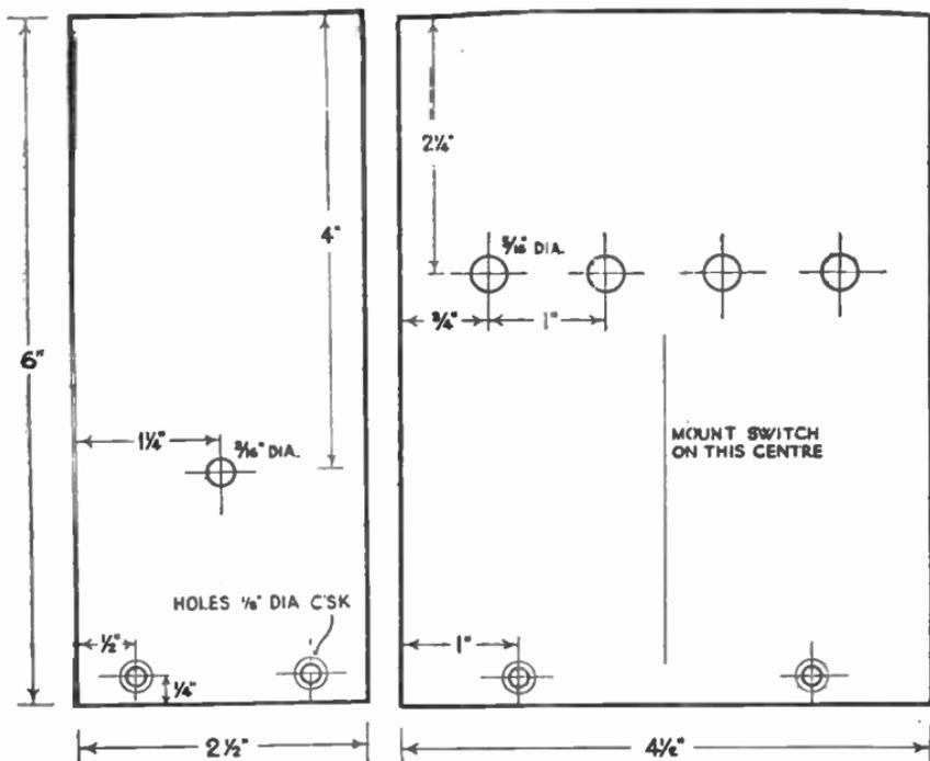
FIG. 431.—The two small Ebonite Panels. Cut from a 7 × 6-in. panel and drill as shown, the four holes in the larger piece being of suitable size for large insulated terminals. In addition the necessary mounting holes for the switch must be made on the centre line shown on the panel.
