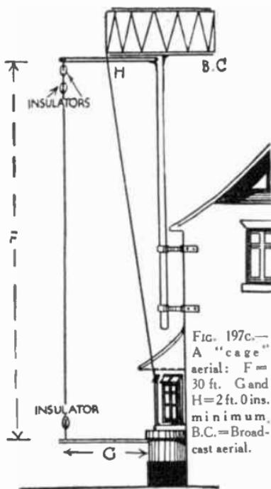
FIG. 197C.—A "cage" aerial: F=30 ft. G and H=2 ft. 0 ins. minimum. B.C.=Broadcast aerial.
