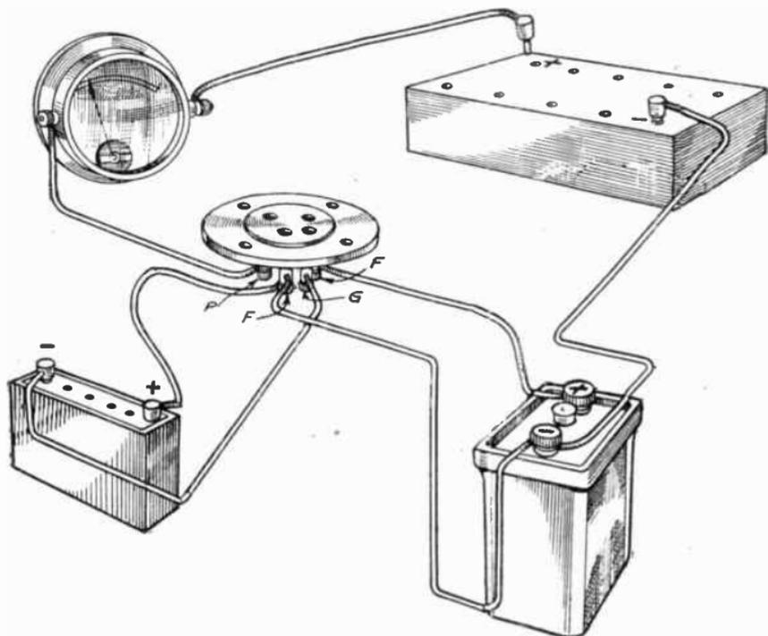
FIG. 82.—How to arrange the necessary parts in order to read a valve and prepare your own curves, or check your valves.
