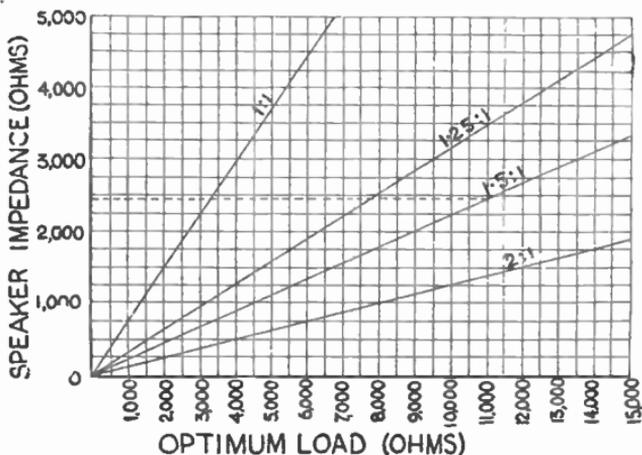
FIG. 304.—Graph for Moving-iron Speaker.
