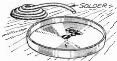
FIG. 370.—Coil of solder with a tin lid underneath to catch the drips of solder.
