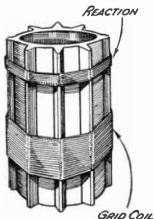
FIG. 122.—Theoretical and actual diagrams of an Aerial Tuning Coil.
