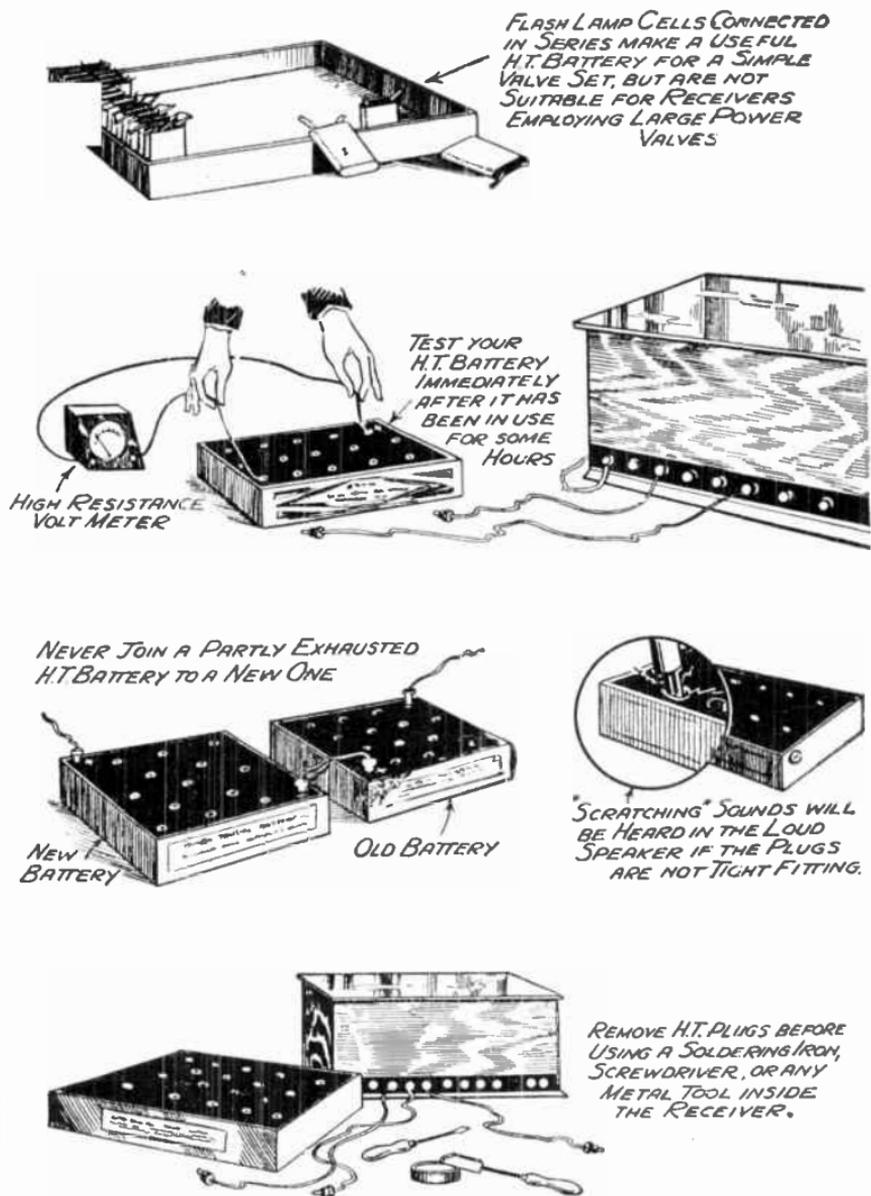
FIG. 224.—The battery user should carefully study the various points shown in this diagram.
