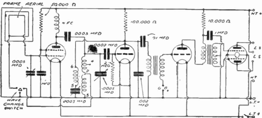
FIG. 119.—Circuit No. 21: A Four-valve Portable.
