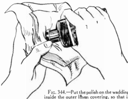
FIG. 344.—Put the polish on the wadding inside the outer linen covering, so that it just squeezes through.
