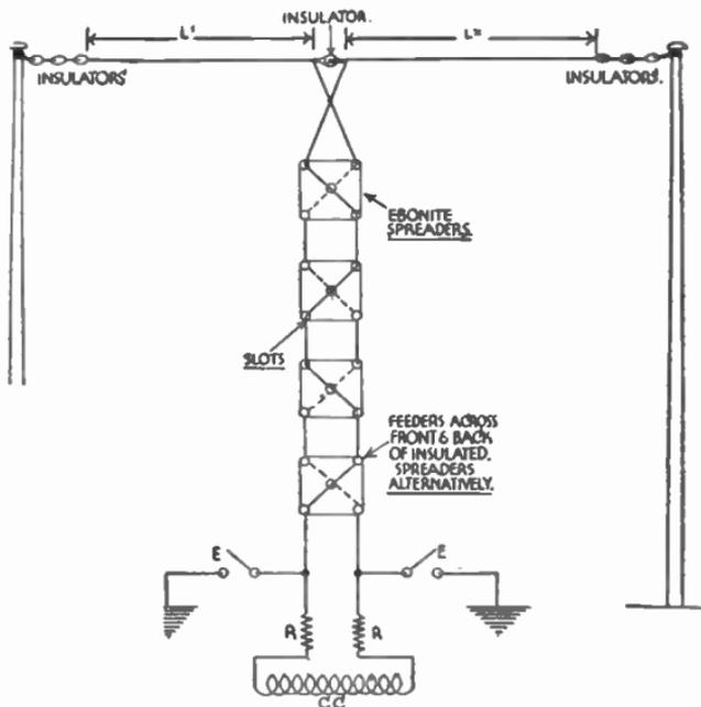
FIG. 197A.—Transposed or horizontal doublet aerial. E=earthing switches. CC=coupling coil. RR=600-ohm resistances.  $L^1, L^2=40$ -ft. aerials.
