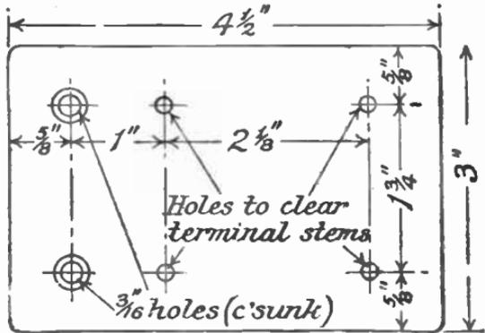
FIG. 45.—How to mark out the Ebonite Base.
