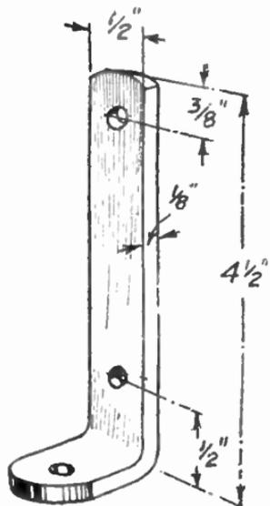
FIG. 265A.—Dimensions of supporting foot of Transformer.
