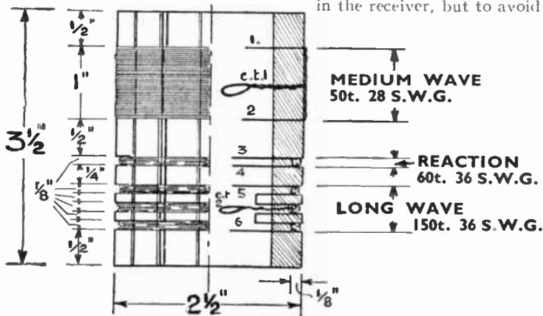
FIG. 434.—Constructional details of a Tuner made on an eight-ribbed 2½-in. diameter Ebonite Former. All turns are wound in the same direction.
