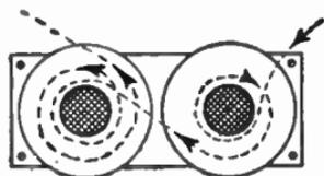
FIG. 395.—Showing how the Magnets are wound.
