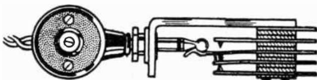
FIG. 385.—Typical Plug and Jack.
