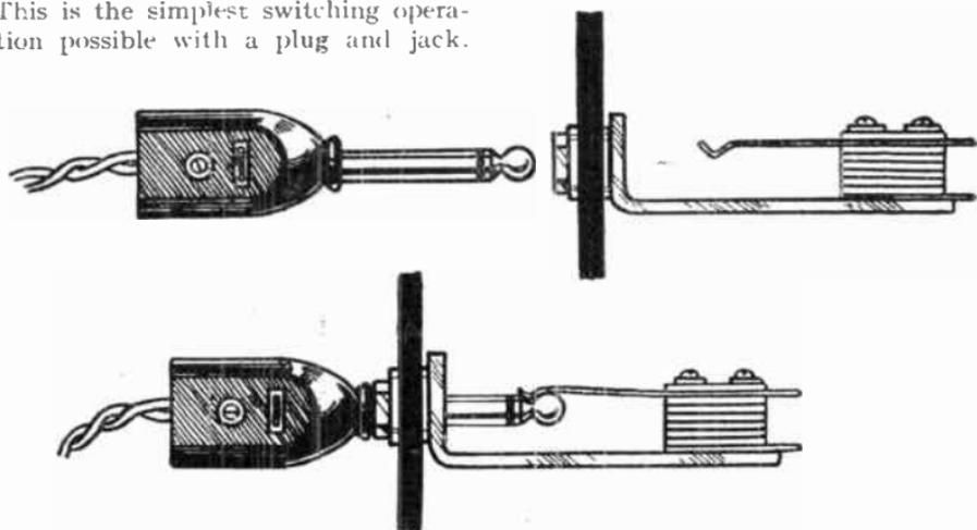
FIG. 327.—How the Plug and Jack connect.
