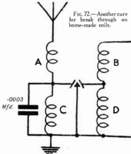
FIG. 72.—Another cure for break through on home-made coils.
