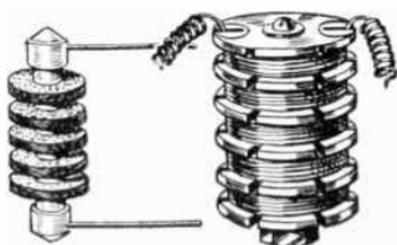
FIG. 214.—Typical short-wave and broadcast-band H.F. Chokes with sectional windings.
