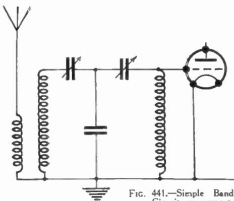
FIG. 441.—Simple Band-pass Circuit arrangement.
