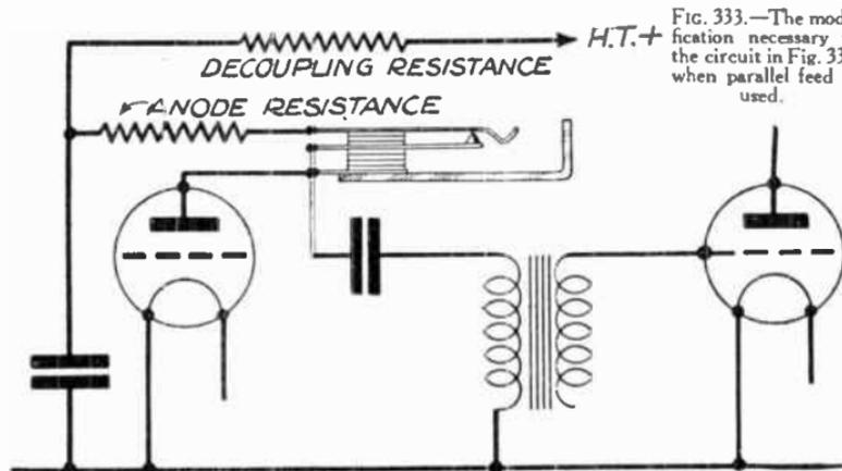
FIG. 333.—The modification necessary to the circuit in Fig. 334 when parallel feed is used.
