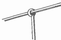
FIG. 362.—A wire to be attached at right angles to another should be looped together as shown.
