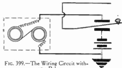
FIG. 399.—The Wiring Circuit without a Relay.
