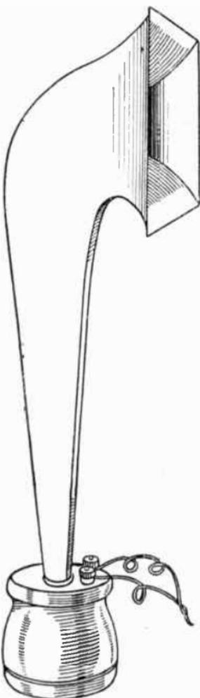
FIG. 250.—"Straight" Pattern Logarithmic Horn.
