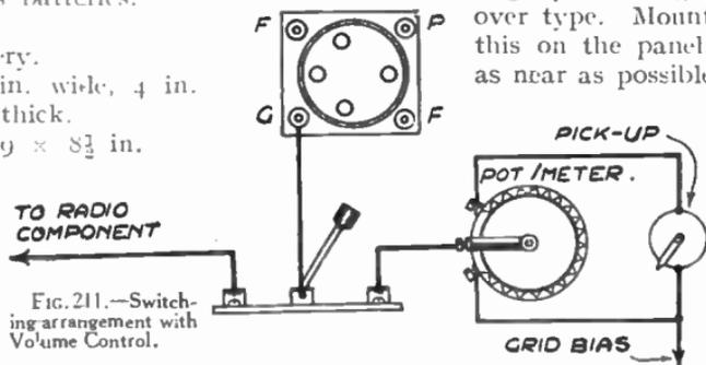
FIG. 211.—Switching arrangement with Volume Control.
