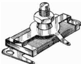
FIG. 288.—Suitable Potentiometer for eliminating Hum.
