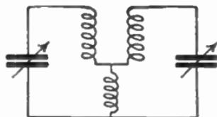
FIG. 175B.—Coil common to both tuned circuits.
