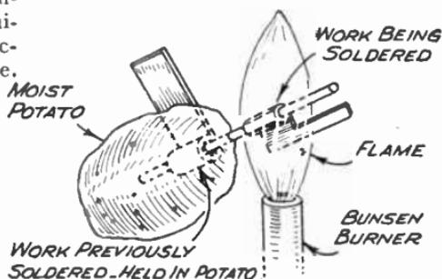
FIG. 369.—A typical case where a potato comes in useful.
