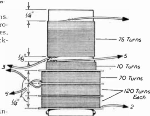
FIG. 151.—Here are the details for an oscillator coil for use with the I.F. transformer shown above.
