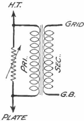
FIG. 471.—A simple form of Control in conjunction with the L.F. transformer.
