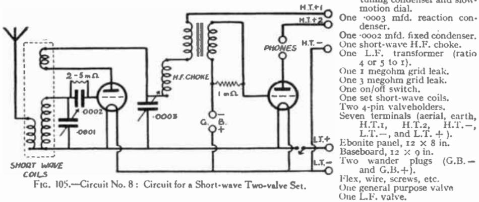
FIG. 105.—Circuit No. 8: Circuit for a Short-wave Two-valve Set.
