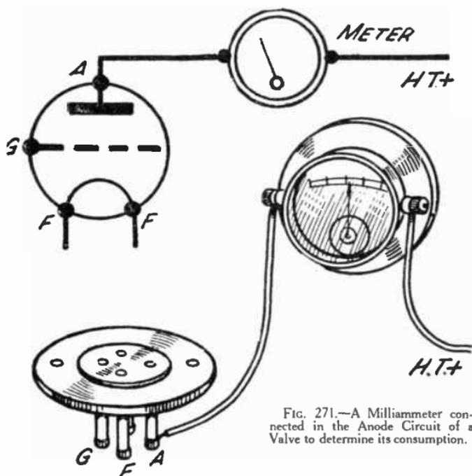
FIG. 271.—A Milliammeter connected in the Anode Circuit of a Valve to determine its consumption.
