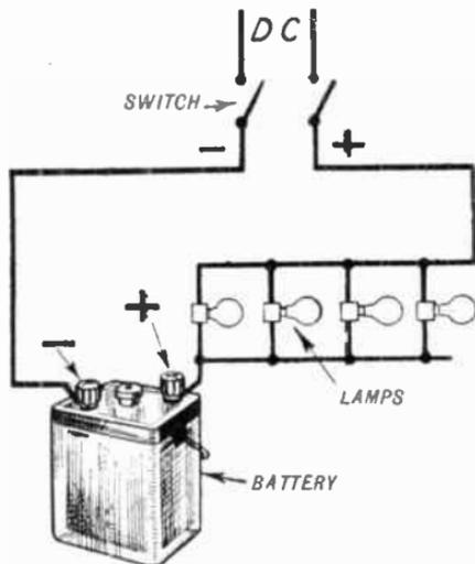
FIG. 24c.—The complete Charging Circuit.
