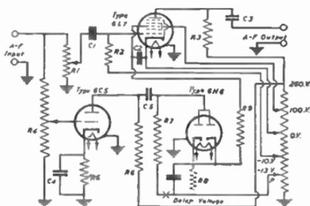
FIG. 478A.—Circuit incorporating Volume Expansion.
