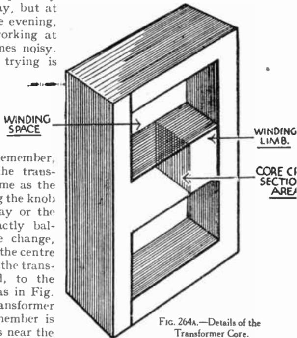
FIG. 264A.—Details of the Transformer Core.
