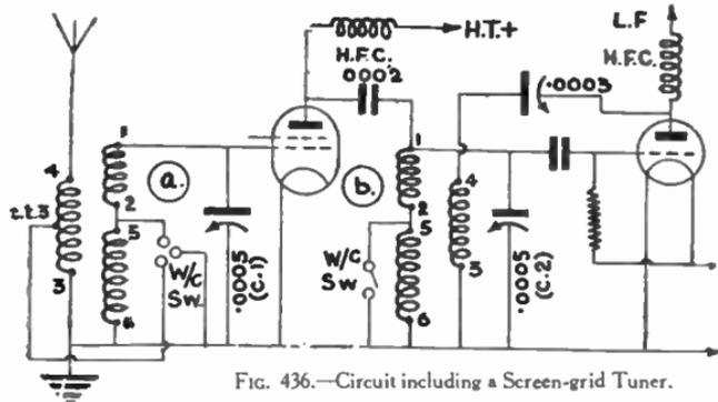
FIG. 436.—Circuit including a Screen-grid Tuner.
