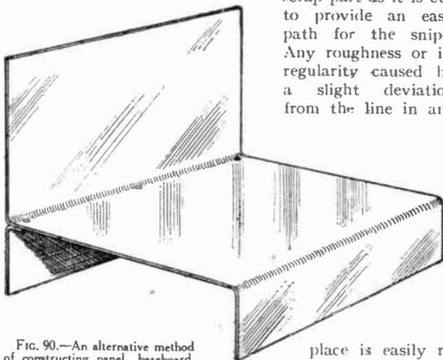
FIG. 90.—An alternative method of constructing panel, baseboard, and terminal strip in one piece.
