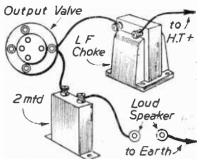
FIG. 354.—The Filter Output Circuit. See also Fig. 191.
