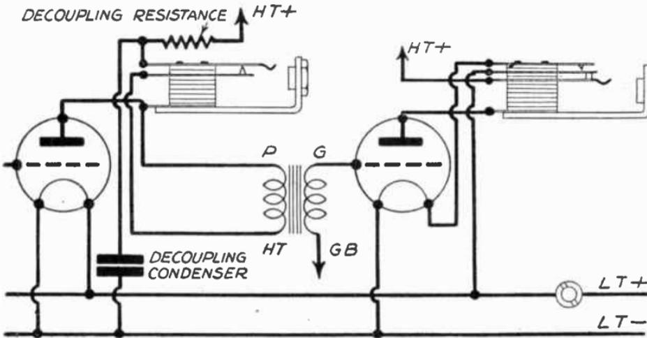
FIG. 334.—One or two L.F. stages can be used at will in this circuit.
