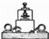
FIG. 402.—The Bridge which carries the Screw to adjust the tension of the Armature.
