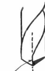
FIG. 179.—Grinding groove edge of twist to prevent the drill digging in on brass work.
