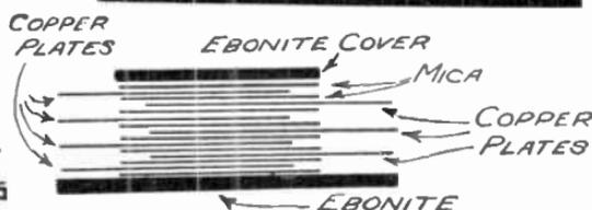
FIG. 159.—How the Condenser is clamped together.
