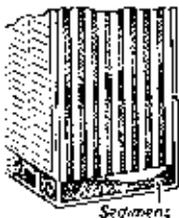
FIG. 23. *Sediment should be removed periodically, to prevent short-circuiting of plates.*
