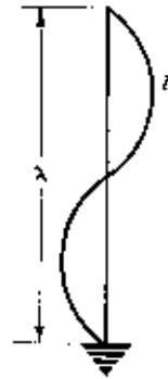
FIG. 35. Cancellation of radiation when aerial length is a multiple of  $\lambda$ .
