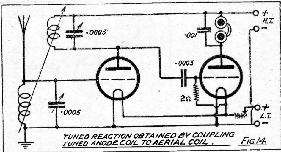
for rectification? The answer may be summed up in two words—Reliability and Reaction. The valve detector eliminates the delicate adjustment and uncertainty of the crystal rectifier, and in addition eliminates the damping effect which a crystal exerts on the circuit across which it is connected, and which results in flat tuning.
