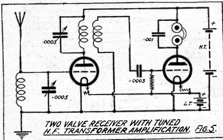
with proper H.T. voltage no added grid potential is required.
