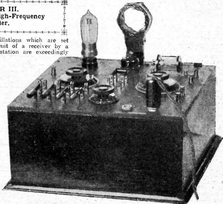
A "P.W." Combination one-valve reflex receiver constructed by a reader of "P.W." The coil at the back is the anode loading coil.
