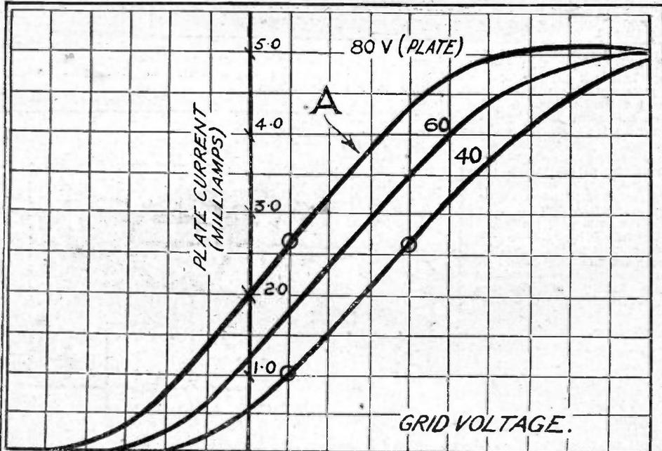
FIG. 1. VALVE CHARACTERISTIC CURVES.
