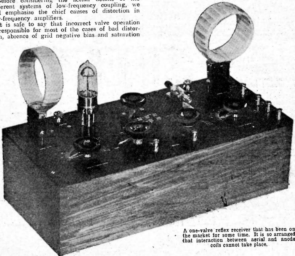
A one-valve reflex receiver that has been on the market for some time. It is so arranged that interaction between aerial and anode coils cannot take place.
