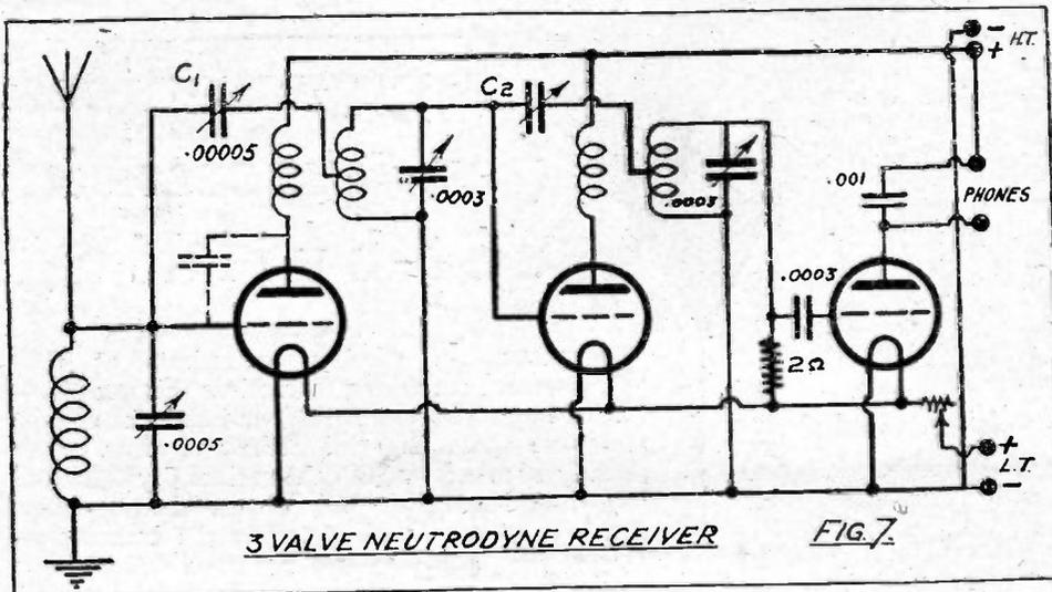
condenser are usually not critical, and in this country .0003 mfd. for the condenser and 2 megohms (2 million ohms) for the leak are in common use.
