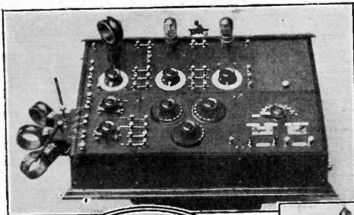
Left : A Two-valve Unit Set built up in cabinet form.
