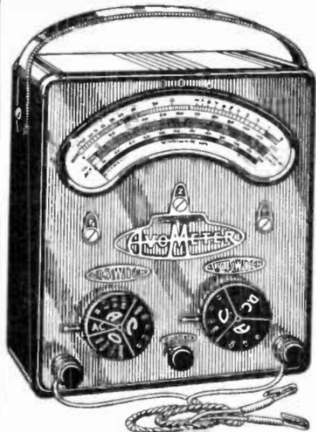
FIG. 275.—An all-in-one instrument.
