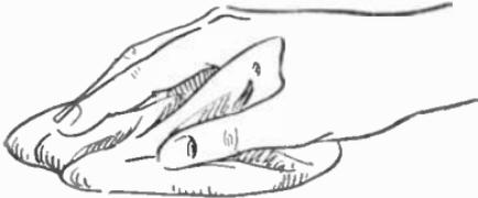
FIG. 345.—How to hold the polishing rubber.
