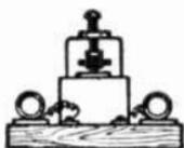
FIG. 402.—The Bridge which carries the Screw to adjust the tension of the Armature.
