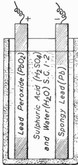
FIG. 19.—State of cell when charged.
