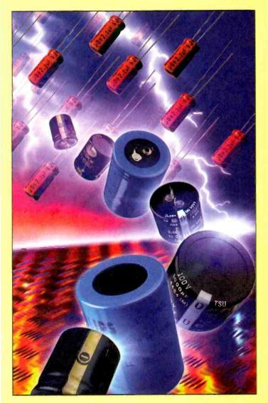
When an aluminium electrolytic capacitor fails, it rarely goes open- or short-circuit. To make matters worse, even its measured capacitance may seem OK. So how do you detect a failed electrolytic? Cyril Bateman explains. capacitor that fails open- or short-circuit can be quickly identified while it is still mounted on the PCB. Most ceramic, plastic-film and tantalum capacitor failures result in a short-circuited component and are relatively easy to locate<sup>1</sup>.
