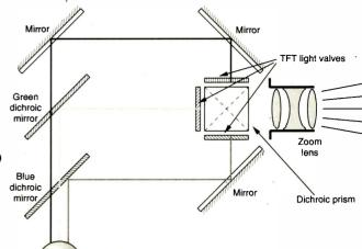
Fig. 1: Basic layout of a light-valve projector. Three TFT liquid-crystal panels modulate the R, G and B light, which is then combined by a dichroic prism.
