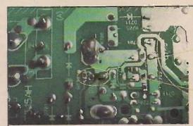
Disconnect either R734 or D721 to disable the standby operation of the power supply
