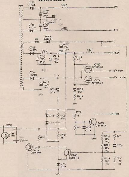
standby. If Q707 is faulty it's a good idea to replace C714 as well, even if it has been replaced before.
