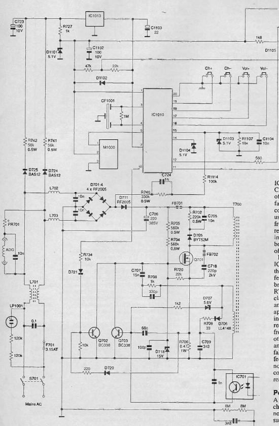
IC1008 and IC1009. Ceramic filter CF1001 determines the frequency of the sync signal. If CF1001 is faulty, there will be no communication with IC1001. The usual symptoms are failure of the front buttons to operate and the remote-control system being inactive. These symptoms will also be present when the voltage at pin 1 of IC1010 is below 3-5V.
