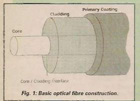
passing through Romsey en-route to Salisbury via the A27. It will presumably then go farther for future activity all over the country. This is not just for regional but also international communications. Fibre-optic communication is cheap, signal transmission delays are minimal, operation is totally secure, there's immunity to interference both inductive and electromagnetic, the bandwidth is wide and is suitable for data, voice and video, digital and analogue.
