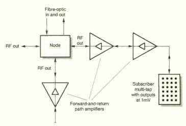
Fig. 5: Typical HFC network.
