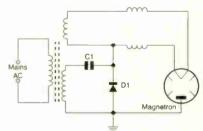
Fig. 1: The basic magnetron circuit.
