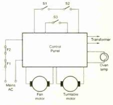
Fig. 2: Block diagram of the LV/control section.
