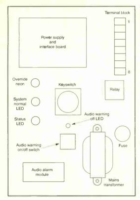
Fig. 10: Suggested locations of the various items inside the control box. Component layout for the power supply and interface board and the audio alarm module is not critical in any respect. Drill fixing holes for the power supply and interface board to match mounting pillars in the box. Terminal block connections are as follows: 1 signal in; 2 +9V out; 3 0V; 4 mains live in; 5 mains neutral in; 6 earth; 7 and 8 relay contacts (mains or motor control).
