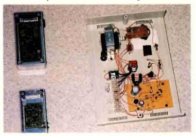
Internal views of the assembled IR transmitter, IR receiver and control boxes.
