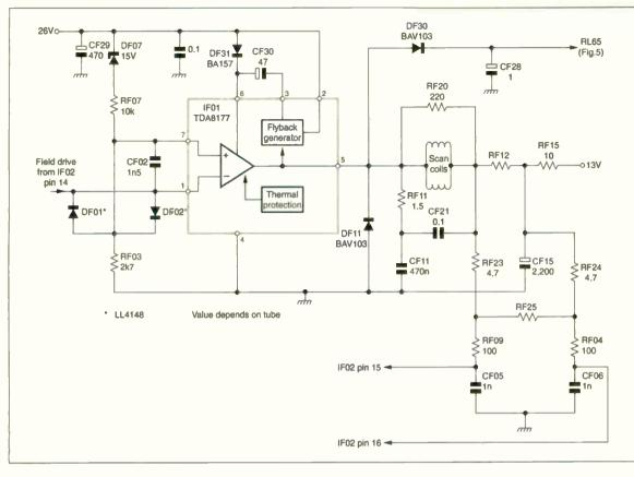
Fig. 7: The field output stage circuit used in the Thomson TX92 chassis
