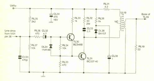
Fig. 4: The line driver stage circuit used in the Thomson TX92 chassis.
