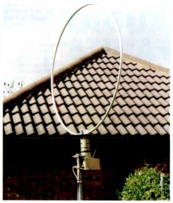
The Wellbrook Communications ALA1530 wideband MF/HF active loop aerial, mounted at 2.2m. Results have been excellent.
