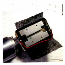
Photo 5: The pole-pieces, with some corrosion still present.
