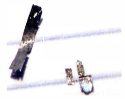
Photo 4: The remains of the original ribbon element.
