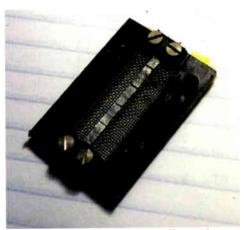
Photo 3: The ribbon had been affected by corrosion, which had created two holes.
