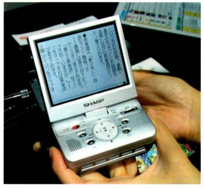
The Sharp 4E-MB1 mobile AV player, which has a 3.6 in. LCD screen, is due for a November launch.
