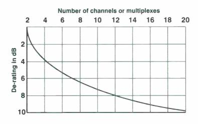
Fig. 19: Assuming that all channels are of the same strength, there is a simple relationship between the number of channels and an amplifier's maximum output.
