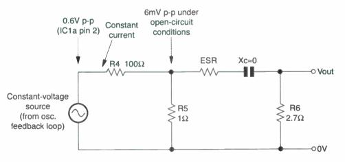
Fig. 5: The method of test capacitor interface used in this meter. The source voltage is not a true constant voltage because of the need for R6, whose value must be comparable to the ESR of the capacitors in which we are interested.
