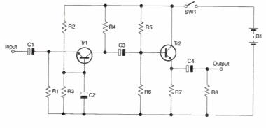
Fig. 2: The preamplifier circuit.
