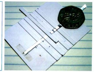
Photo 6: Making the indentations in the replacement foil ribbon.
