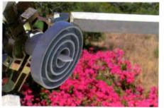
Photo 12: A plastic depolariser inserted in the feedhorn of an H/V LNB.
