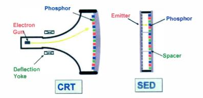
Fig. 1: Comparison between a CRT and an SED. Both rely on electrons striking a phosphor-coated screen to produce light.
