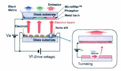
Fig. 2: How the SED electron emitters operate.
