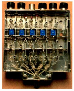
Fig. 21: A five-channel filter unit with the rear cover removed. In this example all five channel paths share one input. From top to bottom, each path has a tuned stage, a variable attenuator (blue) then two more tuned stages.
