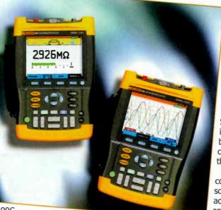
A wide choice of automatic and manual trigger modes gives you the flexibility to capture just about any signal you will encounter. Connect-and-View triggering is ideal for fast and easy checking of multiple test-points.
