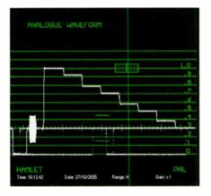
Figure 1: Luminance waveform display
