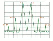
Figure 2: Two tone intermodulation analysis
