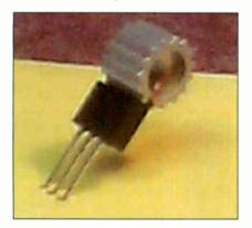
Failure of the CD to operate in this budget Hi Fi, with the laser not even homing, was caused by a defective 8v regulator transistor, Q701. Its type was completely unrecognisable, even to www.datasheetarchive.com and it's very rare to beat this excellent free-to-use web resource.
