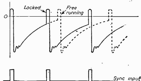
Fig. 4.—This diagram shows how the free-running condition is taken charge of by the Hold setting.
