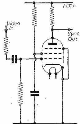
Fig. 1.—The ordinary pentode sync separator.
