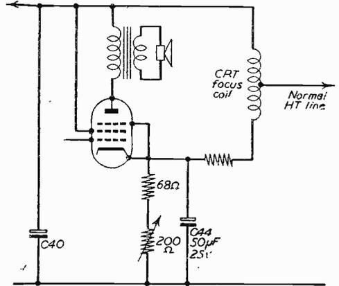
Fig. 3.—Showing the effect of the sound output stage on focusing.
