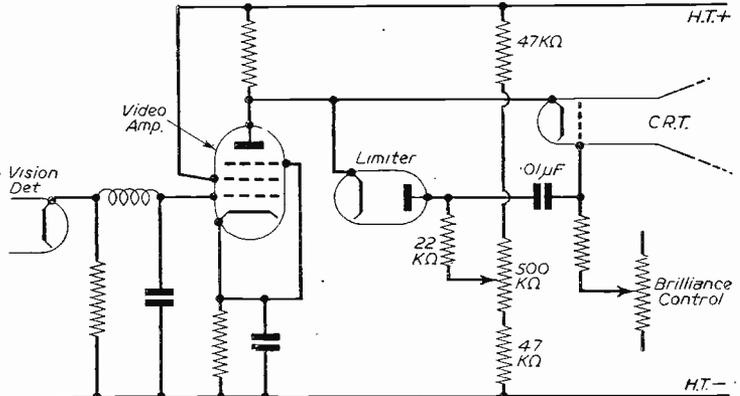
The extra amplification needed for the limiter circuit is obtained by using a tapped video load and it is an advantage to increase the H.T., if possible, to compensate for this additional resistance.
