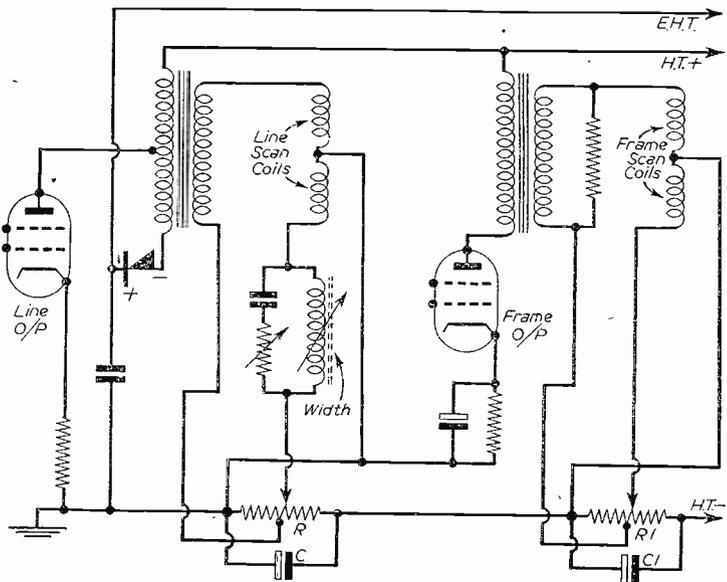
Fig. 5. — Circuit for two shift controls — frame and line.
