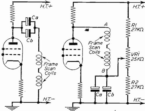
Fig. 3 (left). — Normal high impedance frame circuit.
