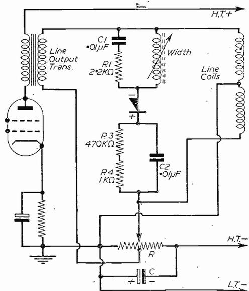
Fig. 2.—Method to be used when a damping diode is included.
