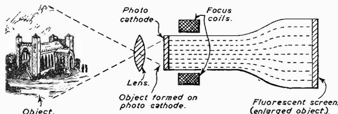
General schematic view of a cathode-ray tube.
