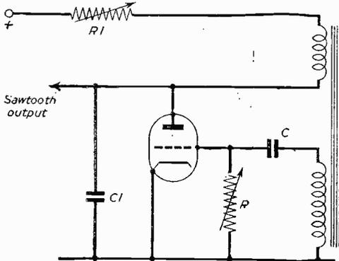
Fig. 3.—The variable resistor, R1, affects the amplitude and also the linearity of the waveform.
