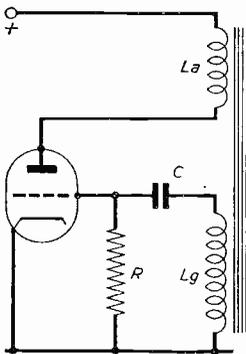
Fig. 1.—A typical circuit of a blocking oscillator.
