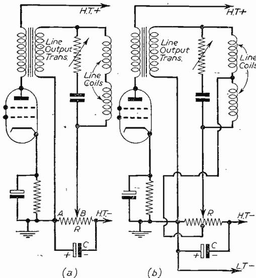
Fig. 1 (a) and (b).—Two methods of obtaining line shift.
