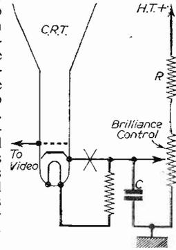
Fig. 3.—Basic tube circuit.
