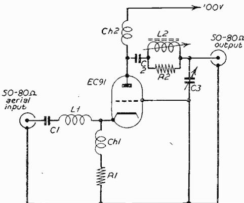
Fig. 1. — A single stage, grounded-grid amplifier.
