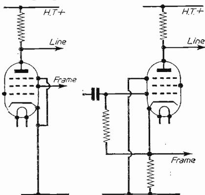
Fig. 2.—Two methods of taking out the sync. pulses to avoid interaction.
