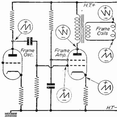
Fig. 2.—Showing sawtooth waveform at different points.
