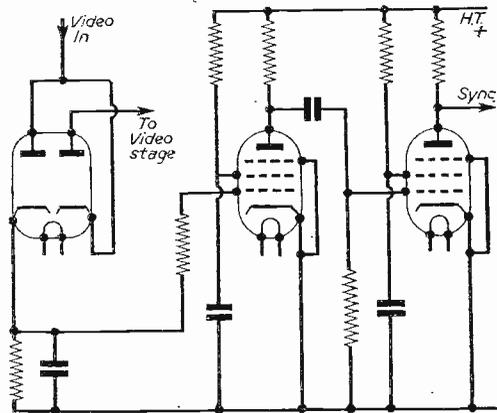
Fig. 3.—The ideal sync separator arrangement, with isolation of picture pulses.
