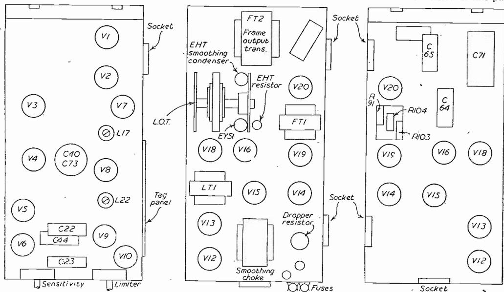
Fig. 1 (left).—Under-chassis view of R.F. unit. C22 and 23 are video amplifier electrolytics; C40 and 73 are main smoothing condensers; C44 is sound output bias condenser. (Centre).—Top view of timebase and power unit, and (right) underview of this unit in which C71 is series framehold resistor, C64 and 65 are frame-output electrolytics, and R103
