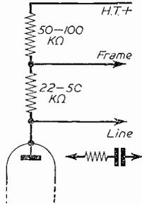
Fig. 4. — Another method of isolating the sync. pulses.
