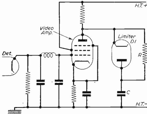
Fig. 1.—Simple automatic type of vision limiter.
