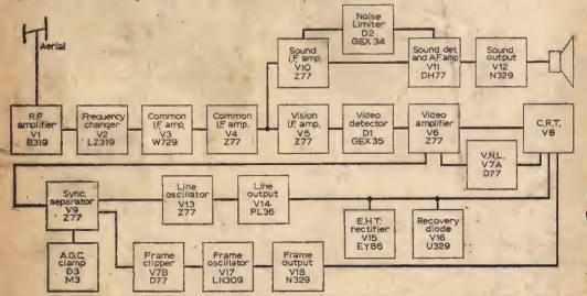
Block diagram of receiver suitable for adaptation to sound-only operation. Best receivers for this purpose have a multi-channel tuner and 0.3A or 6.3V valves.
