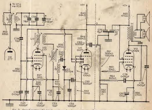
Fig. 2-Sound section of typical receiver, showing sound take-off circuit from common i.f. amplifier.
