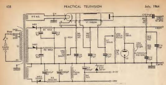
Fig. 1-Circuit of the camera power supplies.
