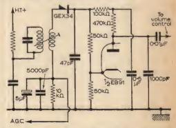
Fig. 15—Decca DM4, etc., detector and noise limiter, using both thermionic valve and semiconductor diade.
