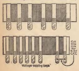
Fig. S (left)—The mains resistors of the V600 and V700 models.
