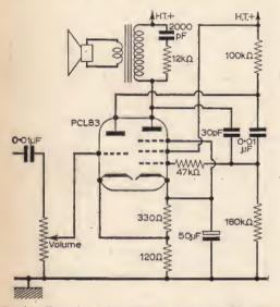
Fig. 16—Typical sound output stage (Ferguson 306). Note tapped cathode bias, correction companents across output transformer primary and 30pF compensating capacitor from anode to control grid of pentode section.
