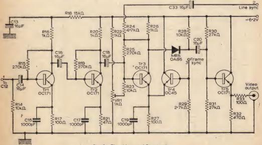
Fig. 2—The video amplifier circuit.
