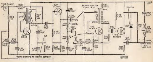
Fig. 3-The timebases and sync stages of the circuit.
