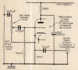
Fig. 4—The cathode-fallower stage. This feeds high quality TV sound to a tape recorder or amplifier and works independent of the audio stages in the soundonly receiver.
