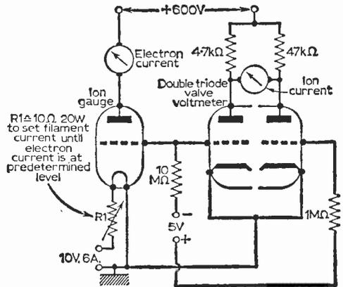
Fig. 2: Method of setting up ion gauge.
