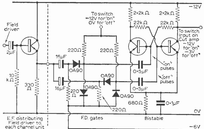
Fig. 52: Additional circuitry for inter-field cutting.
