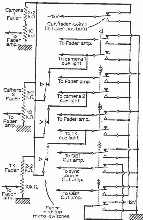
Fig. 57: D.C. control of cut/fade vision mixer
