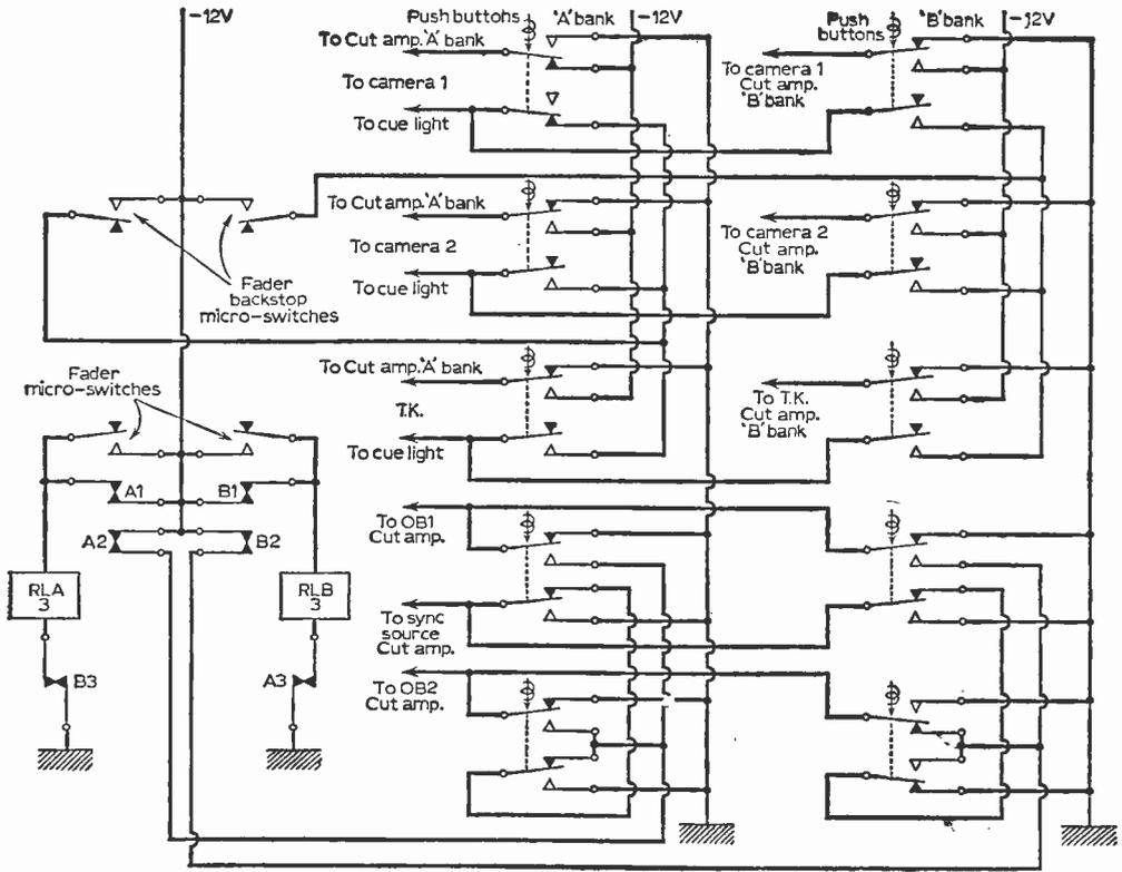
Fig. 55: A/B mixer d.c. switching.
