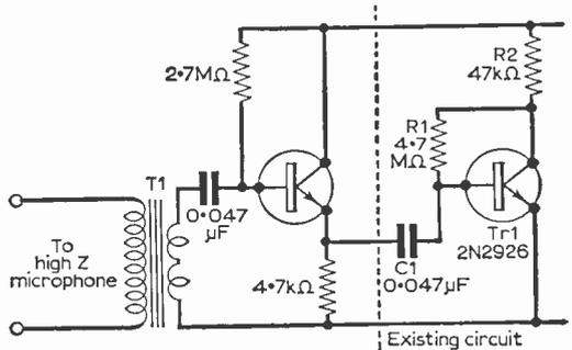
Fig. 2 (right): Impedance matching unit that can be added to the standard circuit to enable a high impedance microphone to be used.
