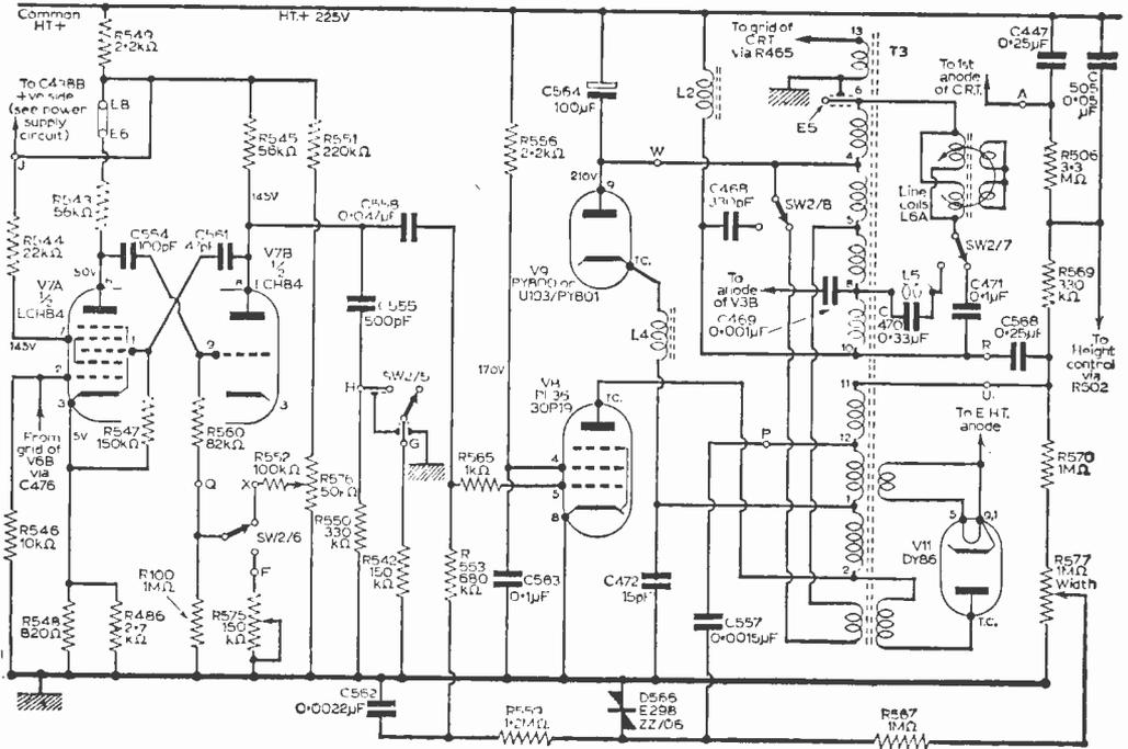
Fig. 5: Circuit of the line timebase
