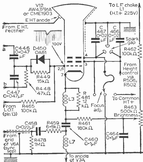
Fig. 4: Cathode-ray tube circuitry.
