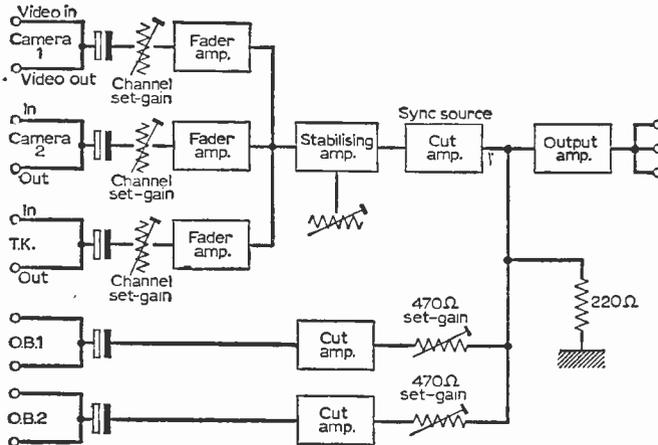
Fig. 56: Vision schematic for cut/fade vision mixer.
