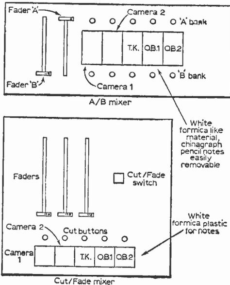
Fig. 58: Layout of mixer control panels.
