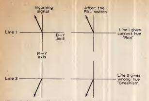
Alternate lines of a field are Red and Green in this example Fig. 23: Vector diagrams showing why a stopped PAL switch causes the overall hue displayed to be the sum of the correct one plus its mirror image. The individual hues can be seen at close range and cause severe blinds.
