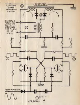
Fig. 24 : A typical bistable PAL switch circuit. Five quick checks with an oscilloscope at the points shown will isolate the fault to a particular part of the circuit.
