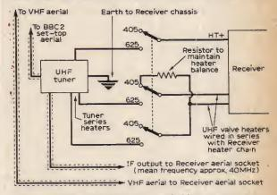
Fig. 1: Simple 405-625 power switching arrangement.
