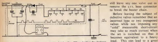
Fig. 4: Typical heater and h.t. power supply circuits. When testing for leakage across the h.t. rail and chassis remember that if the ohmmeter applies a negative potential to the BY100 cathode this will be forward biased and conductivity will be measured through the BY100 and heater chain as well as through any leakage.
