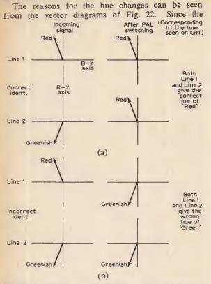
Fig. 22: Vector diagrams showing why incorrect ident results in a hue which is the mirror image of the correct one. (a) Vectors under correct ident conditions. (b) Vectors under incorrect ident conditions. There are no blinds present on the picture when the fault is incorrect ident.
