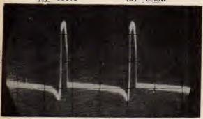
Fig. 9: Equal but opposite phase sync pulses are fed to the two flywheel sync discriminator diodes.
