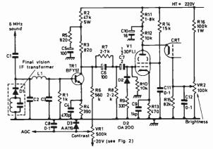
Fig. 1: The suggested video amplifier and a.g.c. circuit. A 6MHz rejector should be included in series with the grid or cathode of V1.
