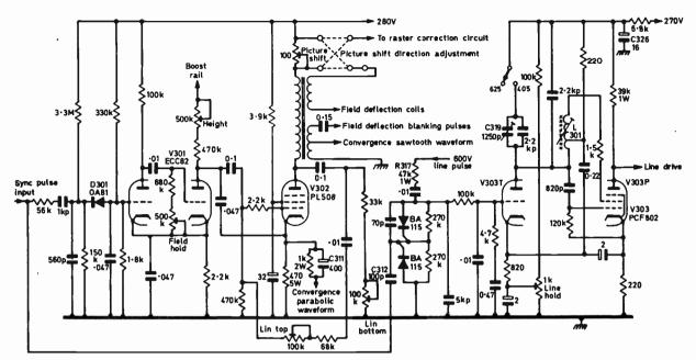
Fig. 1: Circuit of the Decca dual-standard timebase panel on which the line and field generators and field output stage are mounted. R317 47k $\Omega$  is a "favourite" in many chassis. It is 3R1 in dual-standard Rank-Bush-Murphy sets.
