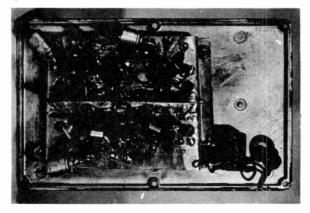
Internal layout of the preamplifier.
