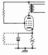
Fig. 1: If a cathode bias resistor goes opencircuit the full h.t. then appearing across the bypass capacitor will break it down forming a leakage path. This will act as a "bias resistor" but of the wrong value, resulting in bottom cramping.
