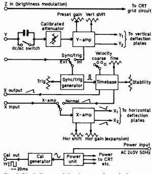
Fig. 4: Block diagram of the elements of a typical oscilloscope.
