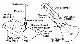
Fig. 1 (left): A mechanical analogy of the operation of an oscilloscope. Fig. 2 (right): Simplified sketch of the instrument type c.r.t. used in a typical oscilloscope.
