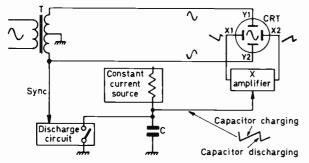
Fig. 3: The basic oscilloscope principle.
