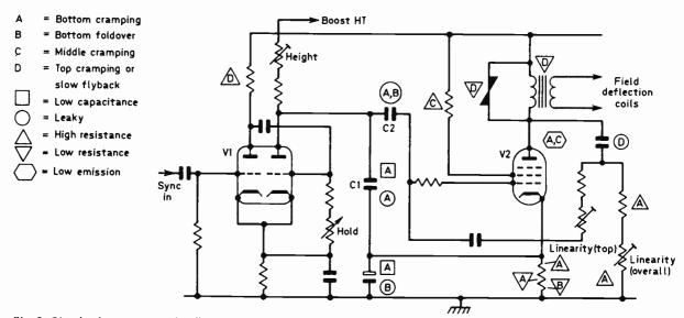
Fig. 2: Circuit of a representative field generator and output stage showing likely component defects and their effects on linearity.
