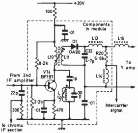
Fig. 2: The third i.f. amplifier and luminance detector stages of the Bush-Murphy single-standard circuit.
