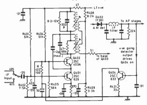
Fig. 1: Cascode sound i.f. amplifier used in the Sony Model TV9-90UB, with a.g.c. applied to Q402 base.
