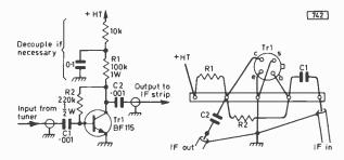
Fig. 1 (left): Simple untuned transistor i.f. stage.
