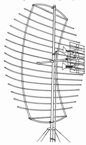
Drawing of the Channel Master paraboloid "Super Panascope" u.h.f. aerial,
