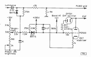
Fig. 3: Beam limiting arrangement used in conjunction with a PD500 e.h.t. stabiliser triode.
