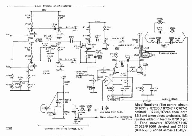
Fig. 11: The colour-difference amplifiers and the audio channel.
