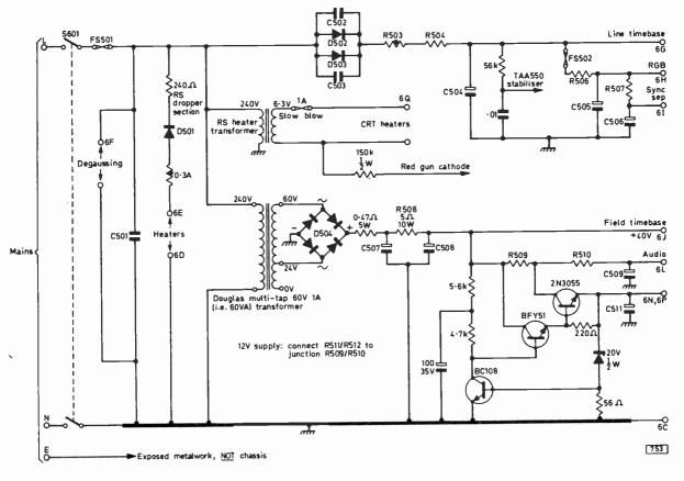
Fig. 1: Power supply circuit used by L. Cook, with stabilised 20V line. 36V a.c. is obtained across the 24V and 60V taps on the secondary winding of the Douglas multi-tap transformer.
