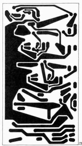
Fig. 6 (left): Layout of E. Erven's power supply, viewed from the component side. C1, C7/8, C14 and C15 are mounted off the board.
