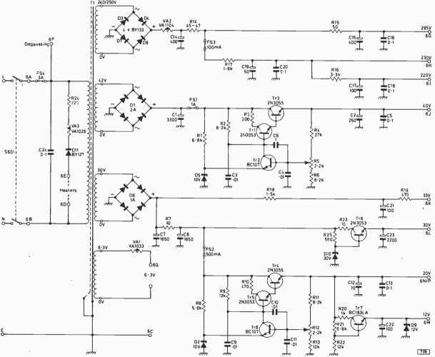
Fig. 4: Power supply circuit designed for the receiver by E. Erven, with stabilised 40V and 20V outputs. R14 can be made up from the  $30\Omega$  and  $15\Omega$  resistors (R504 and R509) supplied in the original component pack.
