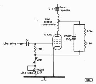
Fig. 1: Line output valve grid circuit of the Philips G6 chassis (single-standard version). The complaint was occasional erratic width reduction.
