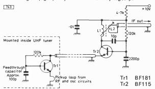
Fig. 3: Cascode mixer-amplifier circuit.
