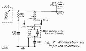
second vision i.f. stage. This (see Fig. 2) is switched into circuit on 405 only by using the otherwise redundant 2S1a—the rejector can be mounted adjacent to the switch by means of a solder tag.
