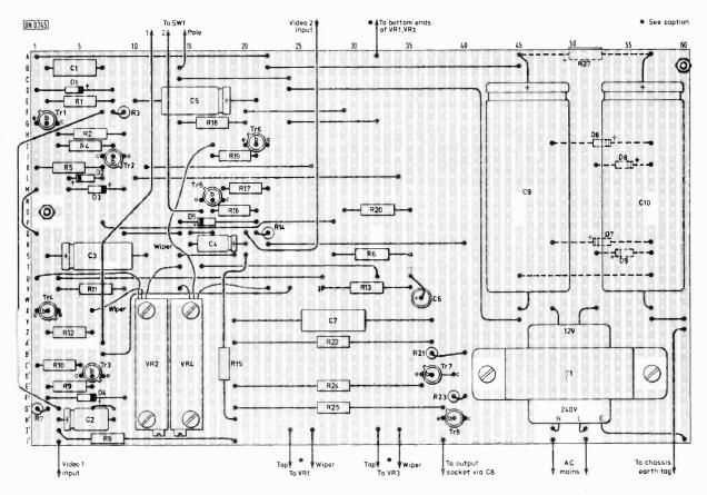
Fig. 4: Veroboard layout, viewed from the component side (0.1 in. Veroboard used). R27 and D6-9 are mounted on the copper side. Connections to VR1 and VR3 can be made via flying leads or if sliding potentiometers are used (as in the prototype) these can be soldered directly to the copper side. Ensure that the mains connections are well insulated from the rest of the circuit board.
