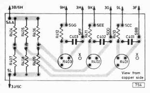
Fig. 5: The small board used by E. Erven to mount the RGB drive controls: drill  $\frac{1}{8}$  in. holes in the positions marked X to secure the board to two of the RGB output transistor heatsinks—ensure that the board is insulated from the heatsinks. Shown half scale (viewed from the copper strip side).
