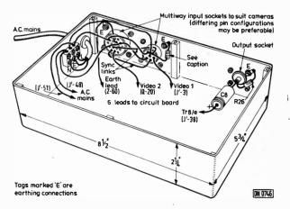
Fig. 2: Wiring to the case. The board and the controls are mounted on the lid of the diecast box. The resistor (say  $100\Omega$ ) shown terminating the sync link at the camera 1 socket may be necessary to match sync lines.
