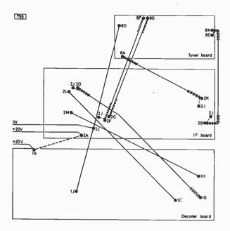
Fig. 3 (left): Arrangement of the three signal boards sideby-side adopted by E. Erven. This arrangement can be used only with 22in. or larger c.r.t.s. If a single regulated 20V line is used, add the link shown in broken line between 1A and 2A and use only one 20V connection to the power supply. Note that this diagram shows the interconnections between the three boards only.
