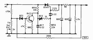
Fig. 2: The stabilised thyristor power supply circuit used in the RBM single-standard chassis.
