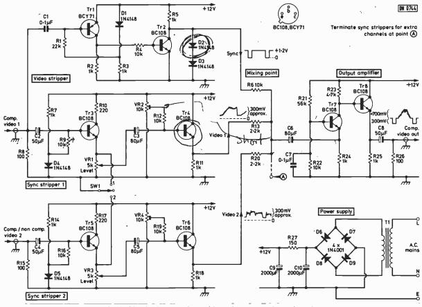
Fig. 1: Circuit diagram of the video mixer—two-channel version.
