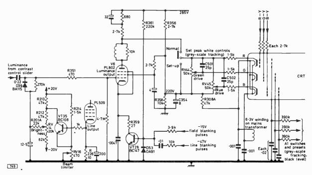
Fig. 1: The luminance output circuit used in the Pye 691 chassis, showing the brightness control, flyback blanking and beam limiting arrangements.
