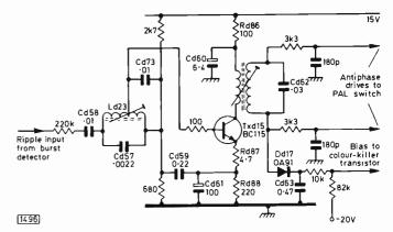
Fig. 3: The ident amplifier and colour-killer circuits.
