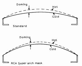
Fig. 6: Comparing doming with standard mask (top) and RCA Super Arch Mask (bottom).
