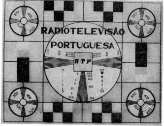
The test card being used by RTP at u.h.f. – it was also used for earlier v.h.f. transmissions.
