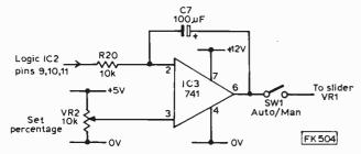
Fig. 5: Use of an additional i.c. to give automatic level setting. VR2 sets the black/white ratio: clockwise rotation gives more white, anticlockwise rotation more black, with 50:50 black/white when the potentiometer is set at the centre of its range.
