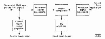
Fig. 1: Block diagram of the basic head servo system in the record mode.
