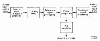
Fig. 2: Block diagram of the basic head servo system in the playback mode.
