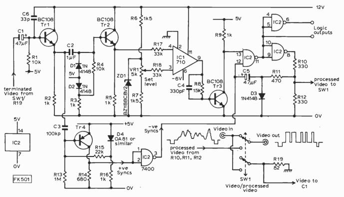
Fig. 1: Circuit of the slicing, logic and sync sections of the unit. Tr4 is type 2N3702 or equivalent.
