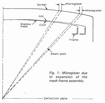
restrained at the edges by the slower heating frame, it tends to dome or increase its curvature and thus reduces the mask-to-screen spacing as shown in Fig. 3.
