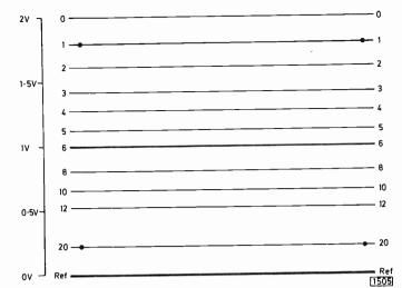
Fig. 4: A dB graticule for display units, plotted against a vertical scale of O-2V (the typical output of a diode vision detector).
