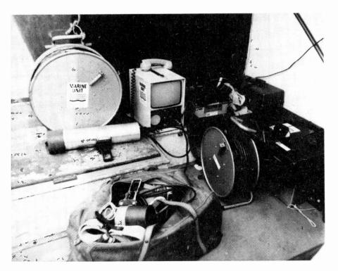
Photograph of the items comprising the system. The camera in the foreground, on the tool bag, is the vidicon type. The camera in the centre left, in front of the cable drum, is the silicon type.
