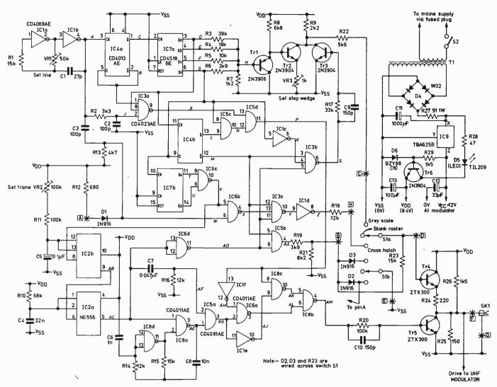
Fig. 2: Circuit diagram of the logic and power supply sections of the pattern generator. Starred points indicate connections off the printed board. Italic letters identify waveforms shown in Figs. 4 and 5, which will appear next month.
