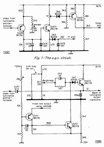
Fig. 2: The beam limiter and brightness/d.c. restorer circuit.
