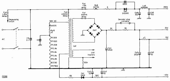
Fig. 6: The power supply circuitry.
