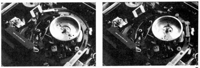
Photographs showing the interior of the machine as the tape starts to leave the cassette.
