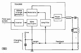
Fig. 2: Block diagram of the TDA2600 class D field timebase.
