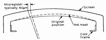
Fig. 3: Shadowmask doming during the initial minutes of tube operation.
