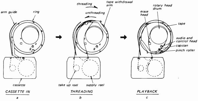
Fig. 4: How the tape is automatically threaded around the rotating video head drum by the tape withdrawal arm.
