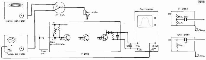
Fig. 1: The basic alignment hook-up.
