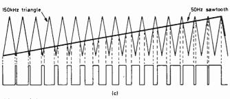
Fig. 1: (a) An LC filter fed with a switched 0-30V squarewave input gives 15V d.c. output. (b) With a modulated, variable mark-space ratio squarewave input the LC filter gives a sawtooth output. (c) Generating a varying mark-space ratio squarewave by mixing a sawtooth waveform with a higher frequency triangle waveform.
