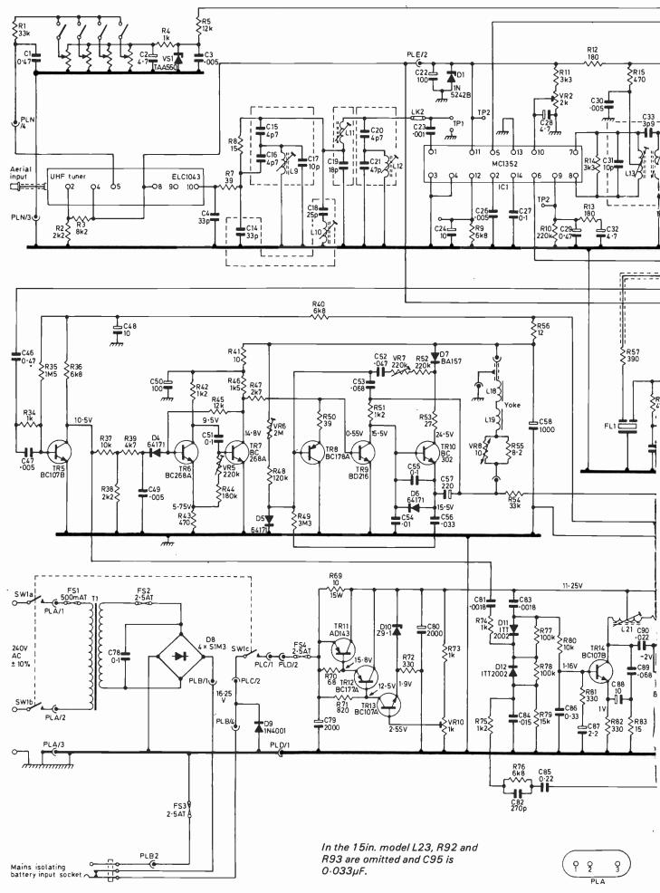
Fig. 1: Circuit diagram of the Decca Gypsy monochrome portable. Earlier sets were fitted with a rotary tune
