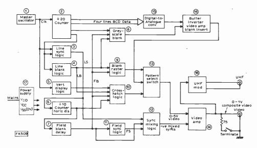
Fig. 1: Block diagram of the complete pattern generator.
