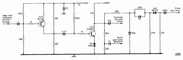
Fig. 5: The two-transistor sync separator circuit. Note that the burst gating pulses are derived from the sync pulses.
