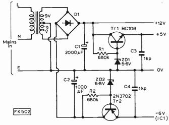
Fig. 2: The power supply circuit.
