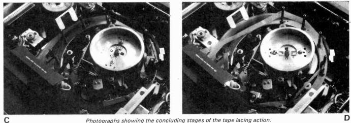
Photographs showing the concluding stages of the tape lacing action.
