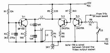
Fig. 3: Circuit diagram of the u.h.f. modulator.
