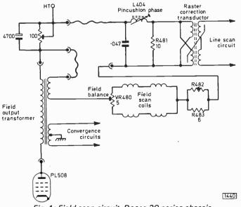
Fig. 1: Field scan circuit, Decca 30 series chassis.
