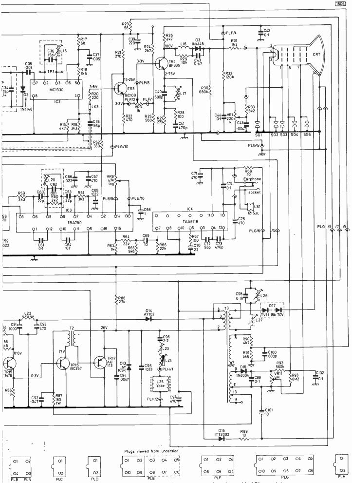
r while some sets have six channel selector buttons. An AU111 line output transistor is used in 15in. models.
