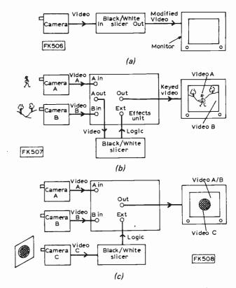
Fig. 4: Methods of using the unit. (a) As simple black/white slicer; (b) keying with effects unit and two cameras; (c) with a third camera to gate specific shapes into a picture.
