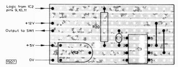
Fig. 6: Layout of the automatic level setting circuit on Veroboard. The 741 i.c. is available in various packages. This layout is for the widely available 8-pin d.i.l. pack.
