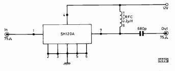
Fig. 2: Test circuit for the SH120A thick-film wideband signal preamplifier i.c. This version operates at 12V with a current consumption of 20mA. The input pin is d.c. isolated internally by means of a 680pF, 50V capacitor.
