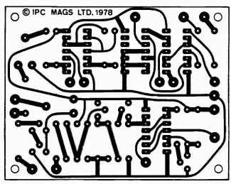
Fig. 2: Suggested printed board pattern for the unit.
