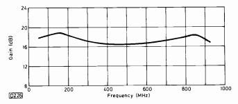
Fig. 3: Gain/frequency characteristic curve.
