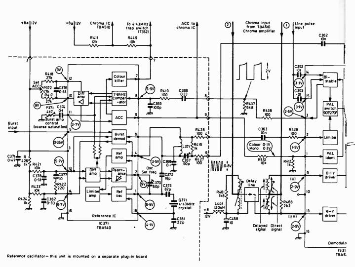
Fig. 15: The reference oscillator, demodulator and lumin
