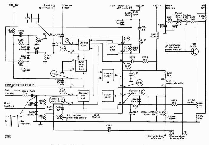
Fig. 14: The TBA510 chroma amplifier i.c. and its peripheral circuitry.
