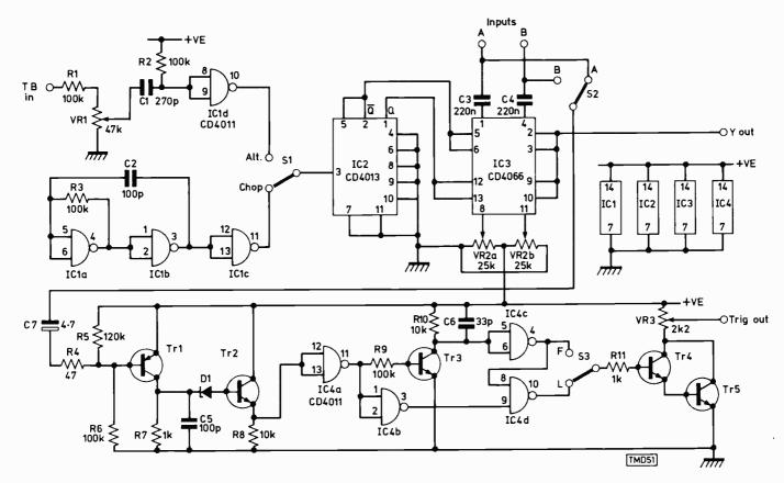
Fig. 3: Circuit diagram of the unit. The prototype operates with a 6V rail. A battery can be used to supply the power therefore.
