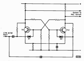
Fig. 8: A bistable multivibrator triggered at line frequency to provide 7 8kHz outputs to drive a PAL switch. Simplified by omission of the ident circuit which synchronises the PAL switching in the receiver with that at the transmitter.
