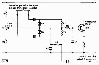
Fig. 4: Simple flywheel line sync discriminator circuit.
