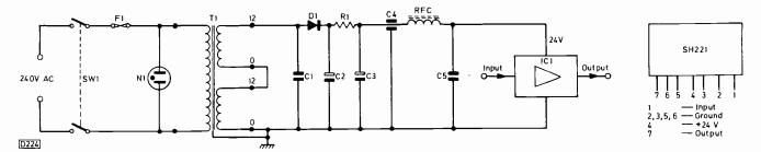
Fig. 1: Complete circuit left, SH221 pin connections right.
