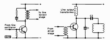
Fig. 5 (left): Basic features of a line driver stage. . Fig. 6 (right): Basic transistor line output stage circuit.
