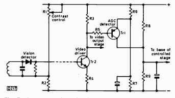
Fig. 7: A pnp transistor (Tr1) used as a peak detector to develop an a.g.c. bias proportional to sync pulse amplitude.
