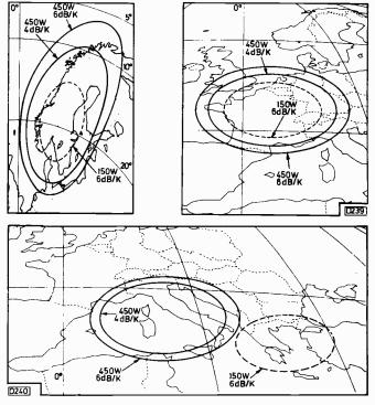
Examples of the OTS-2 satellite's European "footprints". Top left, coverage of Scandinavia by both beams (450 and 150W). Top right, coverage of Western Europe with both beams directed at the same area. Bottom, Southern European coverage, with the 450W beam directed at Italy and the 150W beam at Greece.
