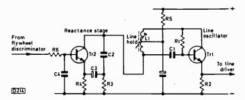
Fig. 3: Simplified line oscillator/reactance stage circuit.
