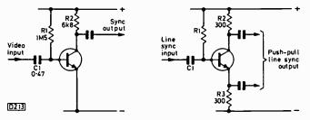
Fig. 1 (left): Typical sync separator stage.
