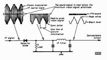
Fig. 4: Demodulation using a diode and LC filter.
