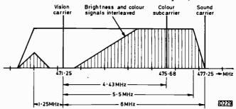
Fig. 1: Relative positions of the signals in a television channel. The carrier frequencies shown are for channel 21.
