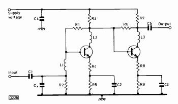
Fig. 5: Internal circuit of the SH221 thick-film wideband signal preamplifier i.c.
