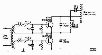
Fig. 2: Line output transistor circuit, Rank A823 chassis.
