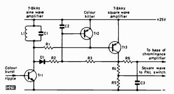
Fig. 9: The colour-killer arrangement used in the Thorn 8000 series chassis. The colour burst ripple input is taken from the burst detector: the ripple arises due to the phase changes  $(\pm 45^{\circ})$  of the burst signal on alternate lines.
