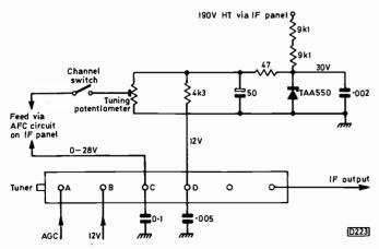
Fig. 1: Varicap tuner supplies, Pye 693/697 chassis. There are six channel selector switches/tuning potentiometers.
