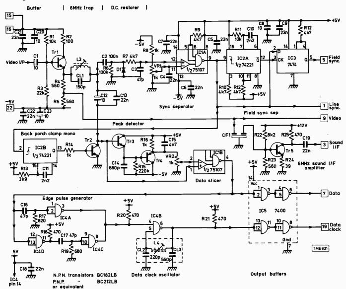
Fig. 1: Circuit diagram of the revised data recovery section. The i.f. section remains unchanged. R12 shown twice in error.
