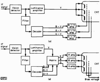
Fig. 1: Methods of driving a colour tube. (a) Colour-difference drive, with the luminance signal (Y) applied to the three cathodes and the three colour-difference signals applied to the grids. The tube then carries out the RGB matrixing, the phosphor screen being activated by the three primary-colour signals. (b) RGB drive. In this case matrixing is carried out prior to the tube, the RGB signals being applied (almost always) to the three cathodes.
