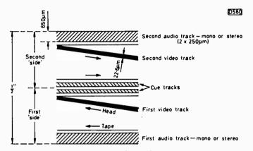
Fig. 1: Arrangement of the tracks on the tape.
