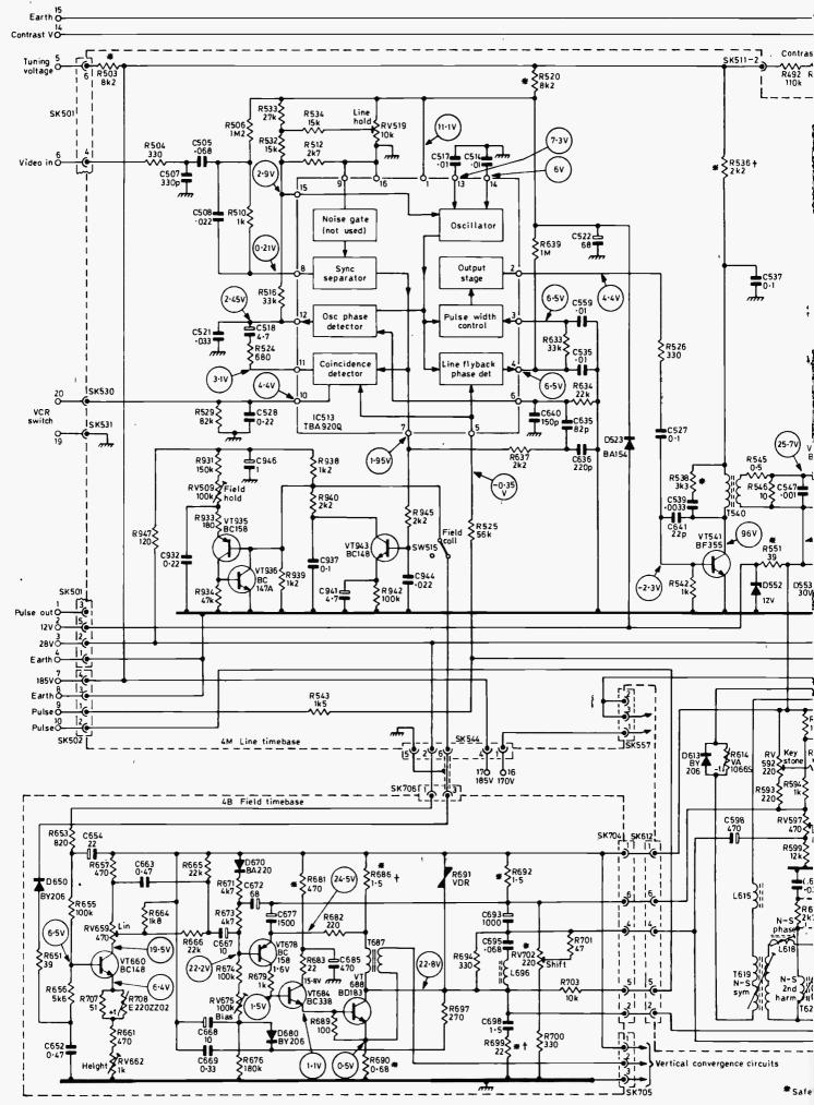
Fig. 1: The timebase, c.r.t. and power supply circuitry used in the 737 chassis. In earlier versions a gating pulse at pin 3 of SK501 is obtain
