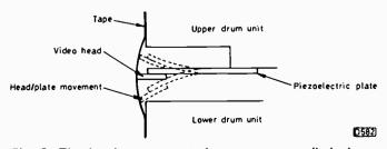
Fig. 3: The heads are mounted on servo-controlled piezoelectric elements to provide dynamic track following.
