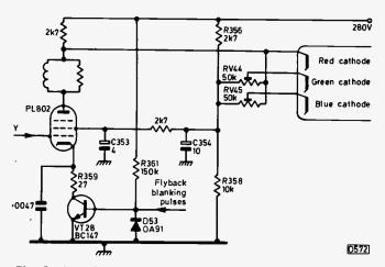
Fig. 3: A typical pentode luminance output stage. In some receivers there are preset controls in all three c.r.t. cathode circuits. The luminance signal is a.c. coupled to the PL802's control grid, and the brightness control acts here via a d.c. restorer. Beam limiting is also generally carried out at this point in hybrid colour receivers.
