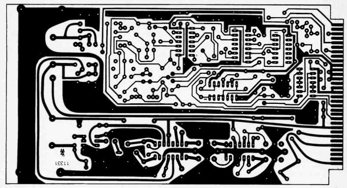
Fig. 3: Copper pattern of the new signal board. The board is available from our Readers PCB Services, reference 11331. Note that the actual size of the board is 386mm × 205mm.
