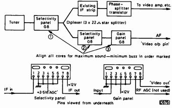
Fig. 2: Block diagram of a single-standard receiver converted for reception of French TV.
