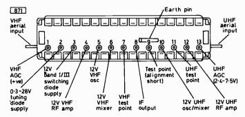
Fig. 1: ELC2000/ELC2060 u.h.f./v.h.f. varicap tuner pin connections. The output from the u.h.f. section of the tuner is coupled to the v.h.f. mixer.
