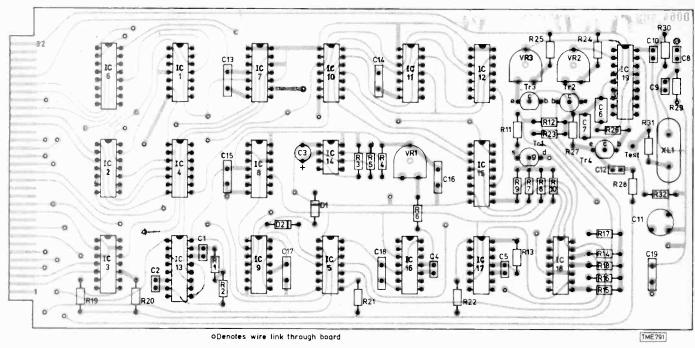
Fig. 7: Component location diagram for the options board.
