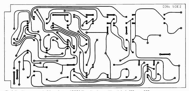
Fig. 6: Topside copper track of the options card D064. Note that the actual board size is  $438mm \times 205mm$ .
