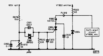
Fig. 2: The over-voltage protection circuit used in early models. On very early versions, PL919 is taken to the cathode of the mains rectifier thyristor: this gives a crowbar action, blowing the mains fuse in the event of excessive h.t. voltage.
