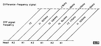
Fig. 5: The sequence of the dynamic track following signals. Read from the right, this is f1, f2, f4, f3.
