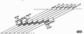
Fig. 6: For dynamic head position correction during recording, a signal is laid down during a 96µsec period while the field flyback is occurring. Recording ceases during the following 96µsec period, the head then reading the crosstalk signal from the previous track. The resultant signal initiates the servo control action.
