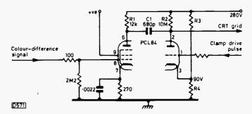
Fig. 2: A typical colour-difference output stage, with triode clamp. C1 couples the signal to the c.r.t.'s grid, with the triode setting the d.c. conditions at the grid. The black level is set by the potential divider R3/R4.
