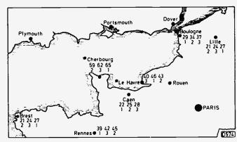
Fig. 1: French TV transmitters which can be received in the UK. Those marked with an asterisk provide a strong signal in good reception conditions only. Cherbourg, Le Havre and Boulogne have an e.r.p. of 100kW, all others an e.r.p. of 1MW. Rouen is also a 1MW transmitter, but the channels are the same as Crystal Palace. The network number is shown beneath the channel number.
