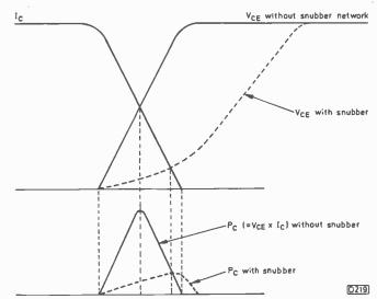
Fig. 16: Use of a snubber network to reduce the power dissipation in the chopper transistor when it switches off.
