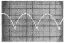
12: Connector D1, timebase board. 3V peak-to-peak.
