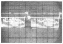
6: Connector A2, timebase board. 3V peak-to-peak.
