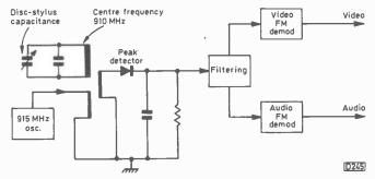
Fig. 1: Principle of the SelectaVision disc replay system.
