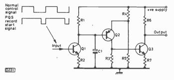
Fig. 1: Toshiba's PQS programme detector circuit.
