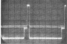
9: Connector A3, timebase board. 11V peak-to-peak.
