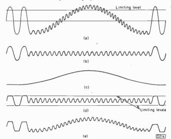
Fig. 26: Luminance signal limiting – see last month. (a) Signal with low-amplitude, high-frequency component. (b) Output from the high-pass filter. (c) Output from the low-pass filter. (d) Output from the limiter. (e) Addition of outputs (c) and (d).
