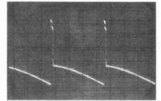
11: Connector D2, timebase board. 48V peak-to-peak.
