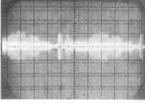
3: Pin 3 of IC3, signals board. 0.2V peak-to-peak.
