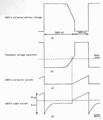
Fig. 14: Switch-mode power supply waveforms.
