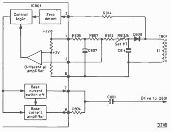
Fig. 15: Output voltage regulation.
