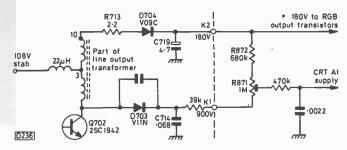
Fig. 1: Method of obtaining the 180V and 900V supplies in the GEC C2055/C2255 series. Q702 is the line output transistor.
