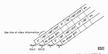
Fig. 30: The head 1 chroma signal is phase shifted by 90° line by line to avoid chroma crosstalk between adjacent tracks.
