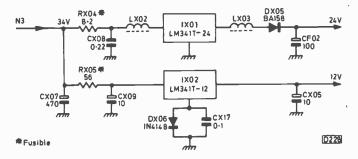
Fig. 2: The 12V and 24V regulators. In earlier versions RX05 was fed from the cathode of DX05 – RX05 is then  $39\Omega$ .
