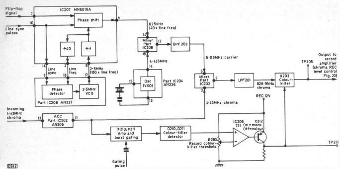
Fig. 29: Chroma signal processing arrangements on record.
