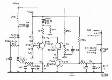
Fig. 4: The electronic trip circuit.
