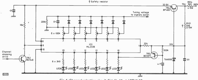
Fig. 1: Channel selection circuit, Fidelity Model CTV14R.
