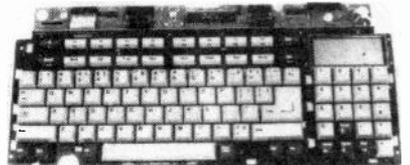
Z8852D Keyboard. Superb brand new high quality keyboard with LCD displaying 1 line of 10 characters and a further line with various symbols. 100 keys, inc separate numeric keypad. Chips on board are 2x74HC05, 80C48. LCD + driver chip are easily removed. Amazing low price - only **£10.00**
