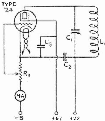
WIRING OF THE A.C. DYNATRON FREQUENCY METER
