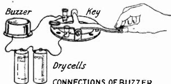
CONNECTIONS OF BUZZER
