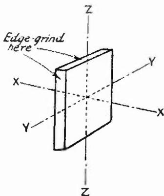
**RELATION OF THE AXES OF AN X-CUT QUARTZ PLATE**
