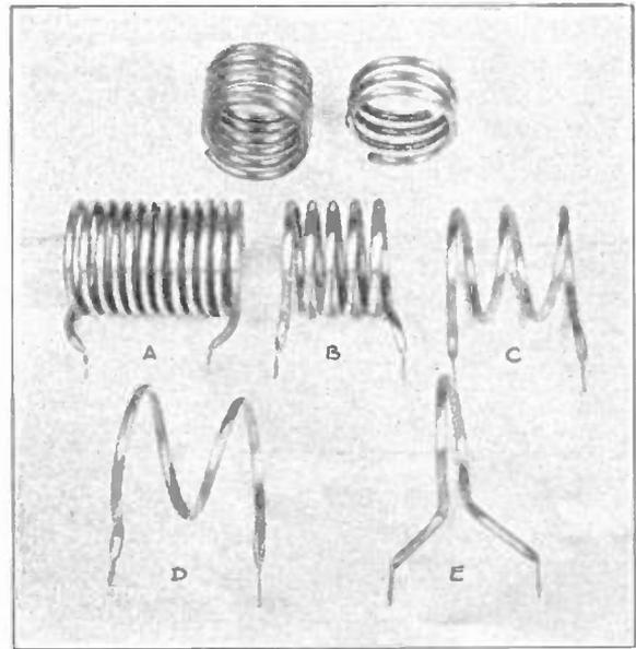
PLATE AND ANTENNA COILS FOR THE HARTLEY SET
