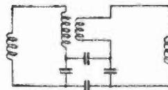
Magnetic and indirect Capacitive Coupling
