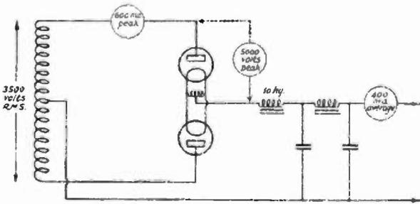
IN THIS CIRCUIT ARRANGEMENT THE FILTER INPUT IS THROUGH A CHOKE
