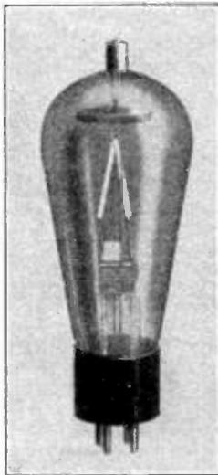
A TYPICAL HOT-CATHODE MERCURY-VAPOR RECTIFIER TUBE
