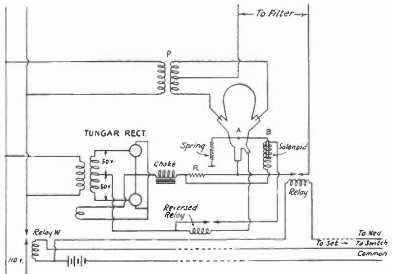
THE WIRING OF THE MERCURY-ARC INSTALLATION
