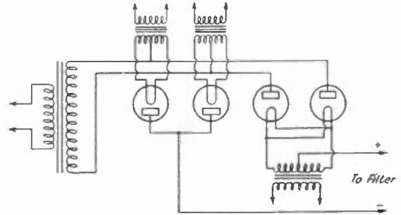
A BRIDGE RECTIFIER WITH MERCURY-VAPOR TUBES
