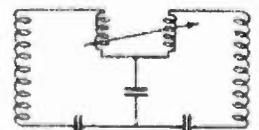
Magnetic and Direct Capacitive Coupling
