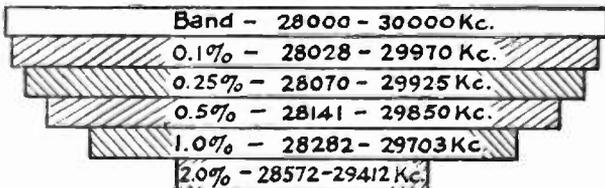
**HOW TRANSMITTER TUNING IS RESTRICTED BY ERROR IN FREQUENCY MEASUREMENT**
