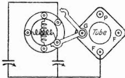
Wiring of coil and setting of switch to connect larger section of condenser across grid coil for the 7,000-K.C. band.
