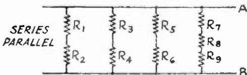
$$R_{total} = \frac{1}{\frac{1}{R_1 + R_2} + \frac{1}{R_3 + R_4} + \frac{1}{R_5 + R_6} + \frac{1}{R_7 + R_8 + R_9}}$$
