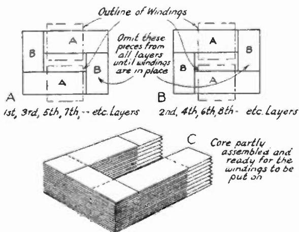
HOW TO PUT A TRANSFORMER CORE TOGETHER
