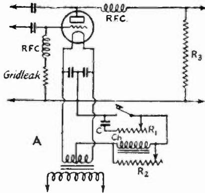
the power-supply system of the transmitter. In the former case radio-frequency choke coils connected to each side of the 110-volt line at the point where it is connected to the receiver will help. If the r.f. is getting back through the trans-
