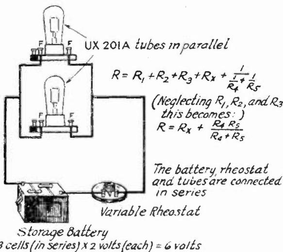
$$R = R_1 + R_2 + R_3 + R_x + \frac{1}{\frac{1}{R_4} + \frac{1}{R_5}}$$
