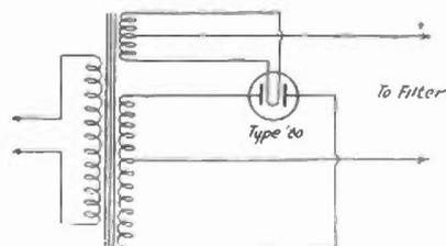
**CONNECTIONS USED WITH A TYPE '80 TUBE**
