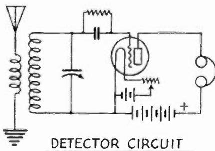
as heat. Any three-element vacuum tube can perform all three kinds of action if we use it properly.
