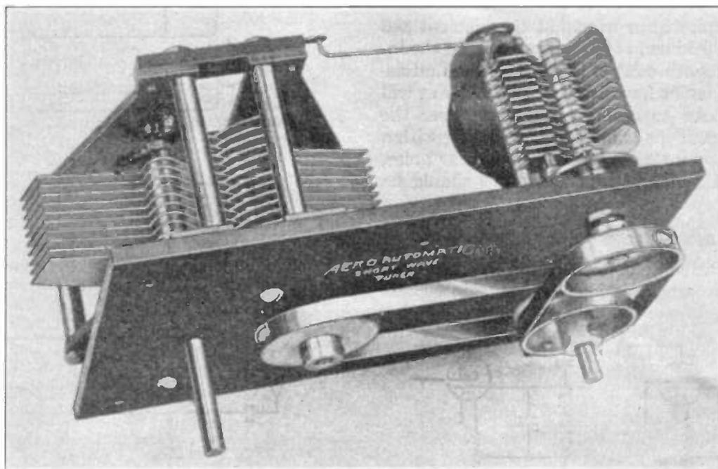
A TUNING UNIT WHICH COVERS FROM 3000 TO 15,000 KC. WITHOUT INTER-CHANGEABLE COILS
