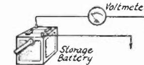
*Opens in wiring or coils are indicated by no reading on voltmeter or by no click in phones. A weak click or low voltmeter reading indicates a circuit closed through a resistance which may be a transformer winding or other part of the set.*
