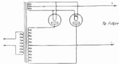
**FULL-WAVE RECTIFICATION WITH THERMIONIC OR MERCURY-VAPOR TUBES**
