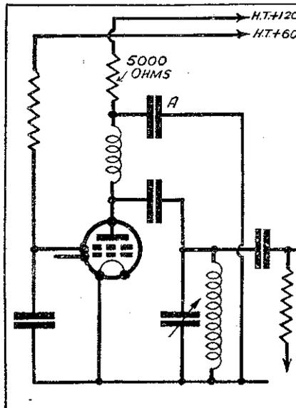
Fig. 4.—S.G. stage decoupled.
