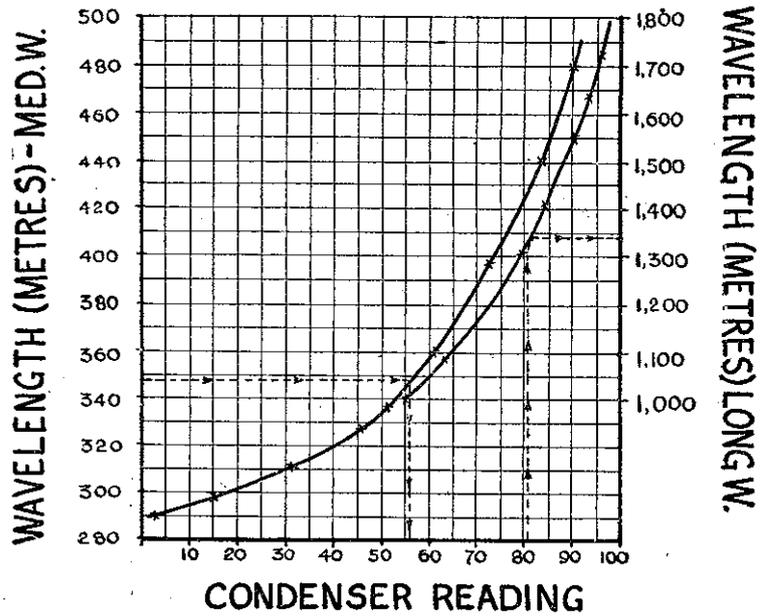
Fig. 5.—How to draw a calibration chart.
