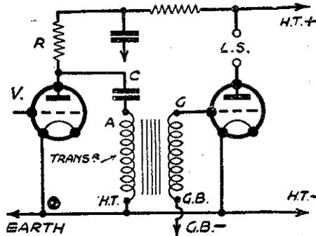
Fig. 2.—The method of parallel-feeding a transformer.
