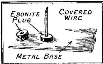
Ebonite plugs for protecting leads where they pass through the chassis.
