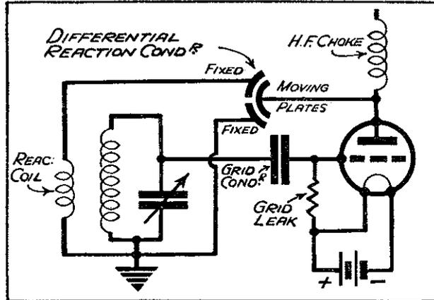
The complete detector circuit, showing the method of joining up the reaction condenser and coils.
