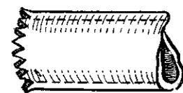
Fig. 9.—The cutting end of a wall drill.
