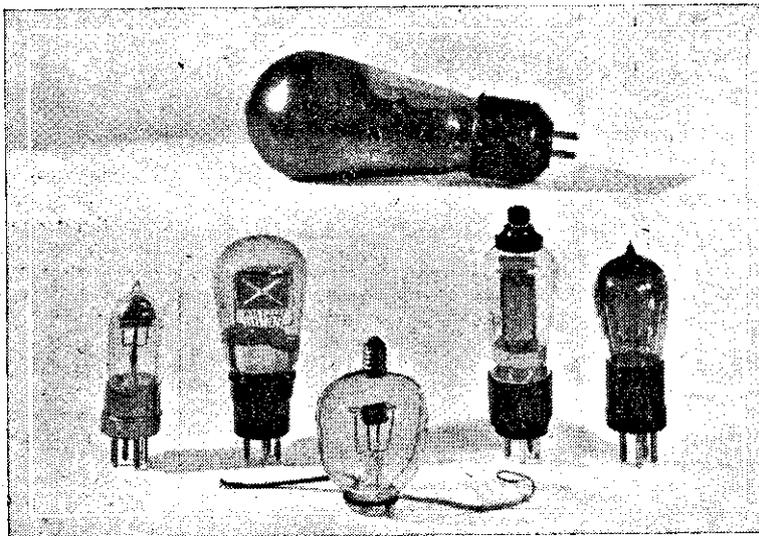
Fig. 2.—A group of Cossor valves indicating various stages in development. Top: Super-power valve of 60-Watt dissipation. Bottom row (left to right): (1) 1921—6 power valve, Stentor class. (2)—Modern pentode. (3)—1916 valve of peculiar construction. (4)—Modern mains S.G. valve (5) 1923—.3 amp. kalenised filament.
