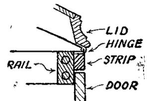
Fig. 16.—How the lid is hinged.
