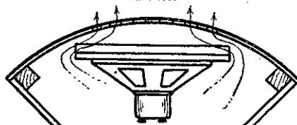
Fig. 3.—Plan of shelf of corner cabinet, showing how sound waves from back of speaker pass round the baffle.
