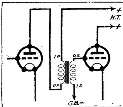
Fig. 2a.—Transformer primary directly in anode circuit.
