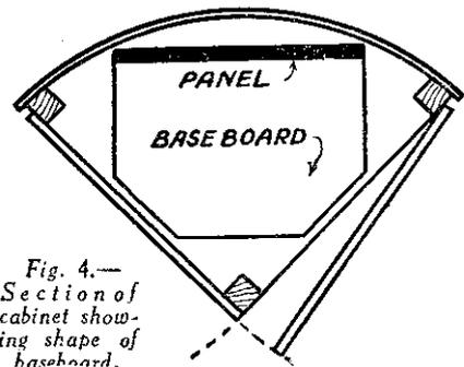
Fig. 4.—Section of cabinet showing shape of baseboard.
