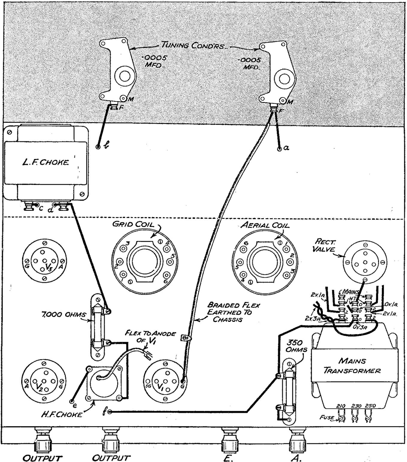
Above—Chassis Wiring Diagram of the Mains Express Three.
