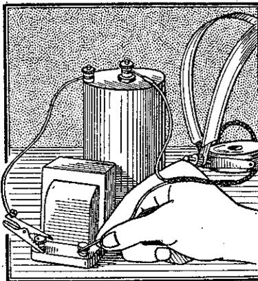
A simple method of testing with phones and a dry battery.
