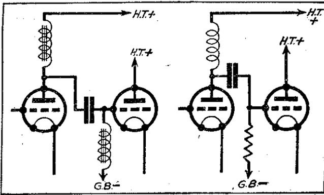
Fig. 3.—Two forms of choke coupling.
