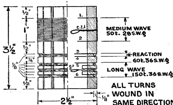
Fig. 1.—Constructional details of a tuner made on an eight-ribbed 2½in. diameter ebonite former.
