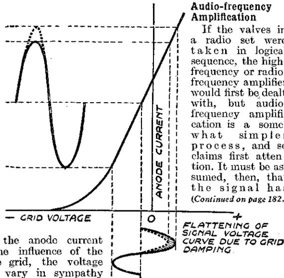
Indicating the result of under-biasing an amplifying valve. The grid becomes positive with respect to the filament during a part of the alternate half cycles. Grid current flows and reduces the effective signal, as shown by the shaded arcs, while the effect on the anode current is shown at the top left of the diagram.
