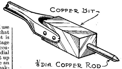
How to fit a small bit to your soldering iron.
