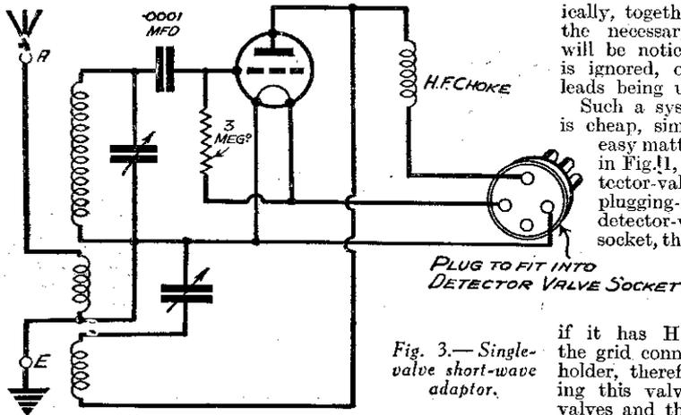
Fig. 3.—Single-valve short-wave adaptor.
