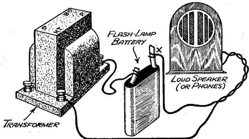
Fig. 2.—The way to test a transformer winding.
