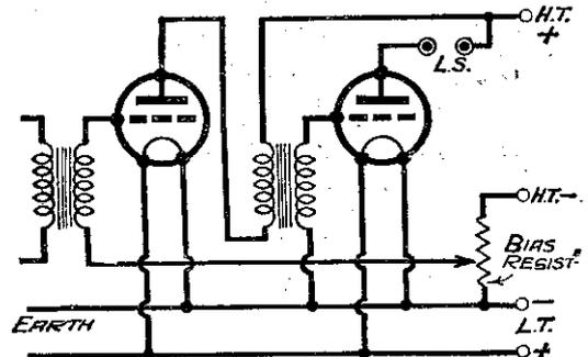
Fig. 6.—A common resistance connected up to provide bias for two battery-heated valves.
