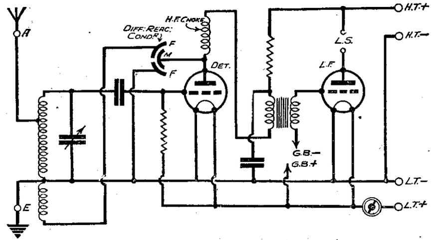
Fig. 2.—Circuit of a two-valve receiver.
