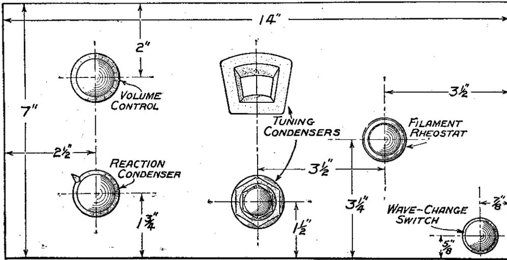
Template for marking position of holes on the Camco Ambassador Cabinet front.
