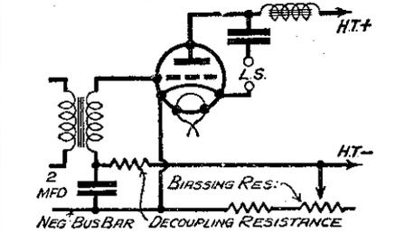
Fig. 3.—An alternative arrangement of Fig. 2, in which the cathode is maintained at the normal negative potential.
