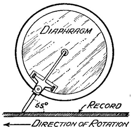
The correct angle for a needle—with either ordinary acoustic sound-box or electric pick-up.
