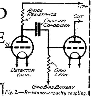
Fig. 2.—Resistance-capacity coupling.
