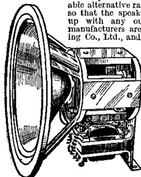
A permanent magnet moving-coil loud-speaker with transformer incorporated.
