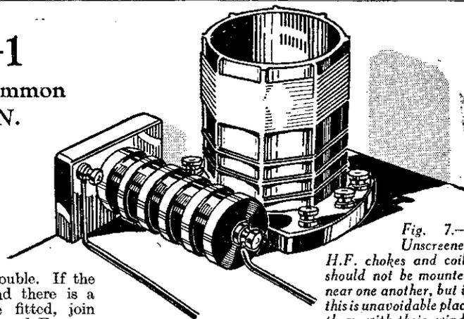
Fig. 7.—Unshielded H.F. chokes and coils should not be mounted near one another, but if this is unavoidable place them with their windings at right angles to prevent interaction and H.F. howling.
