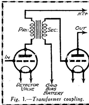
Fig. 1.—Transformer coupling.
