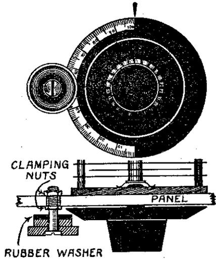
The above sketch shows a simple method of attaching a slow-motion device to the dial of a condenser.
