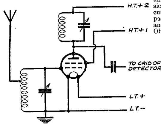
A circuit diagram of a screen-grid-H.F. stage.
