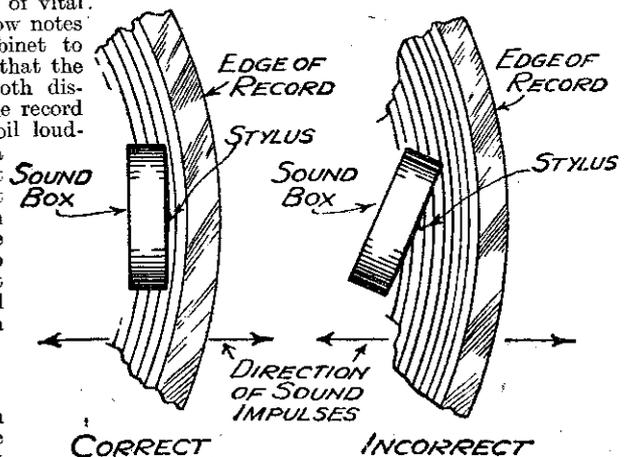
The "tracking" angle—which was fully explained in a recent issue. Note how the sound-box or pick-up must be parallel with the sound grooves.
