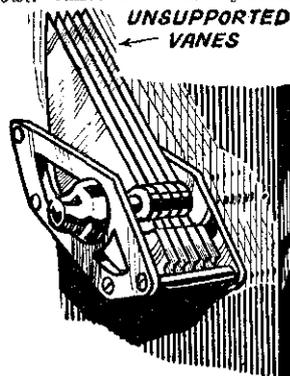
Fig. 2.—Vibrating condenser sponge rubber pads may cause a microphonic howl.
