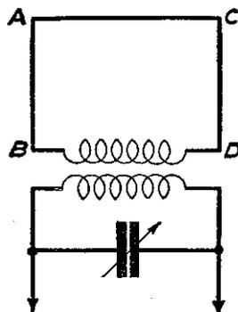
Fig. 3.—The frame aerial with its small coil coupled to the main tuning circuit.
