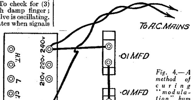
Fig. 4.—A method of curing "modulation" hum
