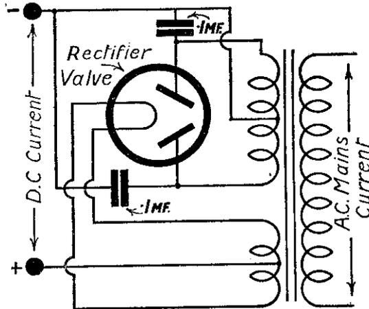
Fig. 1.—Rectifier hum can be cured by connecting two .1 mfd. fixed condensers between the two rectifier anodes and high-tension negative.
