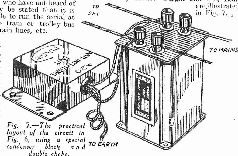
Fig. 7.—The practical layout of the circuit in Fig. 6, using a special condenser block and double choke.
