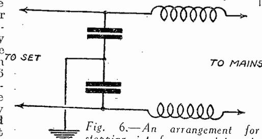
Fig. 6.—An arrangement for stopping interference arriving via the mains
