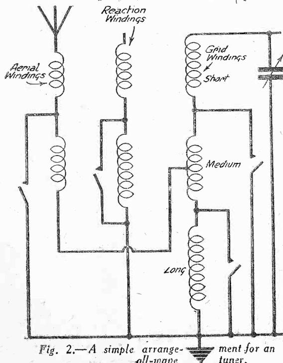
Fig. 2.—A simple arrangement for an all-wave tuner.
