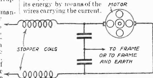
Fig. 3.—Interference suppressor which may be fitted to various domestic appliances.
