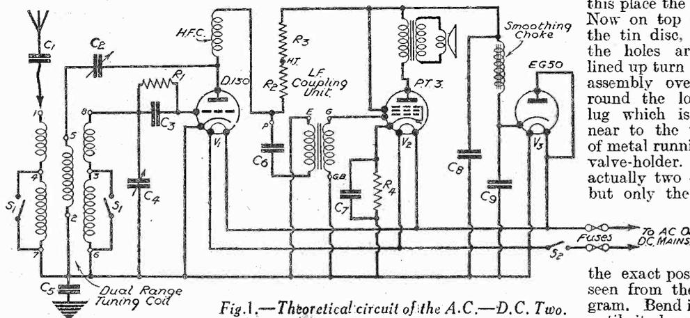
Fig. 1.—Theoretical circuit of the A.C.—D.C. T.W.O.
