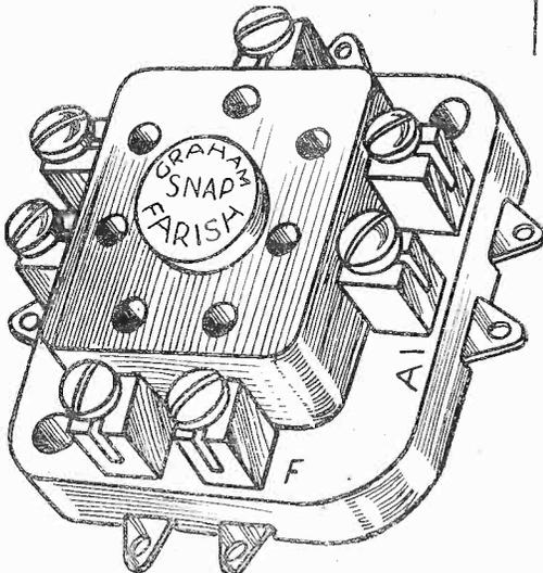
A new type of valveholder, manufactured by Graham Farish. The new idea in terminals enables a number of wires to be accommodated without the trouble of the wires becoming loose owing to the nut untwisting the loop. The wire ends are accommodated in the slots in the terminals.
