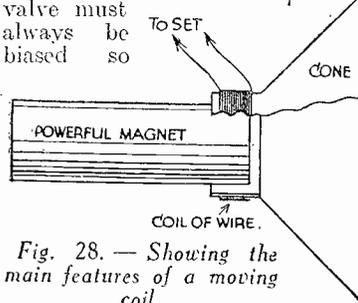
Fig. 28.—Showing the main features of a moving coil.
