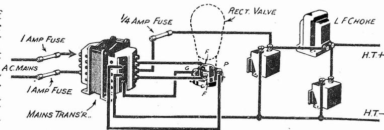
Fig. 15.—A rectifier unit showing suggested position of fuses:
