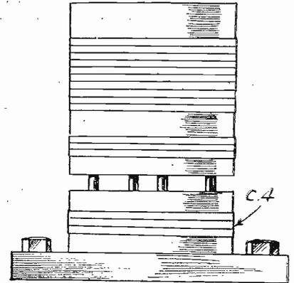
Fig. 4.—Mounting the coupling coil on the same base as the tuning coil.
