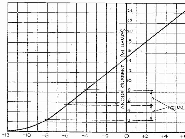
Fig. 25.—For distortionless reproduction the valve must be worked on the lower straight part of its characteristic.
