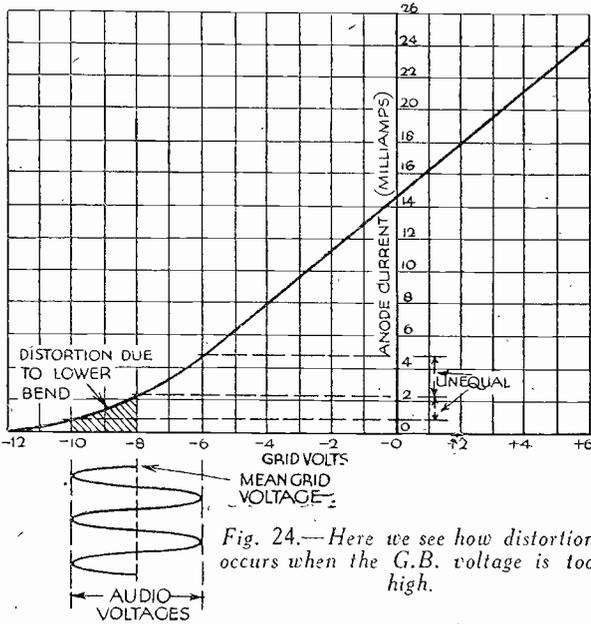
Fig. 24.—Here we see how distortion occurs when the G.B. voltage is too high.
