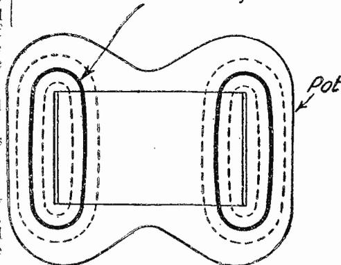
Fig. 2.—This diagram shows the arrangement of the magnetic field round a "potted" coil.
