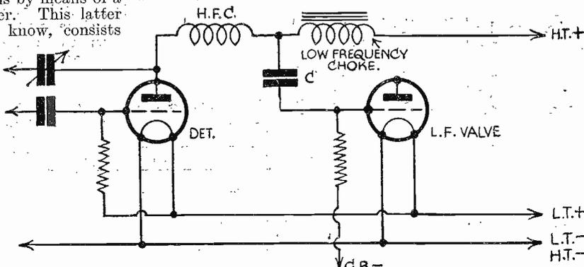
Fig. 21.—Choke-capacity L.F. coupling.
