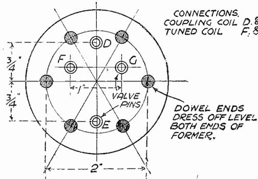
Fig. 1.—Details of coil-former and windings.
