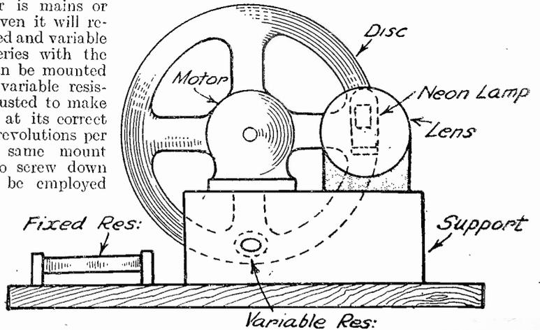
Fig. 2.—A rough layout of the disc model television apparatus.
