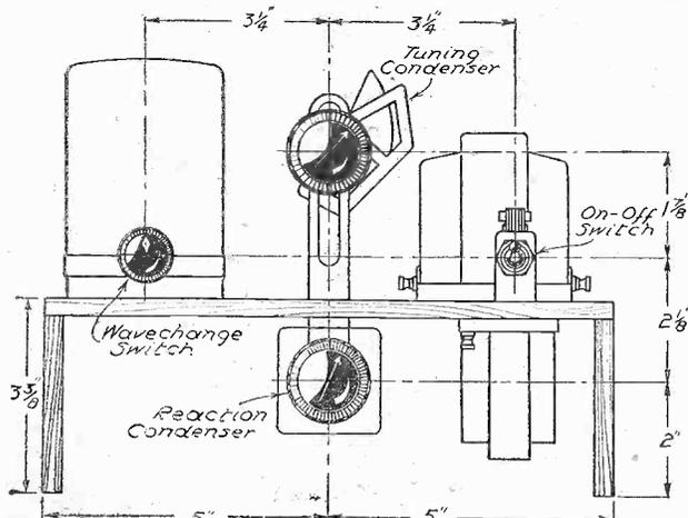
Fig. 2.—Disposition of controls.
