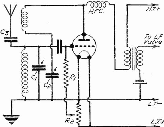
Fig. 1.—A simple reaction arrangement.
