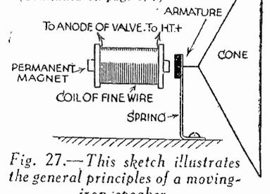
Fig. 27.—This sketch illustrates the general principles of a moving-iron speaker.
