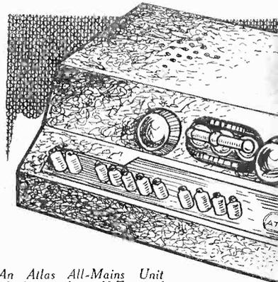
An Atlas All-Mains Unit which supplies H.T. and G.B. voltages as well as possessing a Trickle Charger to keep the L.T. battery in trim. This model costs £6 10s.
