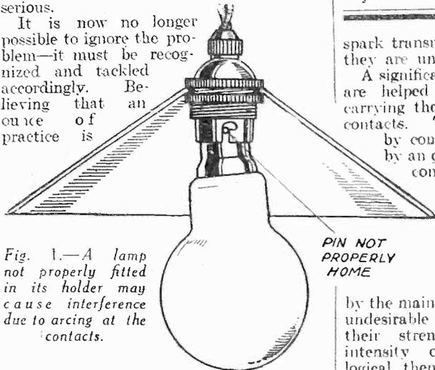
Fig. 1.—A lamp not properly fitted in its holder may cause interference due to arcing at the contacts.
