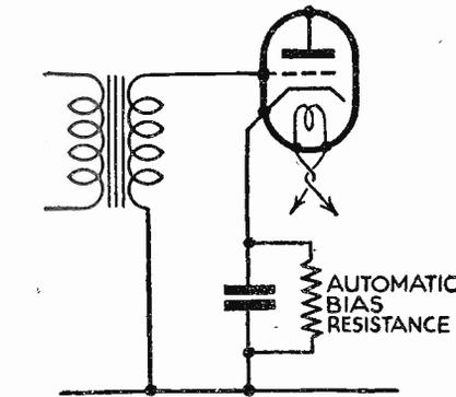
Fig. 2.— The circuit of an indirectly-heated power valve with automatic grid bias.
