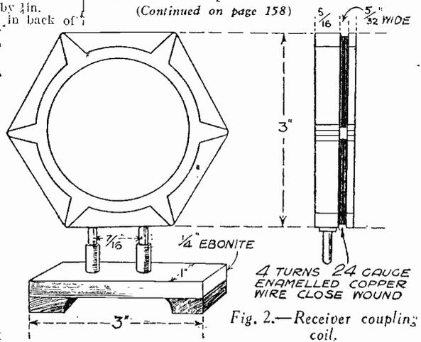
Fig. 2.—Receiver coupling coil.
