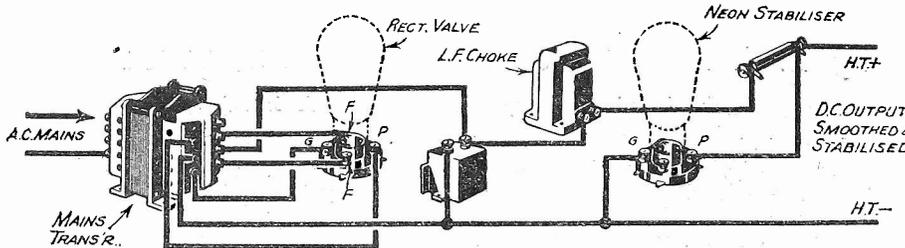
Fig. 14.—Adding a neon tube voltage stabilizer for an eliminator supplying a Class B valve.
