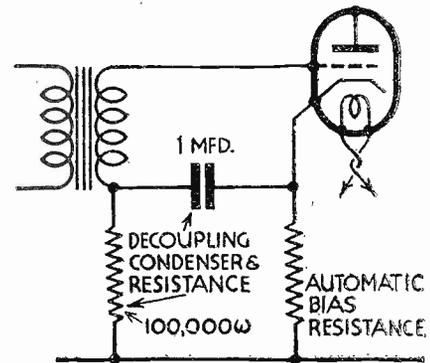
Fig. 3.— Complete decoupling has been added in this modification of the Fig. 2 arrangement
