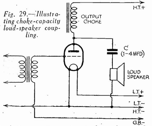
Fig. 29.—Illustrating choke-capacity loud-speaker coupling.
