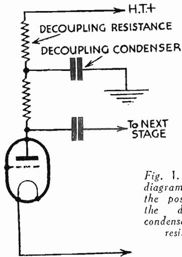
Fig. 1.— This diagram shows the positions of the decoupling condenser and resistance.
