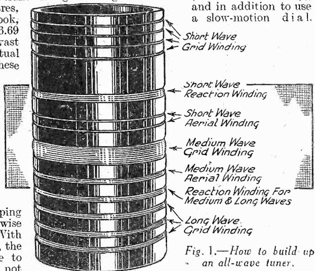
Fig. 1.—How to build up an all-wave tuner.
