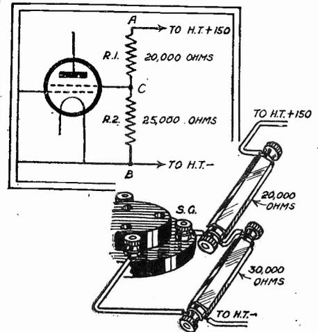
Fig. 9.—Potentiometer method of obtaining screening grid volts.
