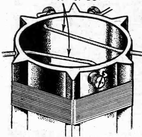
*Method of shortening leads to a tuning coil.* coil former in several places at the upper and lower edges; this procedure enabled me to pass any connections to the more remote coil terminals through the interior of the coil, and considerably shorten the long leads. There is absolutely no tendency
