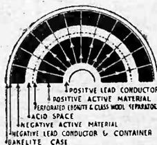
Alongside is a half section of the new cell, in plan. In the old type, current largely concentrated round the good-conducting but inert grids, causing uneven charging. Now plates are gone — and circular formation forces the current to pass through every particle of paste in its passage from central positive to outer negative. Absence of grids also reduces waste weight and space. What a sensible Christmas present!
