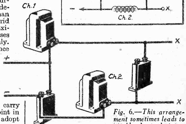
Fig. 6.—This arrangement sometimes leads to trouble, due to the interaction of the two chokes. In addition, the two inductances are in parallel.
