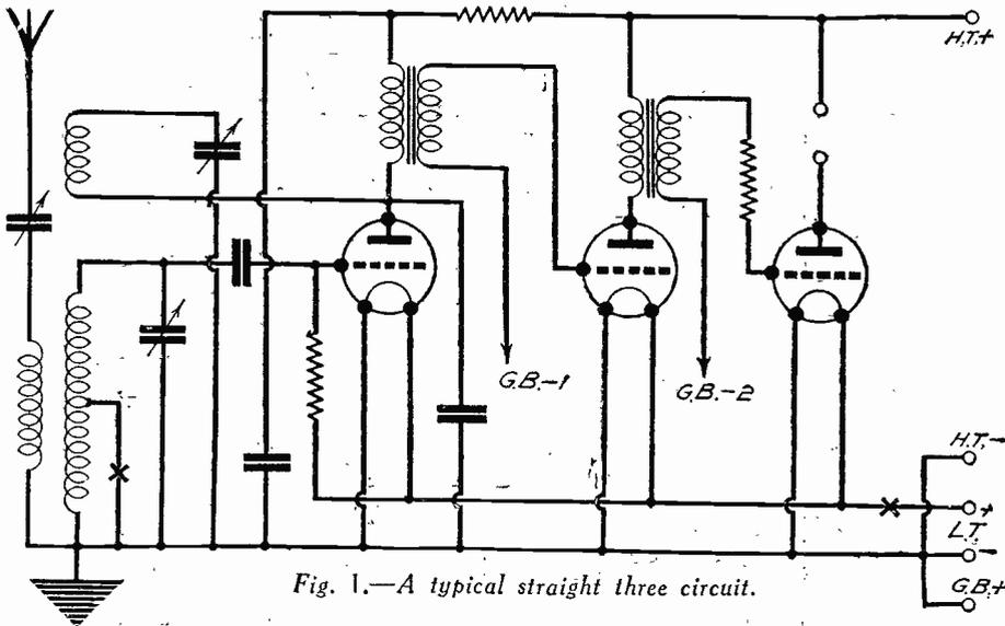
Fig. 1.—A typical straight three circuit.
