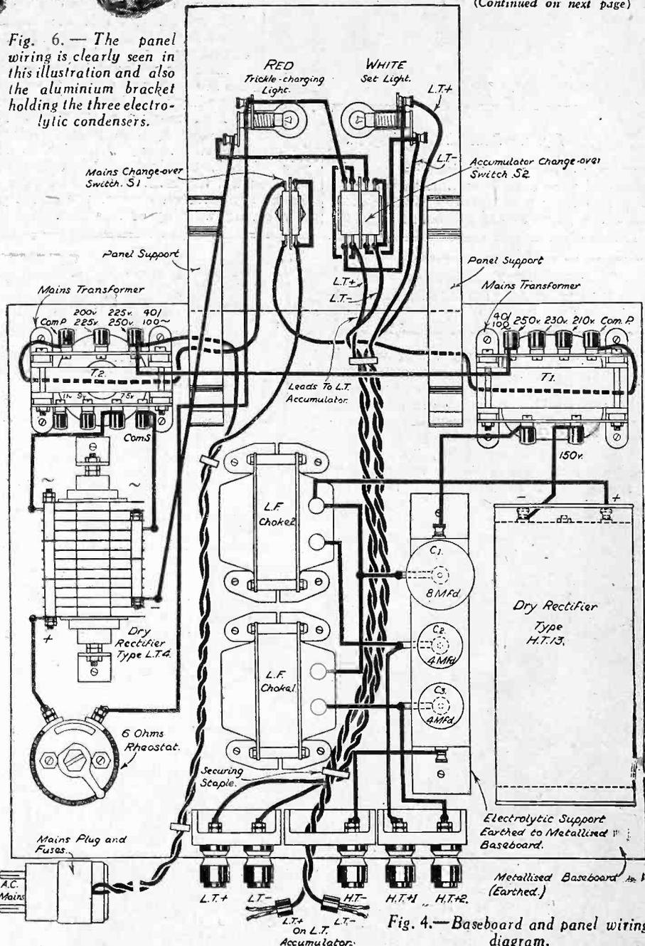
Fig. 4.— Baseboard and panel wiring diagram.
