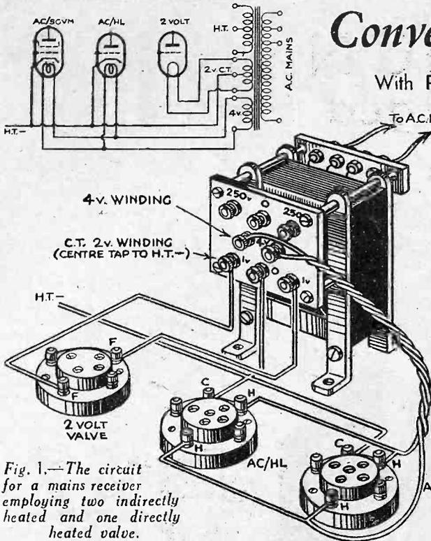
Fig. 1.—The circuit for a mains receiver employing two indirectly heated and one directly heated valve.
