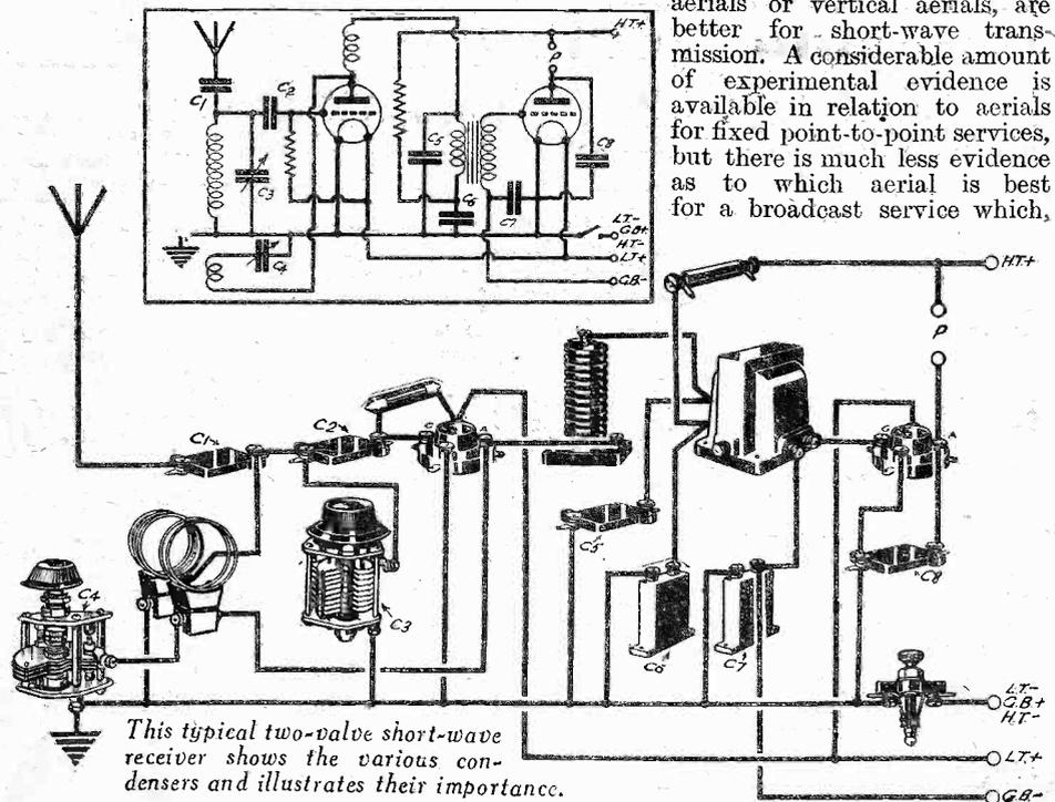
This typical two-valve short-wave receiver shows the various condensers and illustrates their importance.
