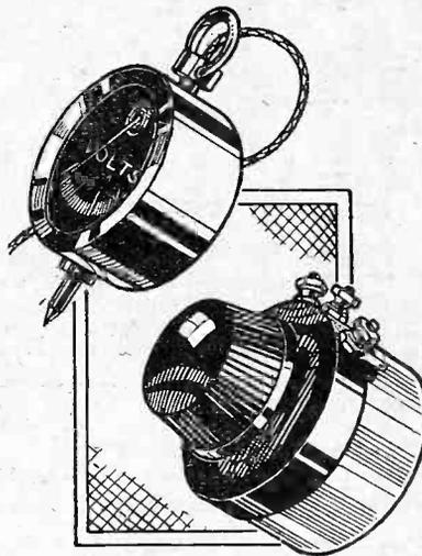
Fig. 3.—A voltmeter is a true potentiometer. The volume control on the right is, strictly speaking, a "potential divider."
