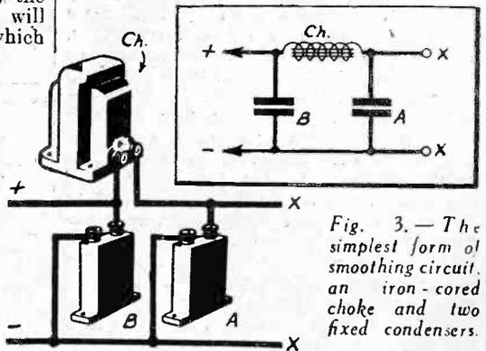
Fig. 3.—The simplest form of smoothing circuit, an iron-cored choke and two fixed condensers.
