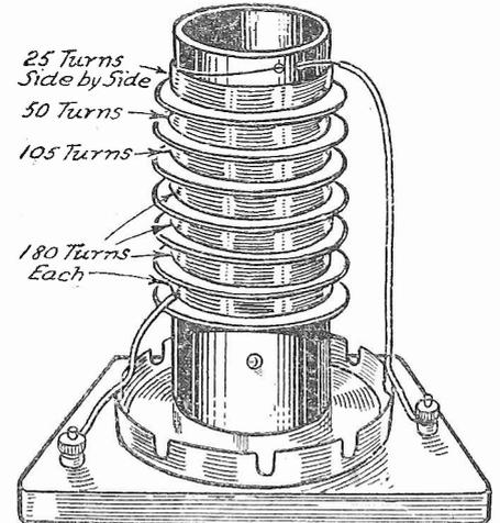
Fig. 6.—Details of an excellent all-wave or universal H.F. choke.
