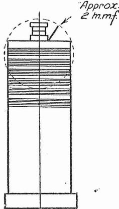
Fig. 5.— Illustrating the method of estimating the capacity of a choke.
