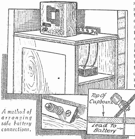
A method of arranging safe battery connections.
