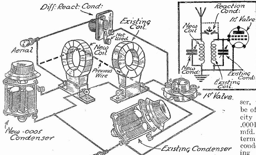
Fig. 1.—This sketch shows a simple means of converting the aerial tuning condenser of a receiver to a simple band-pass arrangement.
