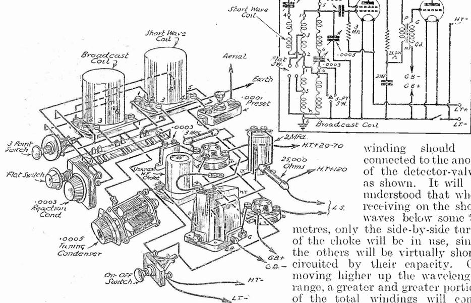
Fig. 5.—A useful all-wave two-valve circuit using two of the coils described.
