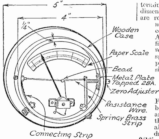
Fig. 1.—Sketch of the finished hot-wire meter described: dimensions are only approximate.
