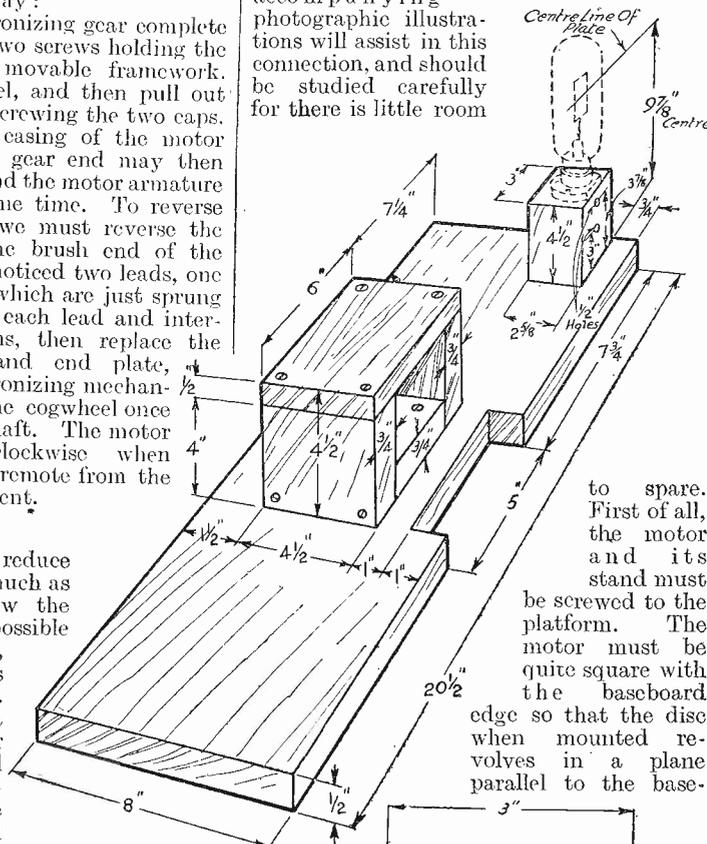
Fig. 9.—The wooden base and motor support.
