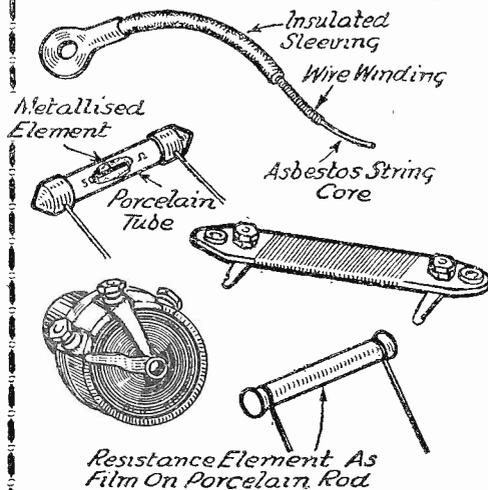
Fig. 2.—Various types of resistances are shown in the above sketch; some of these are sectionalized to indicate the form of construction.
