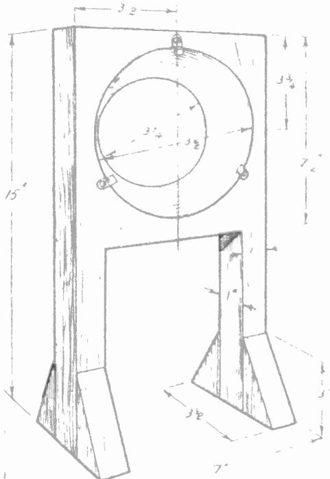
Fig. 10 - The lens mount. Note the bevelled hole.
