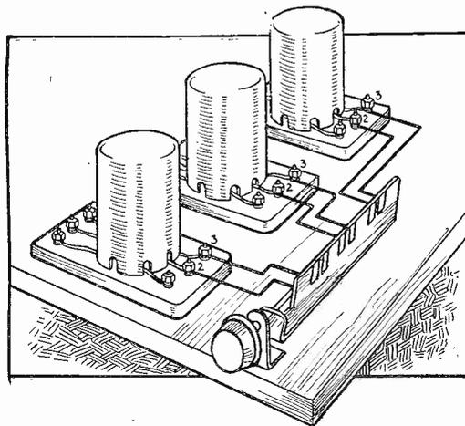
Fig. 3.—A convenient method of mounting the flat wave-change switch beside a set of coils.
