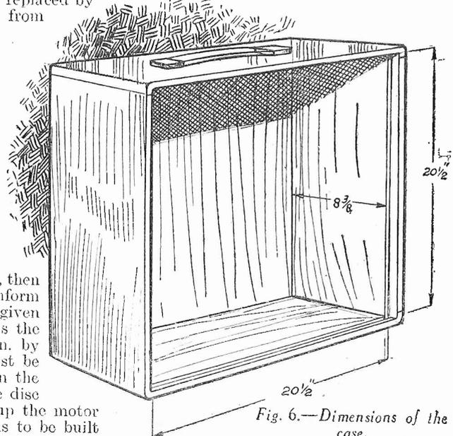
Fig. 6.—Dimensions of the case.
