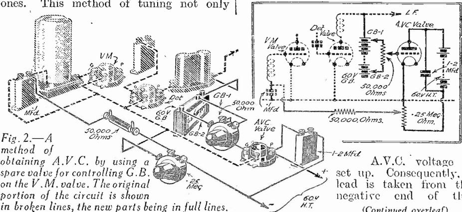
Fig. 2.—A method of obtaining A.V.C. by using a spare valve for controlling G.B. on the V.M. valve. The original portion of the circuit is shown in broken lines, the new parts being in full lines.
