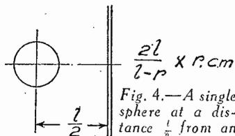
Fig. 4.— A single sphere at a distance *l/2* from an earthed boundary wall.
