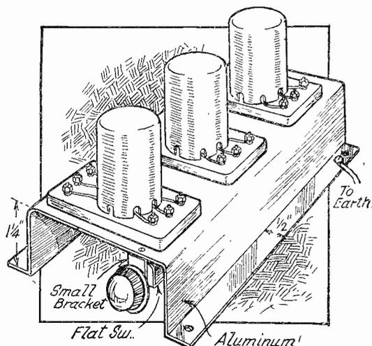
Fig. 4.—A neat way of building up a complete coil and switch assembly.
