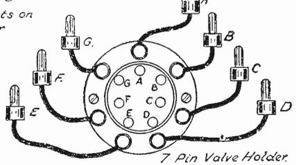
The connection for an additional valve-holder for testing Multi-pin valves on the Six-Sixty and similar test sets.
