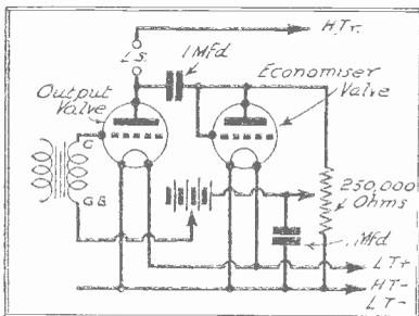
Fig. 3.—A good method of reducing the H.T. current consumption of the output valve by using an additional valve as an "economizer."
