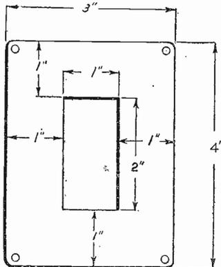
Fig. 7.—The aluminium mask should be cut to these dimensions.
