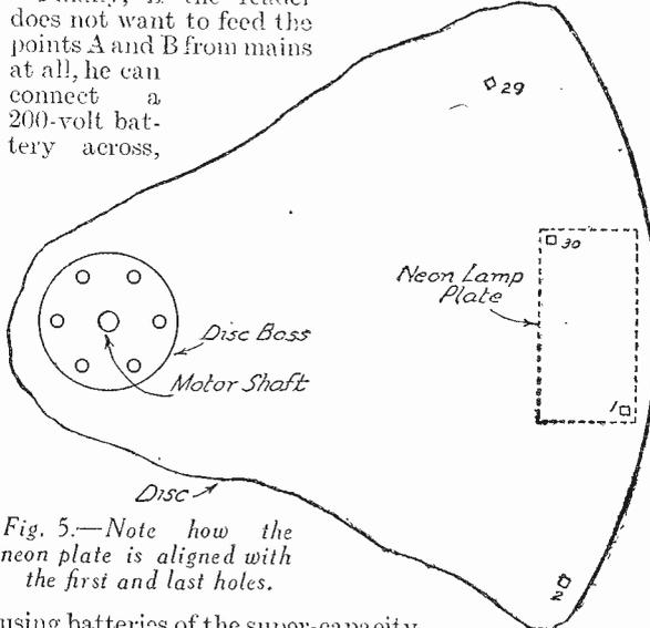
Fig. 5.—Note how the neon plate is aligned with the first and last holes.
