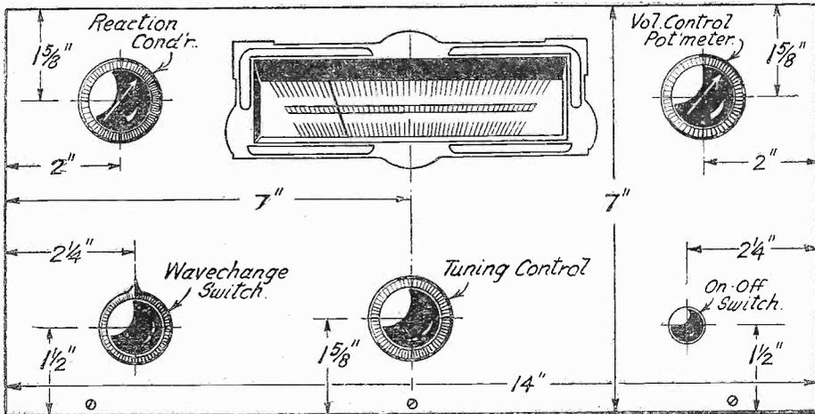
Fig. 2.—Front of panel layout.
