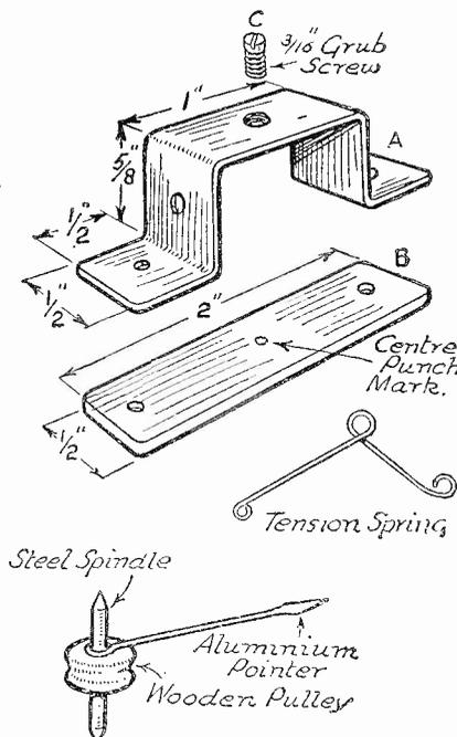
Fig. 2.—The above sketches give all constructional details for the more important parts of the meter described.
