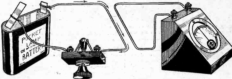
Fig. 1.—Simple experiment to demonstrate the principle of induction, on which the working of a transformer is dependent.
