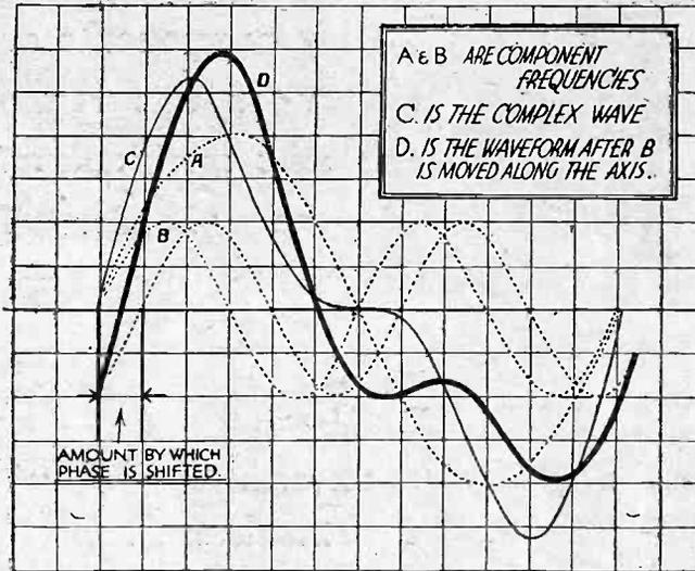
Fig. 1.—A graph illustrating the alteration in shape of signal waveforms.
