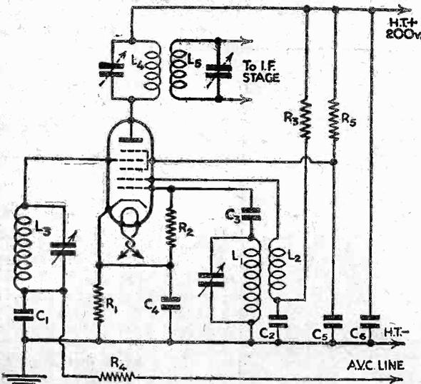
Fig. 3.—The circuit of the pentagrid frequency changer.  $R_5$  is not mentioned in the text as it is merely to drop the 200v. to a lower value for the screen grids.
