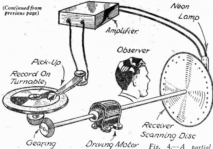
Fig. 4.—A partial duplication of Fig. 1 is undertaken when reproducing the recorded image.
