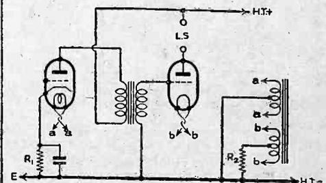
Fig. 9.—When a mains transformer is used which has separate heater windings for the directly-heated and indirectly-heated valves, grid decoupling is generally quite unnecessary, and a circuit such as that shown above can be employed.
