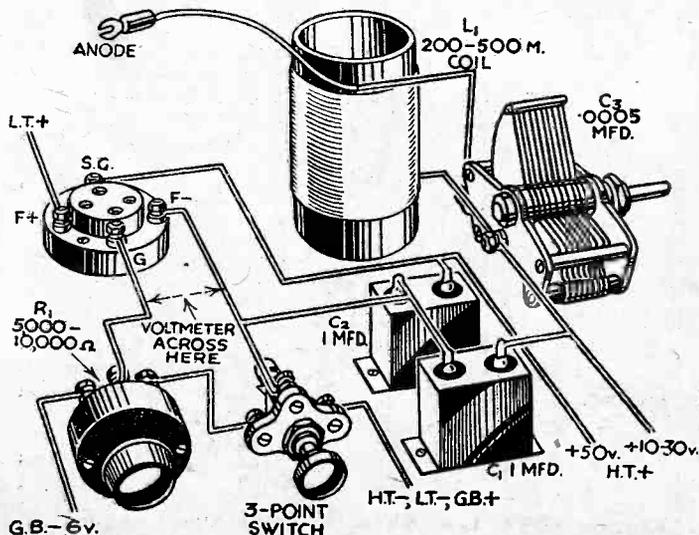
Fig. 3.—A practical circuit of a complete dynatron oscillator which is described in the text.
