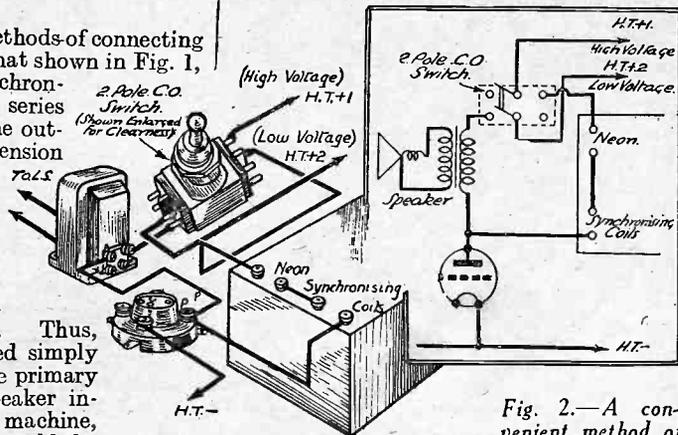
Fig. 2.—A convenient method of switching in a battery set using a single output valve, and where the apparatus is series fed.
