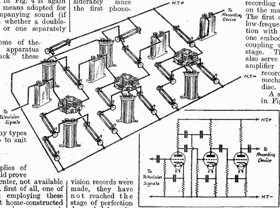
Fig 7.—The form of R.C. coupled amplifier suggested for recording and playing.
