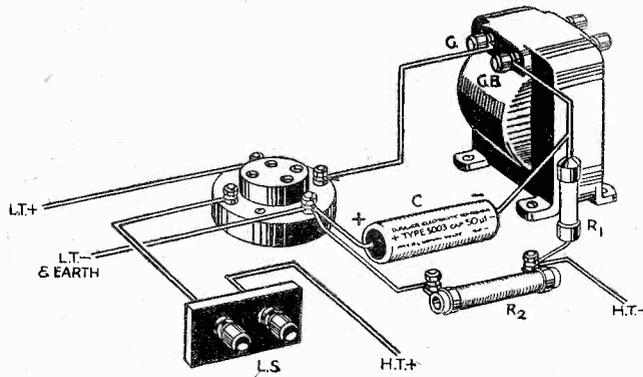
Fig. 3.—G.B. and decoupling resistances in a battery-operated output stage. R.1 is for decoupling and works in conjunction with the electrolytic condenser C.
