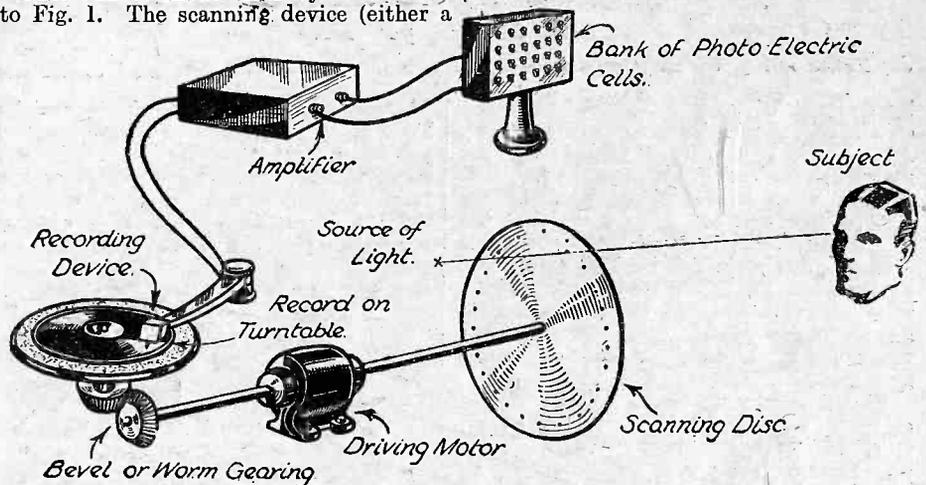
Fig. 1.—Pictorially illustrating how a record of a television transmission can be made in the studio.
