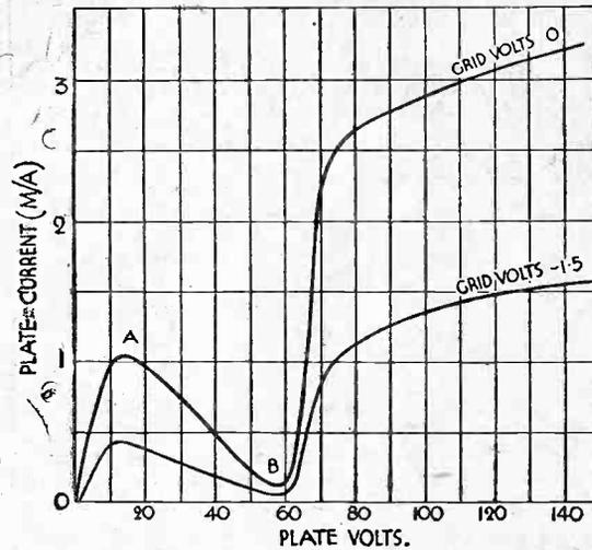
Fig. 2.—Plate volts-plate current curves for an S.G. valve.
