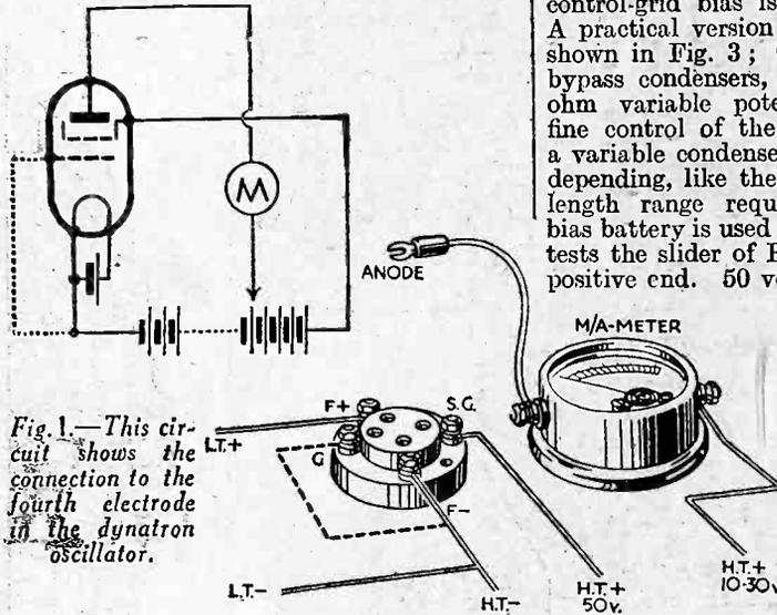
Fig. 1.—This circuit shows the connection to the fourth electrode in the dynatron oscillator.
