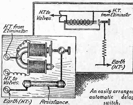
An easily arranged automatic delay switch.
