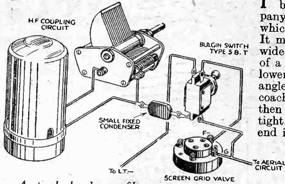
A simple band-pass filter arrangement.
