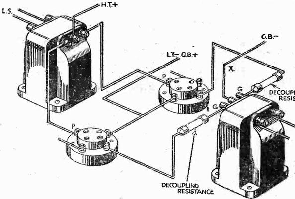
Fig. 1.—Showing how grid decoupling resistances are connected in the case of a battery-operated push-pull amplifier.
