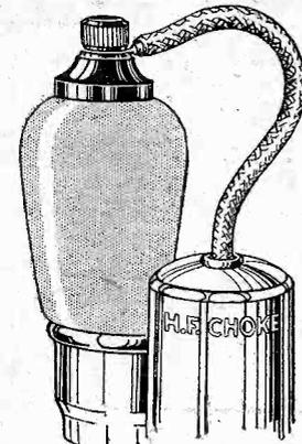
Fig. 6.—Using a screened wire for connection to the anode cap of an S.G. valve.
