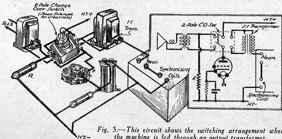
Fig. 3.—This circuit shows the switching arrangement when the machine is fed through an output transformer.
