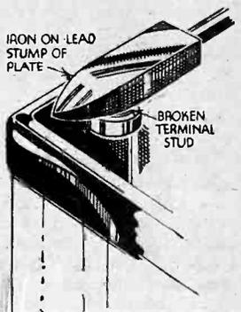
Method of removing broken terminals from accumulators.
