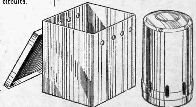
Fig. 4.—The screening box and "can."
