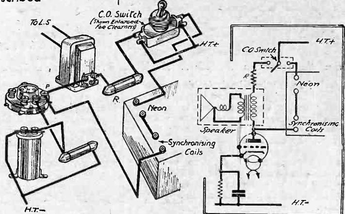
Fig. 1.—The method of switching from "sound" to "vision" when the apparatus is wired in series with the anode of the output valve.
