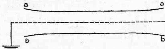
Fig. 1.—Showing simple electrostatic screening.
