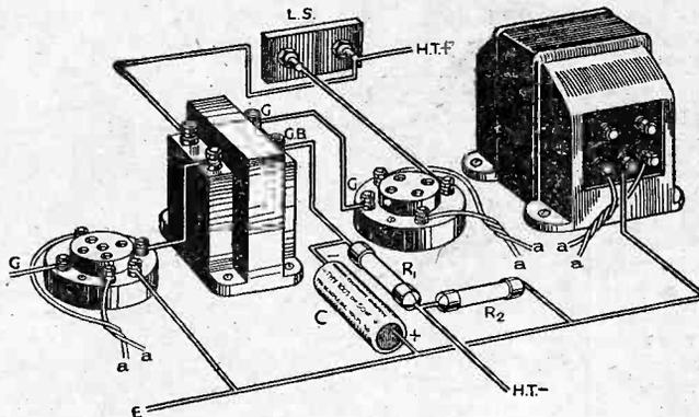
Fig. 8.—A good method of biasing a directly-heated valve which is used along with other indirectly-heated valves and whose cathode (or filament) is heated from the same source.
