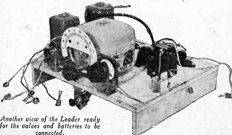
Another view of the Leader ready for the valves and batteries to be connected.
