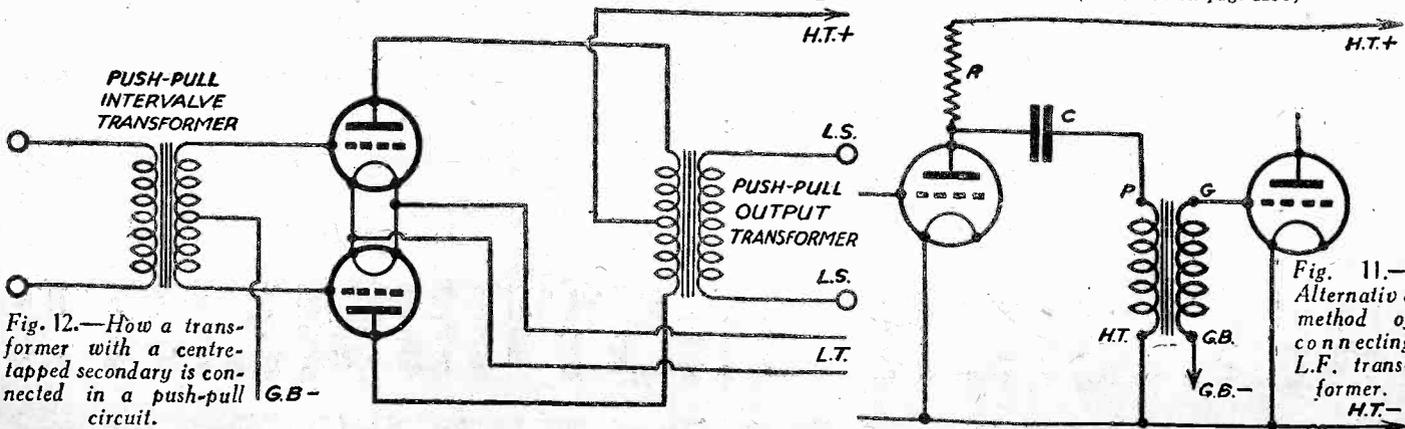
Fig. 12.—How a transformer with a centre-tapped secondary is connected in a push-pull circuit.
