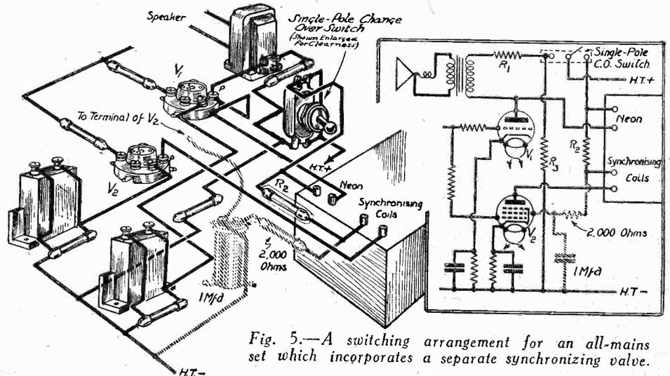
Fig. 5.—A switching arrangement for an all-mains set which incorporates a separate synchronizing valve.
