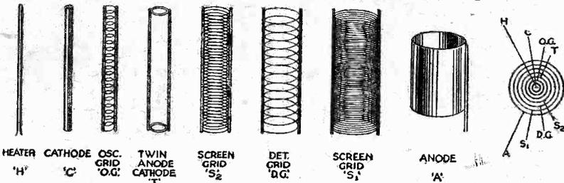
Fig. 2.—Showing the eight elements of the pentagrid valve. There are five grids in all. Note particularly the open structures of the grid marked "T."
