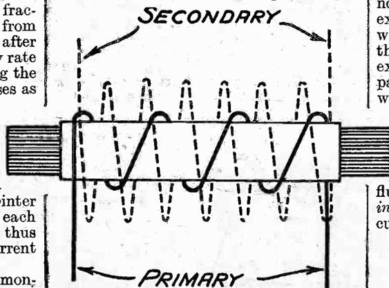
Fig. 6.—A simple transformer made of two coils of wire.
