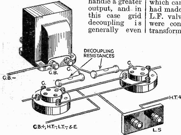
Fig. 2.—Grid decoupling resistances are very desirable when two valves are wired in parallel.
