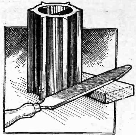
A method of slotting ribbed coil formers.
