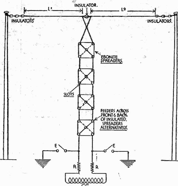
Fig. 5.—Transposed or horizontal doublet aerial.  $E$  = earthing switches.  $CC$  = coupling coil.  $RR$  = 600 ohm resistances.  $L^1, L^2$  = 40 ft. aeriels.
