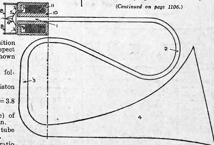
Fig. 3.—1 is a duct, leading to 2, Acoustic tube, leading to 3, Taper passage, communicating with 4, Final flare, or horn. 5, Conical diaphragm or piston. 6, Piston extension. 7 and 8 are Ligatures forming centring means. 9, Field gap with moving coil within. 10, Electro magnet (core). 11, Electro magnet winding.
