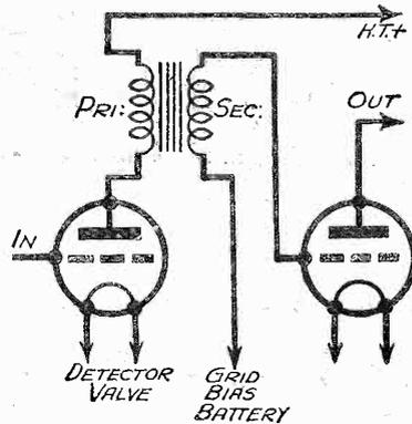
Fig. 10.—The commonest manner of connecting an intervalve transformer.
