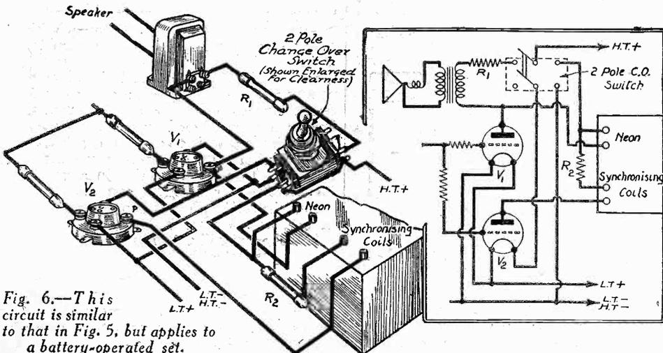
Fig. 6.—This circuit is similar to that in Fig. 5, but applies to a battery-operated set.
