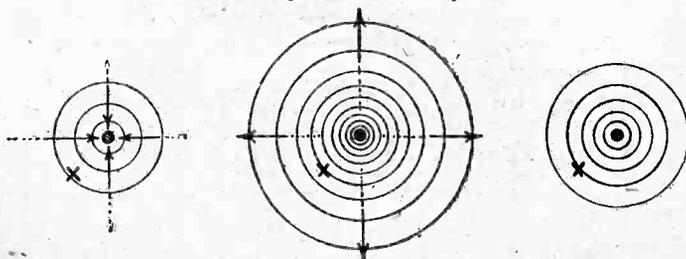
Figs. 2, 3 and 4.—Diagrams showing the lines of force round a wire carrying an electric current.
