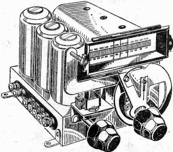
Fig. 5.—An example of a completely screened modern tuning pack.
