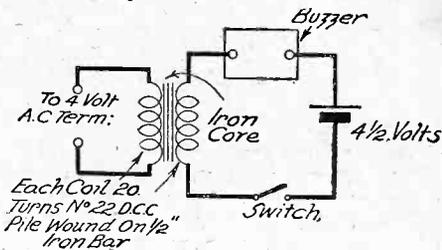
Fig. 5.—Method of using a buzzer to provide oscillations.
