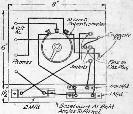
Fig. 2.—Sketch plan of lay-out and wiring diagram.
