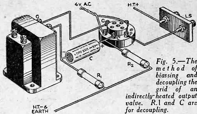
Fig. 5.—The method of biasing and decoupling the grid of an indirectly-heated output valve. R.1 and C are for decoupling.
