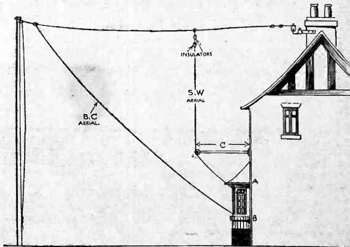
Fig. 3.—A dual aerial, A=S.W. aerial: lead-in at top right-hand side of window. B=B.C. aerial: lead-in at bottom left-hand side of window. C=2ft. minimum.
