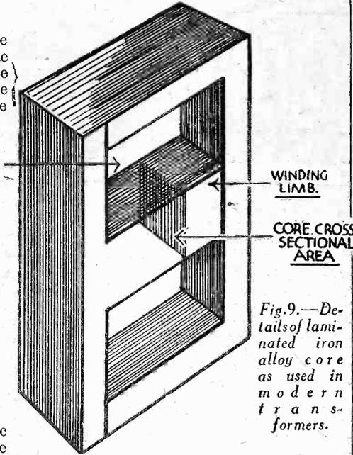
Fig. 9.—Details of laminated iron alloy core as used in modern transformers.
