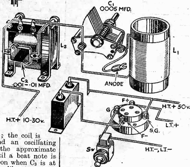
Fig. 4.—By using the circuit shown above, where an iron-core choke is connected in series with a tuned H.F. circuit, the oscillator will oscillate at both high and low frequencies.
