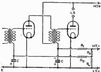
Fig. 4.—This shows grid-bias decoupling arrangements when two battery-operated L.F. valves are automatically biased.
