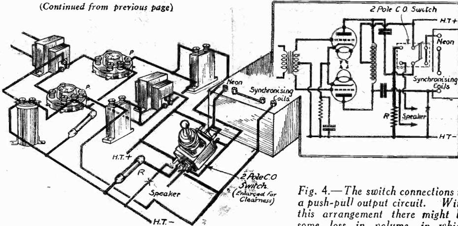
Fig. 4.—The switch connections in a push-pull output circuit. With this arrangement there might be some loss in volume, in which
