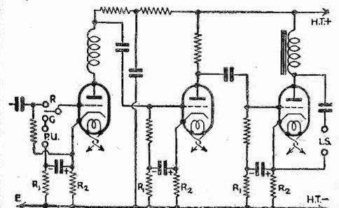
Fig. 6.—Skeleton circuit of the detector and two L.F. stages of a mains receiver where every grid is effectively decoupled.
