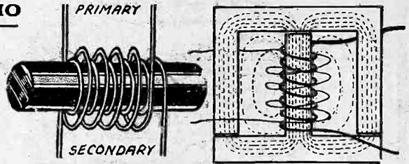
Figs. 7 and 8.—Two forms of iron core. Left, a simple iron rod; right, a core which completely surrounds the coils of the transformer.
