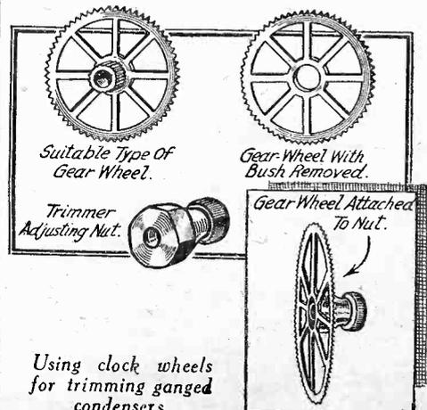
Using clock wheels for trimming ganged condensers.
