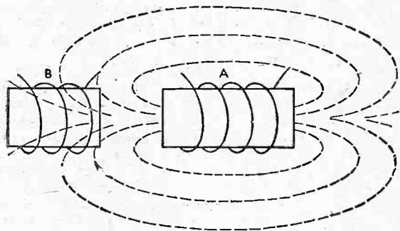
Fig. 2.—Magnetic field leakage between A and B.
