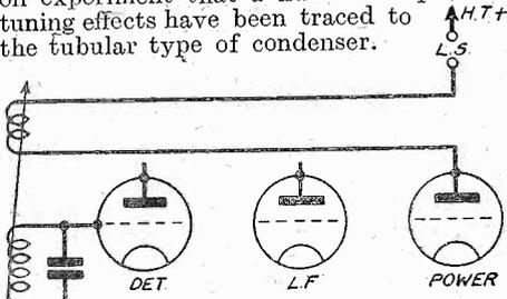
Fig. 6.—A simple method of testing the efficiency of the H.F. arrangements.
