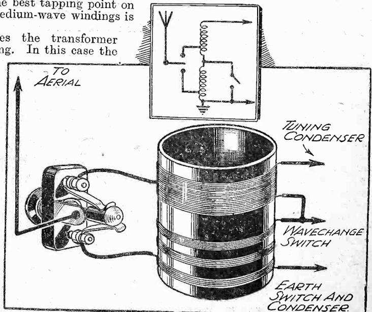
Fig. 2.—Tap method of aerial coupling.
