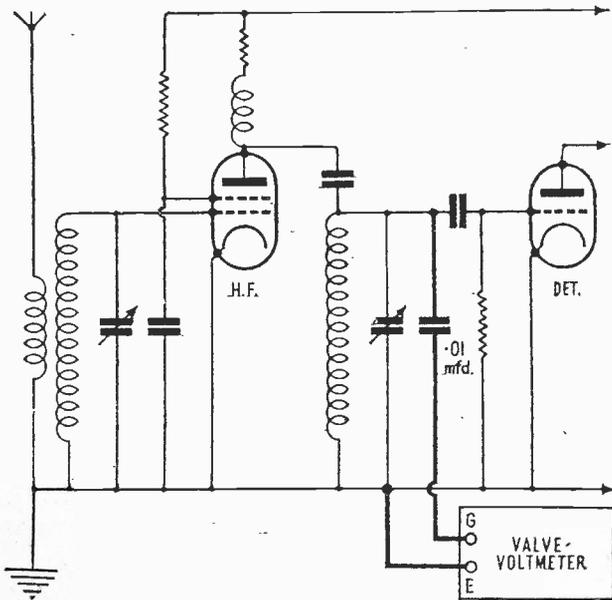
Fig. 1.—Method of measuring the voltage developed across a tuned circuit.
