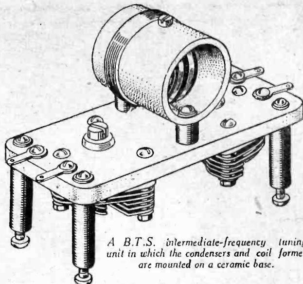
A B.T.S. intermediate-frequency tuning unit in which the condensers and coil former are mounted on a ceramic base.
