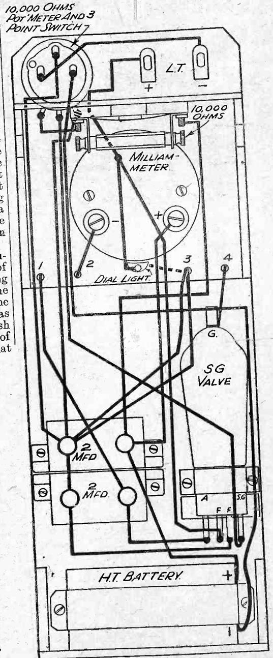
Fig. 3.—Wiring diagram showing all the connections.
