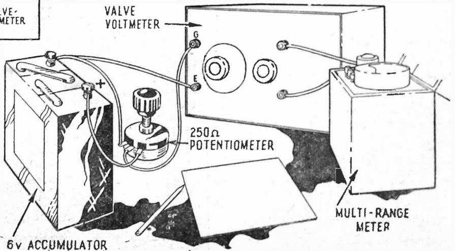
Fig. 2.—Adjusting the zero reading.
