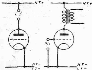
Fig. 2.—The output circuit of an S.W. set and the input circuit of an L.F. amplifier.
