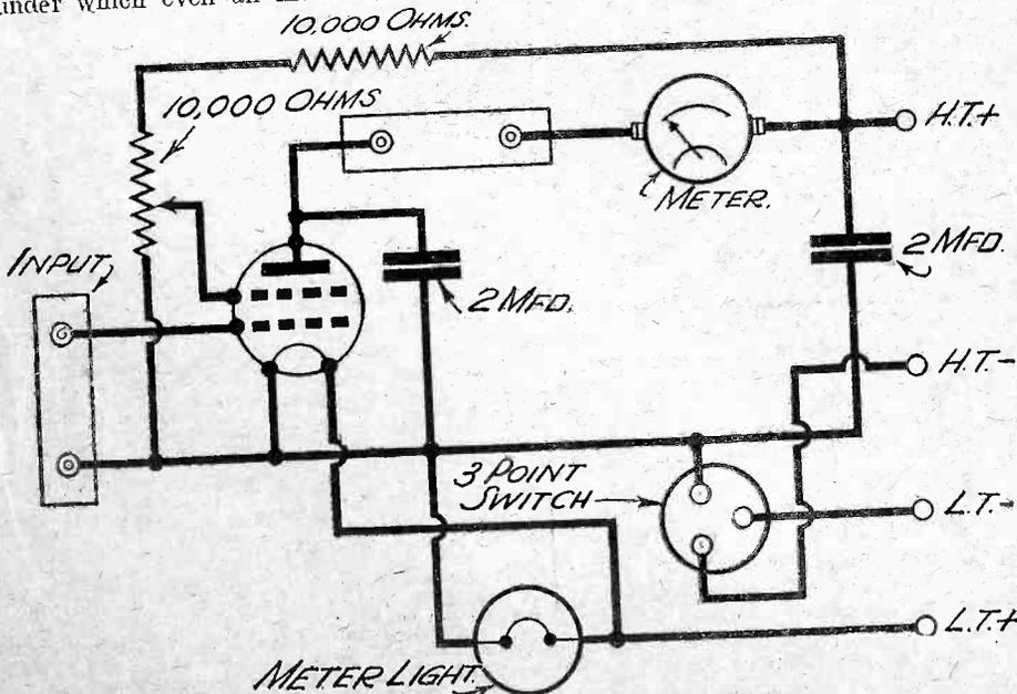
Fig. 2.—Theoretical circuit of the valve voltmeter.
