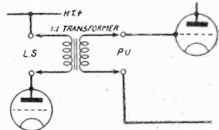
Fig. 4.—An alternative method of coupling the circuits shown in Fig. 2.
