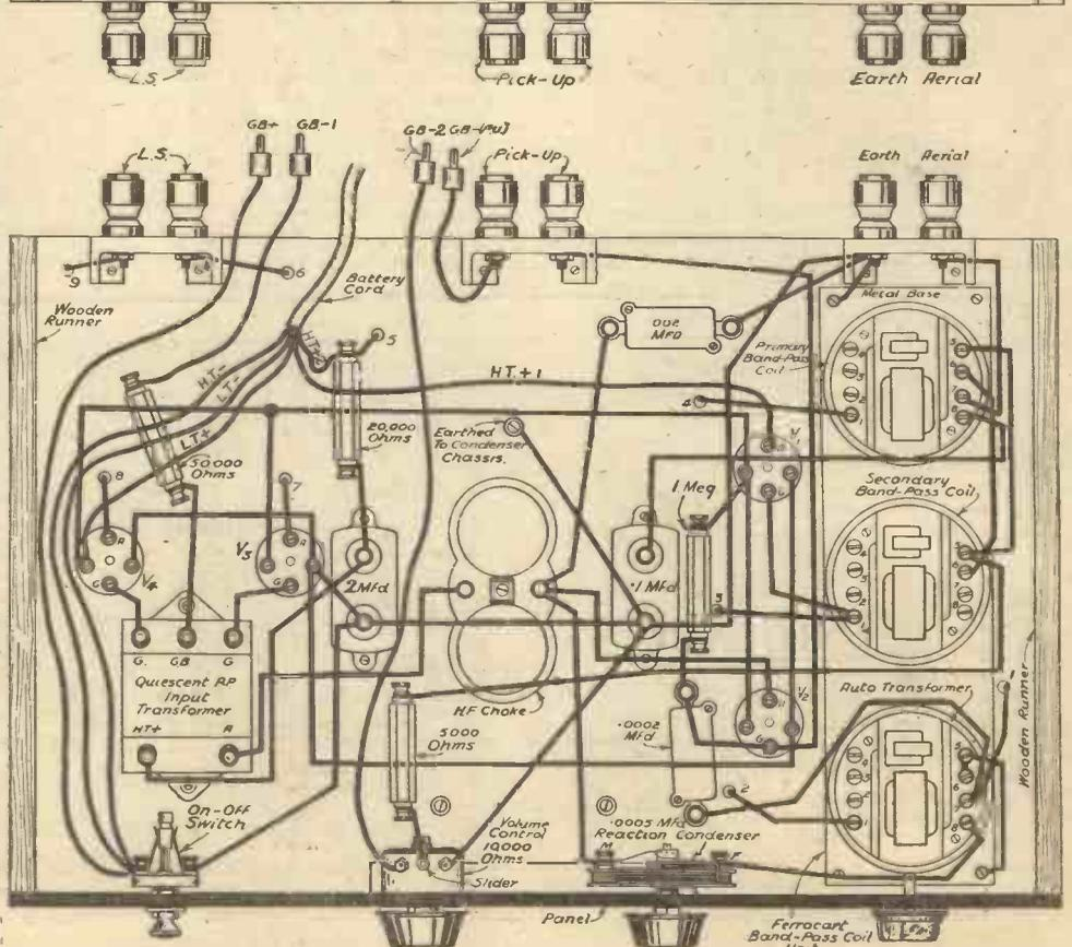
Top and sub-baseboard wiring of the Ferrocart Q.P.-P. Hi-mag Three.
