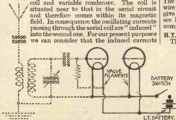
Fig. 5.—The filament circuit.
