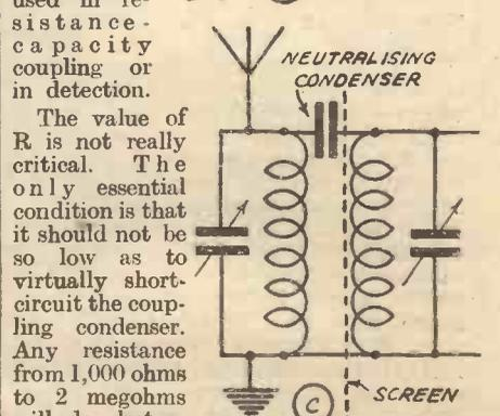
Fig. 5.—Various arrangements for capacitive coupling.
