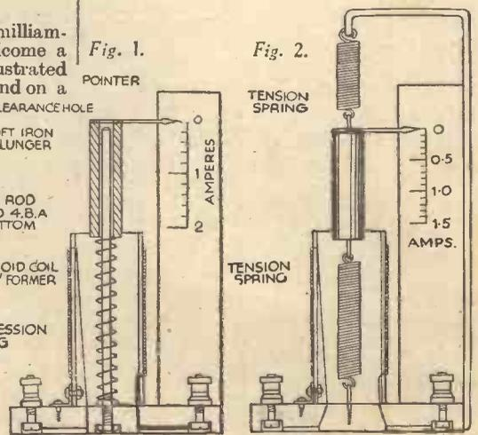
Two home-made high-reading ammeters.
