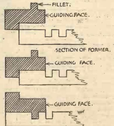
the slot cut, and you have a second guiding face which will keep the pitch of the slots constant. Another idea is to use two or three hacksaw blades in the frame at once. —W. ROWLANDS (Dalton-in-Furness).
