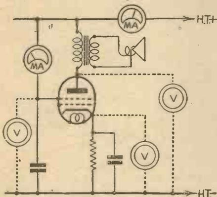
Fig. 1.—Testing a mains output pentode.
