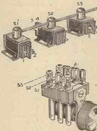
Fig. 5.—Two transmit-receive switch arrangements. The terminal numbers correspond with those in Fig. 4.
