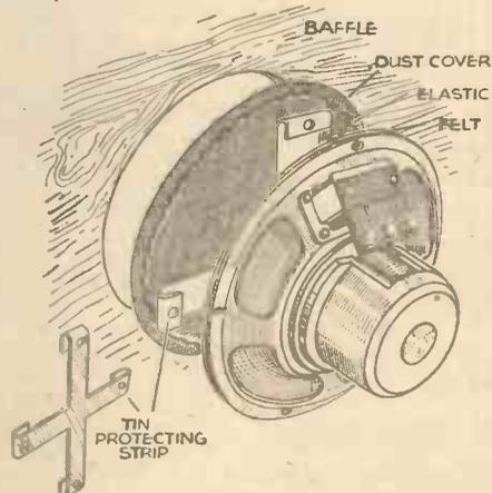
A novel fitment for protecting the cone and spider of a loudspeaker.
