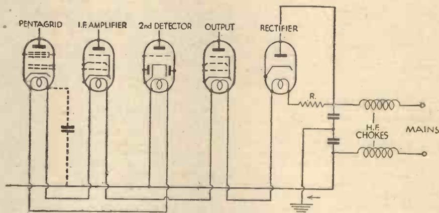
Circuit diagram showing the sequence of heater connections that is generally the most satisfactory for a universal superhet.
