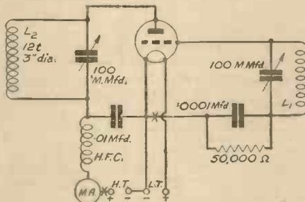
Fig. 6.—Circuit of the inexpensive transmitter described in a letter from Mr. V. H. Thomas.
