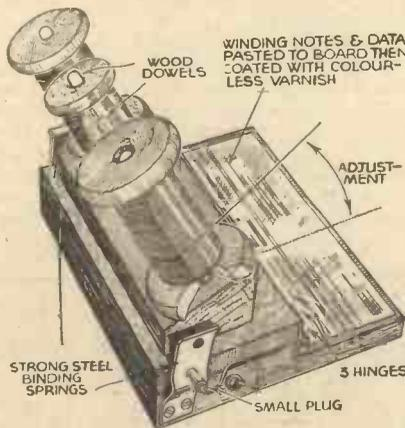
General view of an adjustable coil-winding stand.
