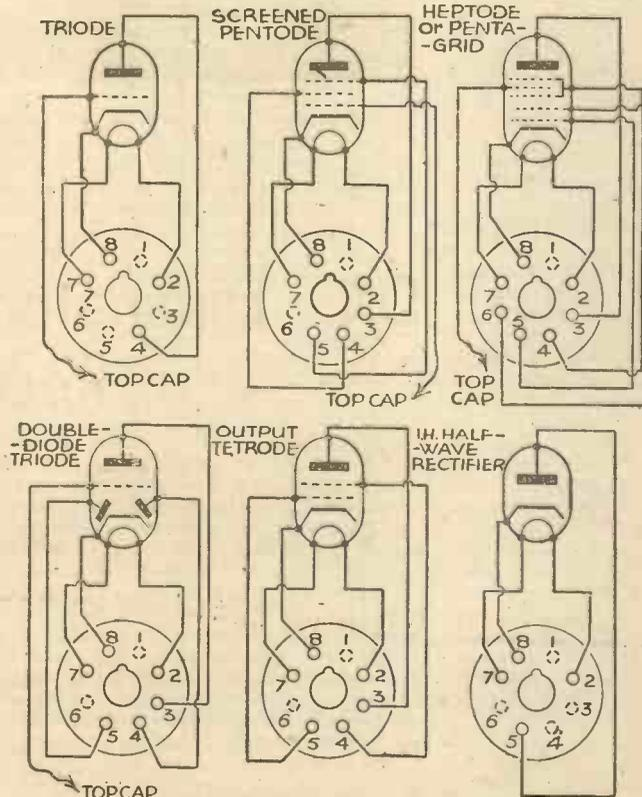
Fig. 2.—Under-base connections for a few typical "International" octal valves.
