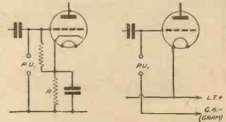
Figs. 71 and 72.—Connecting a pick-up in a detector stage—using a mains and a battery valve.
