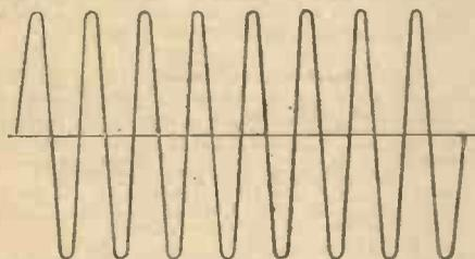
Fig. 1.—The simple wave-form of an unmodulated carrier.
