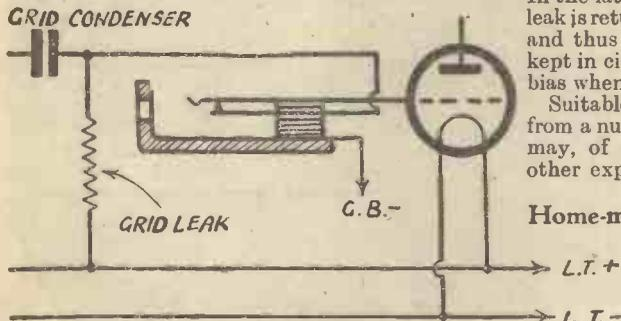
Fig. 1.—How to use a jack for pick-up switching in a battery circuit.
