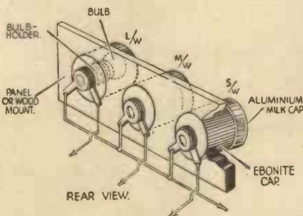
this purpose, fitting over the ebonite caps snugly. The fitment is wired to the wave-change switch contacts as shown in the theoretical circuit drawing.
