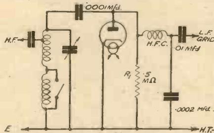
Fig. 2.—This skeleton circuit is of the same general form as that in Fig. 1, but applies to a diode used in a "straight" circuit, where the frame of the tuning condenser is earthed.
