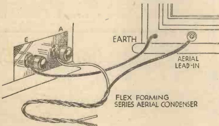
This simple dodge for providing a series aerial condenser is useful when no spare condenser is at hand.
