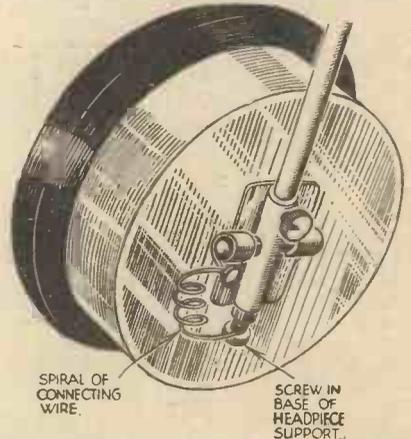
A method of preventing cracking in headphones.
