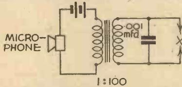
Fig. 2.—Connections for a microphone and microphone transformer to provide the audio frequencies.
