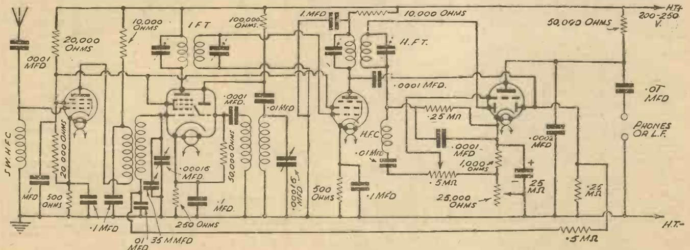
This is the superhet circuit referred to above. It is not necessarily complete in every detail, but gives sufficient data for experienced constructors.
