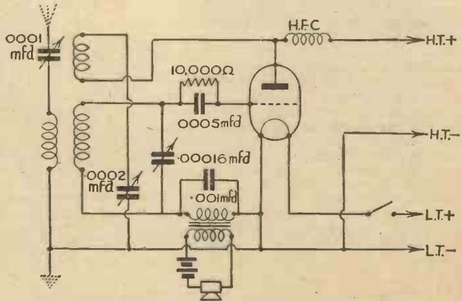
Fig. 3.—The similarity between this simple transmitting circuit and the receiving circuit shown in Fig. 1 is obvious. Aerial and earth are shown broken because these will be replaced by a "dummy" aerial when a full transmitting licence is not held.
