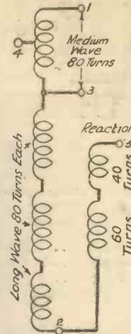
Fig. 3.—Wiring data for a broadcast coil with reaction and aerial tap.
