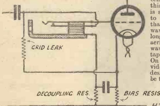
Fig. 2.—This diagram shows the same type of jack used for pick-up switching in a mains circuit.
