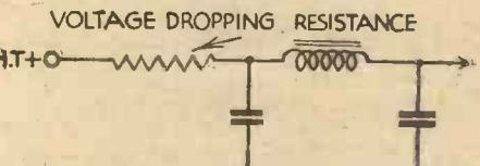
Fig. 2.—A voltage dropping resistance is sometimes included in the H.T. positive lead as shown here.
