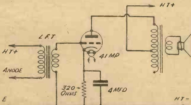
Fig. 2.—A simple L.F. amplifier circuit of conventional type, using a single 41 M.P. valve. Note that the bias resistor has twice the value of that used in Fig. 1.
