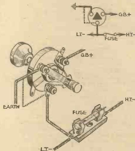
Fig. 4.—When a variable-mu valve is used, as shown in Fig. 3, the existing two-point on/off switch may be replaced by a three-point component adopting the connections shown above. In some cases the H.T.— lead may be joined direct to earth. The original two-point connections are indicated by the broken line.
