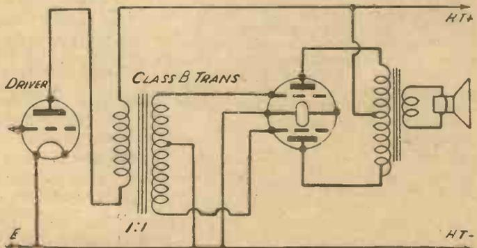
Fig. 3.—Skeleton circuit for a Class B output valve with driver
