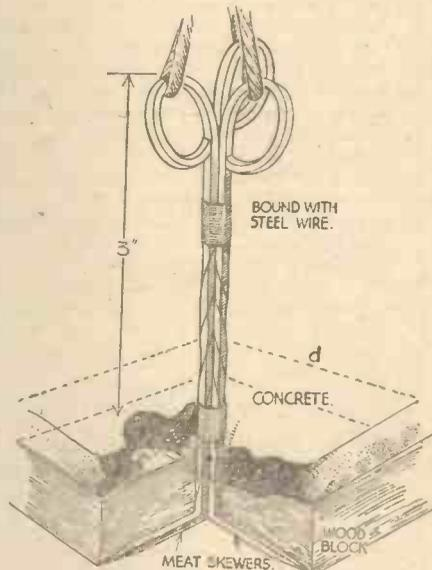
Method of arranging an anchoring hook for a vertical single-wire aerial.
