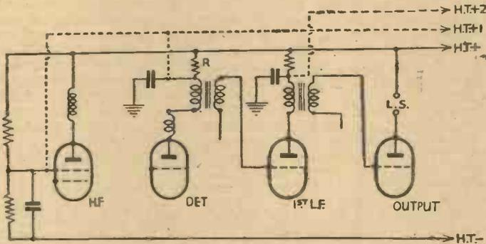
leave the voltage which is required as indicated by the battery tests. For the benefit of those who are not familiar with the method of working out such resistance values it may be mentioned that the simple formula of Ohms Law is used, the voltage required at the anode being deducted from
