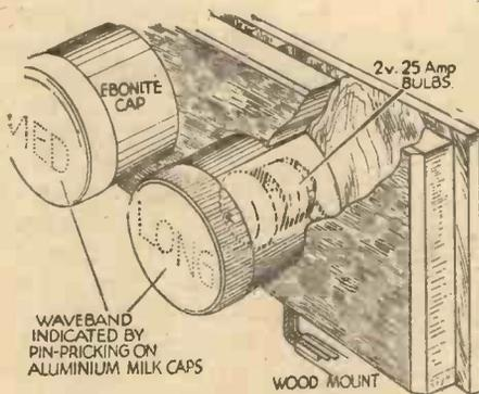
Front and rear views, and diagram of connections for a simple wave-band indicator.
