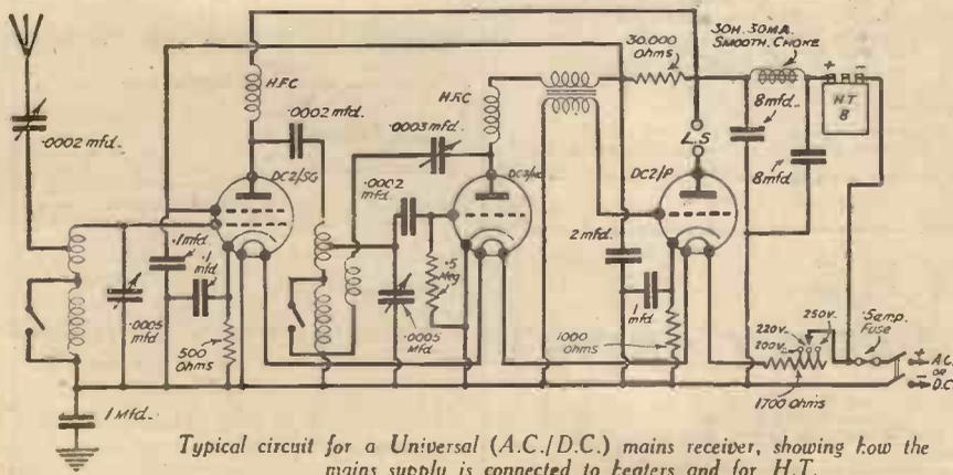
Typical circuit for a Universal (A.C./D.C.) mains receiver, showing how the mains supply is connected to heaters and for H.T.
