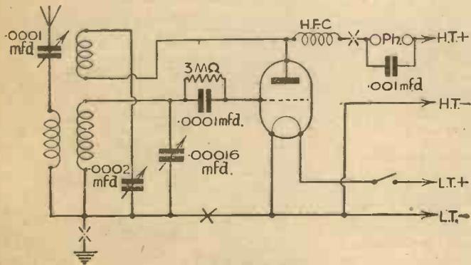
Fig. 1.—A normal type of single-valve S.W. receiver. Points at which audio frequencies can be injected are marked X.
