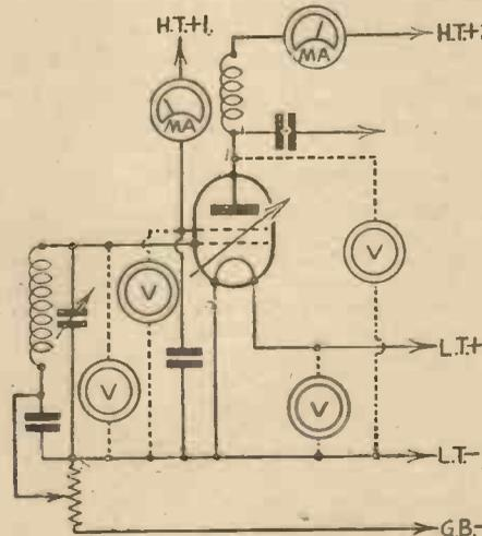
Fig. 2.—Testing a variable- $\mu$  H.F. pentode or screen-grid valve.
