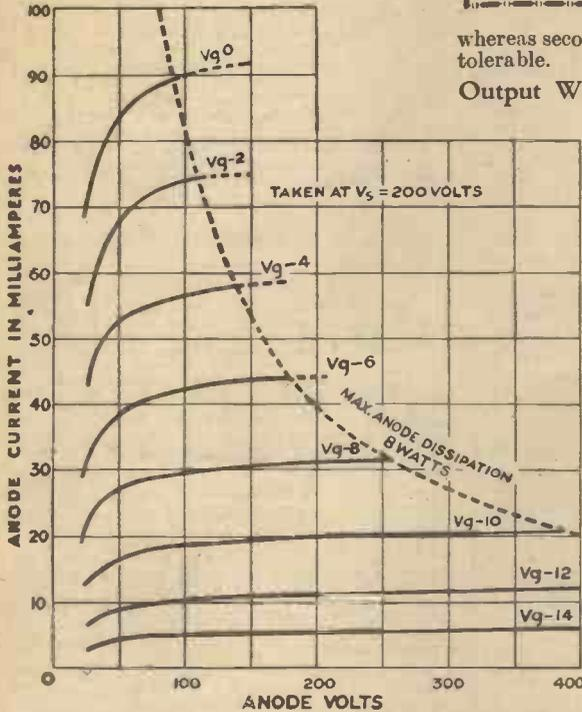
Fig. 1.—A typical example of an anode-volts/anode-current curve from which the undistorted output is calculated.
