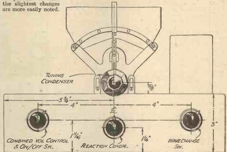
Dimensions for drilling a panel or cabinet for the Triband Three.
