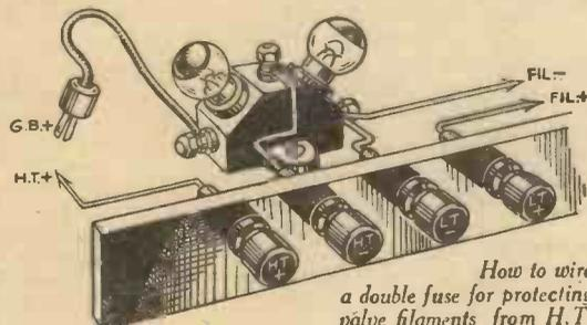
How to wire a double fuse for protecting valve filaments from H.T. and G.B. shorts.
