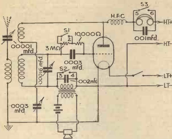
Fig. 4.—How receiver and transmitter circuits can be combined by using a simple switching system.
