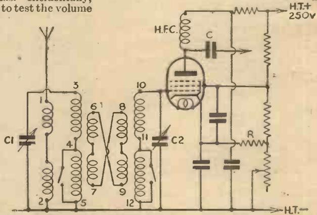
Fig. 3.—A typical H.F. stage with band-pass tuning employing a variable- $\mu$  H.F. pentode (mains type).
