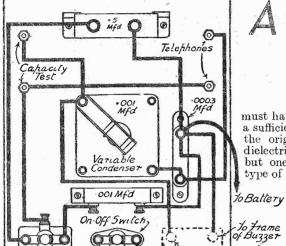
Fig. 1.—Wiring diagram of the simple capacity tester.
