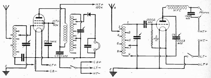
Fig. 2.—The H.F. transformer system of inter-valve coupling is shown in this circuit.
