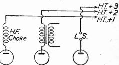
Fig. 2.—A skeleton standard 3-valve circuit showing normal anode connections.
