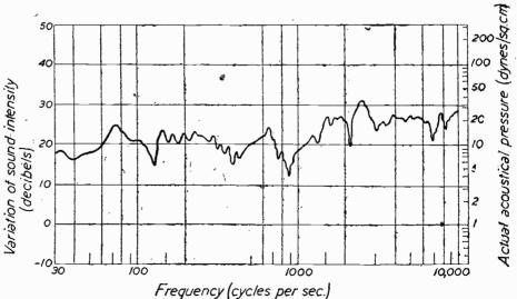
Fig. 3.—A scientific method of plotting a response graph for a high-grade loudspeaker. This is detailed" than usual, for in most cases the graph is drawn as a smooth curve.
