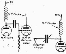
Fig. 2.— Aperiodic Fig. 3.—The stan-H.F. coupling includes dard reaction H.F. a choke as shown here.
