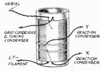
Coil connection details for the Gas-mask Box Receiver.
