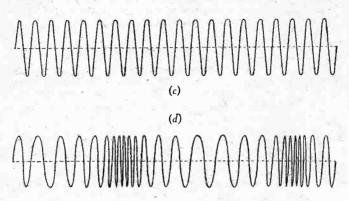
(c) is the carrier and audio wave combined in Amplitude Modulation, whilst (d) is the same combination in Frequency Modulation.
