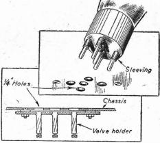
A novel method of fitting sub-chassis valveholders
