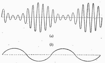
(a) Is a radio carrier wave of constant amplitude; and (b) is a programme or audio wave for modulating (a).
