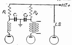
Fig. 3.—The arrangement of Fig. 2, plus decouplers
