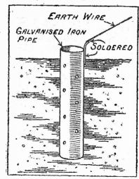
A piece of galvanised iron pipe makes an efficient earth tube.
