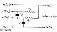
Fig. 4.—How to arrange for the decouplers shown in Fig. 3, so that they may be included between the receiver and mains unit.
