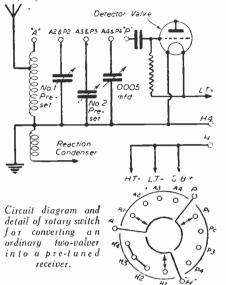
The wire from the grid condenser to the to the pole feeds marked "A" and "P" respectively. The grid end of each con-denser (1 variable, 2 pre-set) is taken to contacts on "A" pole and "P" pole, as shown.
