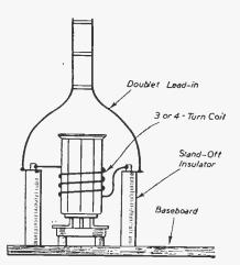
Method of using a doublet aerial with a 4-pin coil, as described by J. Hunter.
