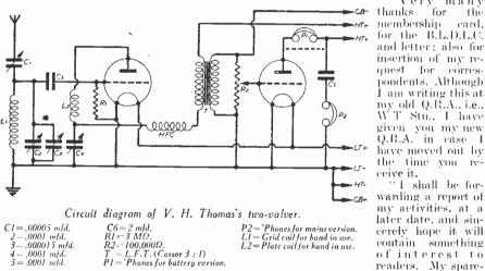
P2= 'Phones for mains version. L1 = Grid coil for band in use. L2= Plate coil for band in use.
