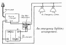
per) was carried out with wire from old two-pin plug-in coils, and ordinary screwin dial-light pattern 6 v. bulbs are used. To add to the appearance of the actual lights, they are housed in the "half-hexagon" type shades, which were purchased from a cheap stores. Other details will be seen from the sketch.—B. A. WHEATLEY (Bridgwater).
