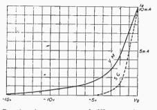
Fig. 1.-A representative Ia-V9 curve for a variable-mu valve. It shows that the "slope reduced with increasing negative bias. A broken line shows a corresponding curve for a "plain" S.G. type of value.
