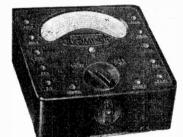
THE UNIVERSAL AVOMINOR ELECTRICAL MEASURING INSTRUMENT **22 Ran D.C. Volts** 0- 75 millivolts 0- 5 volts 0- 25 22 Ranges of Direct Readings
