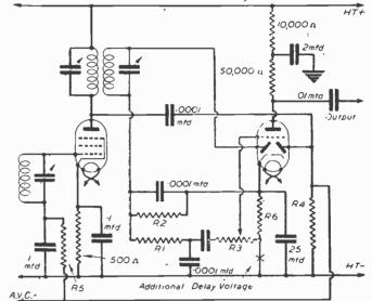
Fig. 6.—An arrangement similar in principle to that shown in Fig. 5, but using mains values and a double-diode-triode for second detection, A.V.C. and L.F. amplification.
