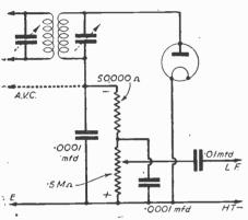
Fig. 4.—A more practical form of the circuit shown in Fig. 3. It includes an H.F. filter.
