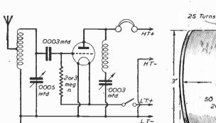
Theoretical circuit of M. Lockwood's single-valver, and details of coil.
