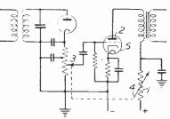
Fig. 2.—Circuit diagram of a diode rectifier and L.F. amplifier stage.
