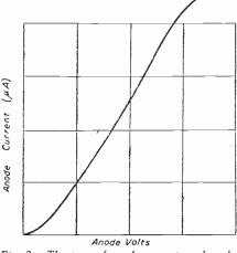
Fig. 2.—The type of anode current-anode volts curve obtained for a diode.
