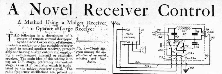
valve serves as output valve and oscillator valve, no switching of the control grid circuit is required, and since in the case of the screen-grid output valve the oscillatory tuned circuit may be maintained in circuit audio - frequency amplification, the for switching is simplified.
