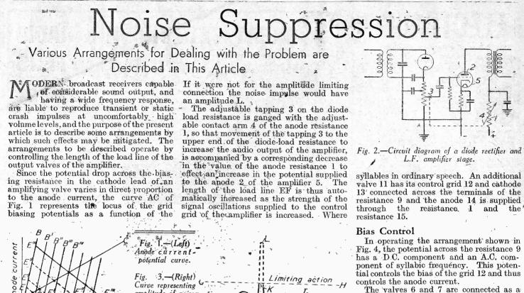
anode potential. The lines EF, E'F', etc., represent the load lines, the slope of which is a function of the output-circuit impedance determined by the particular valve employed. The anode swing of the valve is limited to the length of the line EF, E'F' (the length of which is a function of the anode potential) being limited at the abscissa axis by the anode-current cut-off; and at the line AB by grid current. Thus, the length of the load line may be controlled by adjusting the anode voltage.
