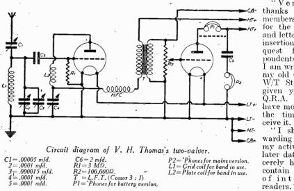
P2='Phones for mains version. L1=Grid coil for band in use. L2=Plate coil for band in use.
