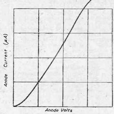
Fig. 2.—The type of anode current-anode volts curve obtained for a diode.
