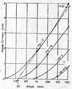
Fig. 4.—Anode current-anode volts curves for a battery triode of the "H.L." type. The chain line is used to find the anode resistance of the valve.
