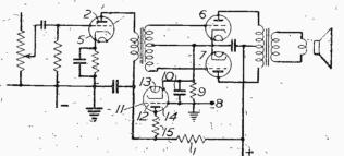
through a resistance 9 which is shunted by a condenser 10 having a capacity to provide a low impedance in comparison to that of a resistance at twice the lowest audio freresistance at twice the lowest audio ire-quency supplied to the amplifier, and yet to have a high impedance at syllabic frequencies. By syllabic frequencies are meant that range of frequencies from zero to approximately 30 c.p.s which is the frequency range of the occurrence of
