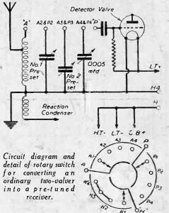
The wire from the grid condenser to the grid coil is broken and the two ends taken to the pole feeds marked "A" and "P" respectively. The grid end of each con-denser (1 variable, 2 pre-set) is taken to contacts on "A" pole and "P" pole, as shown.
