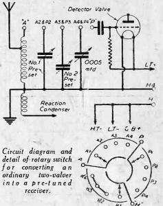
The wire from the grid condenser to the grid coil is broken and the two ends taken to the pole feeds marked "A" and "P" to the pole leeds marked A and F respectively. The grid end of each con-denser (1 variable, 2 pre-set) is taken to contacts on "A" pole and "P" pole, as shown.
