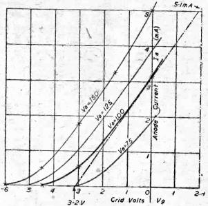
oltage Amplification Fig. 5.—Anode current-grid volts curves for a battery triede A point which is often over- of low mutual conductance. The latter is found by constructing a triangle as explained in the text.
