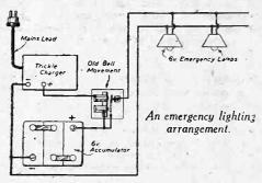
per) was carried out with wire from old two-pin plug-in coils, and ordinary screw-in dial-light pattern 6 v. bulbs are used. To add to the appearance of the actual lights, they are housed in the "half-hexagon" type shades, which were purchased from a cheap stores. Other details will be seen from the sketch.-B. A. WHEATLEY (Bridgwater).
