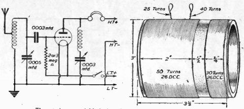
Theoretical circuit of M. Lockwood's single-valver, and details of coil.
