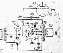
Fig. 6.-A modification of the circuit given in Fig. 5, showing how a high-mu value is incorporated
