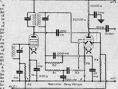
Fig. 6.—An arrangement similar in principle to that shown in Fig. 5, but using mains valves and a double-diode-triode for second detection, A.V.C. and L.F. amplification.
