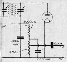
. 4.—A more practical form of the circuit hown in Fig. 3. It includes an H.F. filter.
