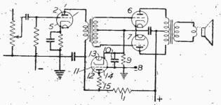
Fig. 4.—Circuit diagram of an output amplifier stage.
