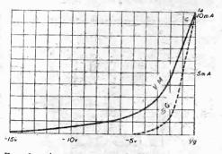
Fig. 1.—A representative Ia-V9 curve for a variable-mu valve. It shows that the "slope" is reduced with increasing negative bias. A broken line shows a corresponding curve for a "plain" S.G. type of valve.
