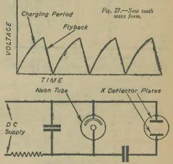
Fig. 28.-Neon tube time base.
