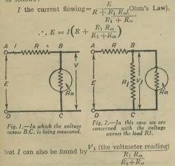
$$\therefore E = \frac{V_1 \left( R + \frac{R_1 R_m}{R_1 + R_m} \right)}{\frac{R_1 R_m}{R_1 + R_m}} = \frac{V_1 \left\{ \left( R_1 + R_m \right) \left( R + \frac{R_1 R_m}{R_1 + R_m} \right) \right\}}{R_1 R_m}$$
