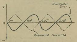
Fig. 109. -Quadrantal error and correction curves.
