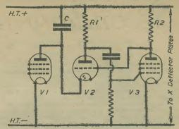
Fig. 30.-A hard value time base circuit.
