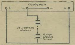
Fig. 1.—An output arrangement, for use with mercury vapour rectifiers, to enable 24 2-volt cells to be charged.
