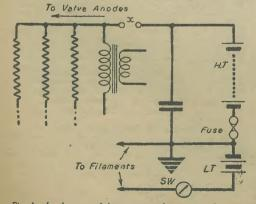
Fig. I.—In the case of ballery-operated receivers, the power supply takes the simplest form as shown here.
