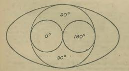
Fig. 106.—Effect of combining loop and straight aerial voltages having a phase difference of 90 deg.
