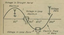
Fig. 105 .- Phase difference between loop and straight aerial voltages.
