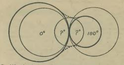
Fig. 107.—Aerial effect produces resultant polar diagram depending on relative phase of loop and aerial voltages.
