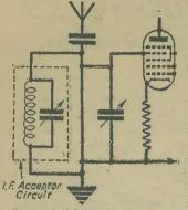
Fig. 2.—An I.F.-tuned acceptor circuit connected between aerial and earth terminals of a superhet to prevent birdies."
