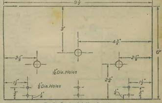
Fig. 2.-Panel and drilling dimensions.
