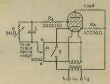
Fig. 3.-Basic time-delay circuit
