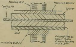
Fig. 2.- A metal rectifier unit assembly.
