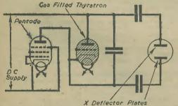
Fig. 29.-The circuit of a thyratron time base.
