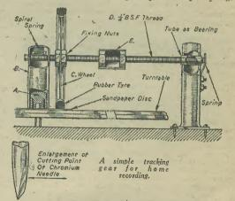
This method gives a track of approximately 50 grooves to the inch as compared with 100 on commercial records. D is threaded with in. B.S.F. thread with 25 turns to the inch.
