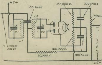
Fig. 8 .- A convenient type of discriminator circuit.
