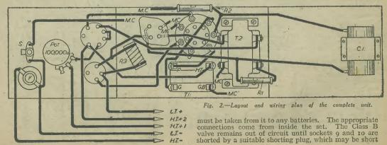
lengths of flex complete with two plugs. Sockets 8 and o are shorted only if the filament resistance is not needed.
