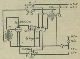
Fig. 1.- The circuit of the L.F. oscillator, together with the amplifier section.
