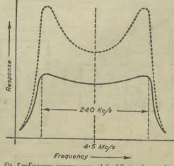
Fig. 5.—Frequency response curves of the I.F. transformer when damped and undamped.
