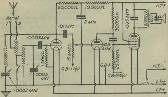
Fig. 1.-The theoretica? circuit of the receiver.
