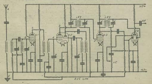
Skeleton circuit diagram of a superhet illustrating testing points referred to in this article.
