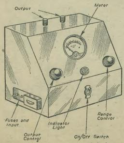
Fig. 3 .- The general layout of the unit made by the writer.
