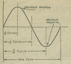
Fig. 2.—Shows graphically the manner in which an alternating voltage or current varies during one cycle.
