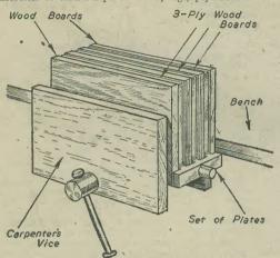
Fig. 1.-A set of plates, with plywood pieces in position, being straightened in a vice.
