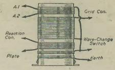
Fig. 6.—Showing location of and the connections for the coil windings.
