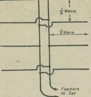
Fig. 3.-A stacked dipole or broadside aeria!
