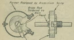
Contact Arm Bent to Fit into Grooves Side elevation of the bandsetter.
