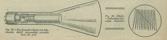
time within the beam and so produce a column of positive charge along it. This has the effect of drawing the outside electrons in towards the centre of the beam.
