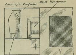
Fig. 4.—Rear view of Fig. 3, showing sliding door and part of assembly.
