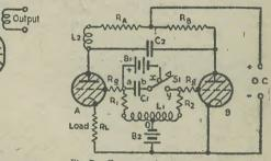
Fig. 7 .- Generator of square-wave single pulses.
