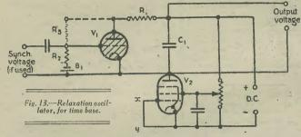
Relaxation Oscillators.—When applied to relaxation oscillators the thyratron has a great advantage over the neon tubes first employed, owing to the much greater range available between the extinction voltage and voltage at which the arc can be struck, the latter being under the control of the bias applied to the grid. If the charging resistance is replaced by a pentode, which acts to maintain the charging current constant, a linear relation between time and condenser
