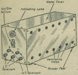
Fig. 3.—The completed mains unit as assembled by the writer. Note the well-ventilated protecting metal cover.
