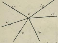
Fig. 3.—Currents flowing to and from a point, demonstrating the first law.
