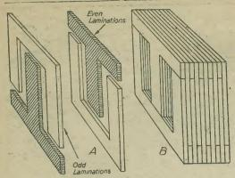
Fig. 5.—Method of interleaving stampings.
