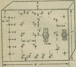
Fig. 5.—Layout and drilling template of the panel. Dimensions of a suitable case are also shown.
