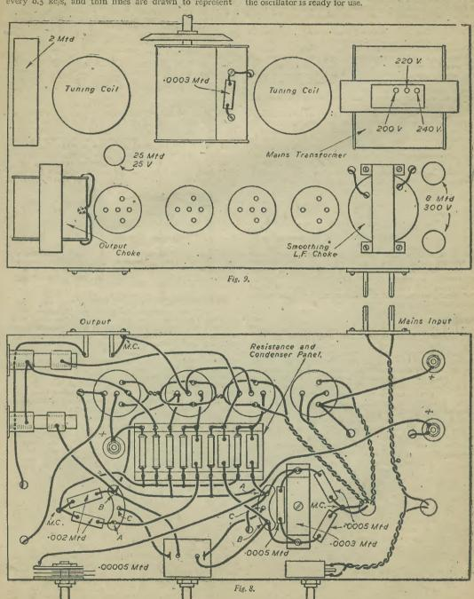
Figs. 8 and 9.—Layout and wiring diagram. Resistance and condenser valves, reading from left to right: 1,000 Ω; 1 MΩ; 50,000 Ω; 1 MΩ; .0001 mfd.; 50,000 Ω; .01 mfd.; 1 MΩ; .0001 mfd.
