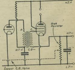
Fig. 4.—The normal arrangements for automatic grid-bias with battery operated valves.
