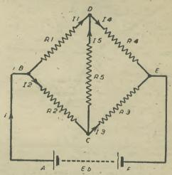
Fig. 2.—The additional resistor R5 which complicates the circuit of Fig. 1.
