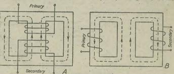
Fig. 2.—Shell-type construction.
