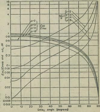
Fig. 22.—Critical inductance and direct output voltage as a function of delay angle. p == number of rectifying phases.
