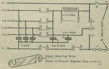
Fig. 2.—The theoretical circuit of the unit described in this article, together with a simple form of shorting strip.
