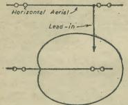
Fig. 4.—(Left) Exaggerated potar diagram (below), of a horizontal inverted aerial (above).
