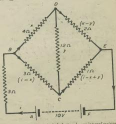
Fig. 5. - An example in which the battery has an internal resistance of 3 ohms.
