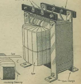
Fig. 6.—Three stages in the winding of coils.
