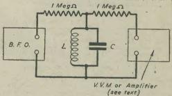
Fig. 5.-Method of coupling the B.F.O. and the amplifier
