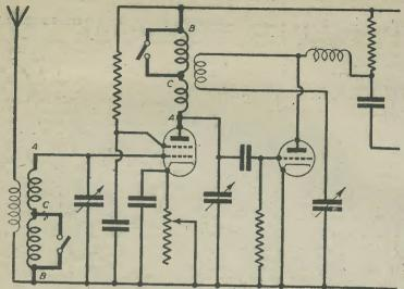
Fig. 4.-Windings and connections to be retained using two typical coils.
