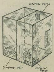
Fig. 2.-Method of repairing leaky containers.
