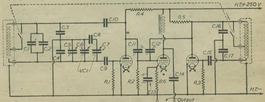
Fig. 3.—Circuit diagram of the beat-frequency oscillator; C1 .0003 mfd. preset; C2, C3 and C4, .0005 mfd. fixed; C5, .0005 mfd. set zero; VC1 (C6, C7, C8) .0007 mfd.; C6, C7, .0005 mfd. ganged; C8, .0003 mfd. fixed; C9, C15, .0001 mfd. fixed; C10, .01 mfd.; C11, C12, 10 mmfd. preset (see text). C13, 25 mfd. 25 v. fixed; C14, 2 mfd.; C16, C17, .002 mfd.; R1, R2, R3, 1.0MΩ; R4, R5, R6 depend on valve used (see text).
