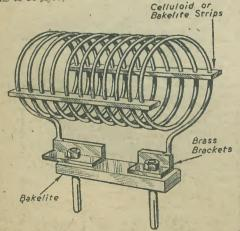
An air-spaced coil of 16-gauge wire, wound double, and threaded through bakelite supporting strips.
