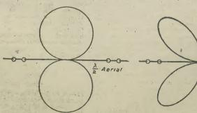
Fig. 2.—Polar diagram of a free-spaced (no: earthed) half-wave aerial.
