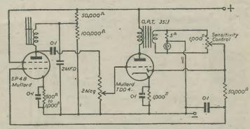
Fig. 3.—The complete circuit, including the amplifier. The exploring stack of laminations is shown in the anode circuit of the SP4B Mullard valve. Circuit constants should be adhered to. If other valves are used, cathode bias resistors must be correspondingly changed in values. Operating potentials are dependent upon the types of valves employed.
