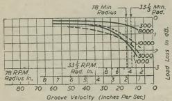
Fig. 3.—Shows cutting load loss, with R.G.A.MI-11850 head, and lacquer-coated disc.
