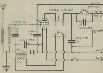
Fig. 11.—A simple reflex circuit.
