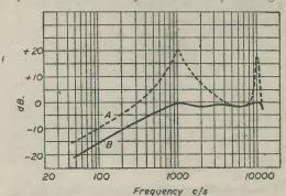
Fig. 2.—Frequency response of damped and undamped cutting-head. A is without viscoloid damping block, and B is with damping block inserted.
