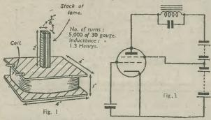
Fig. I shows the most interesting component of this new device, the coil to be tested having to be placed over the stack of laminations. The wire is wound on a bobbin with presspahn flanges to keep it snug. Insulated wedges assure rigidity. Fig. 2 shows the basic circuit of the dynatron oscillator.
