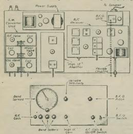
Fig. 3.—Suggested layout of the complete superhet.
