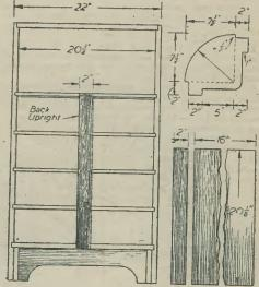
Fig. 4.—A back view of the carcase, with details of the lid.
