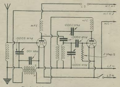
Fig. 16.—A reflex circuit employing a valve for detection.
