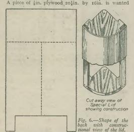
This is first glued and panel nailed to one of the cross-rails and bent (unglued) over to the second cross-rail. This will be easy, owing to the shortness of the grain. It only remains to brush on glue, bend the wood over and add a panel nail here and there to hold it down.
