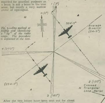
After the two letters have been sent out for about 30 seconds, a different type of keying comes into operation and this causes a two-letter call-sign to be radiated, first by the "N" aerial loop, and then by the "A" aerial loop. The call-sign is radiated for two reasons. The first is to identify the particular radio range so that the pilot can tell, by looking at his chart, precisely where
