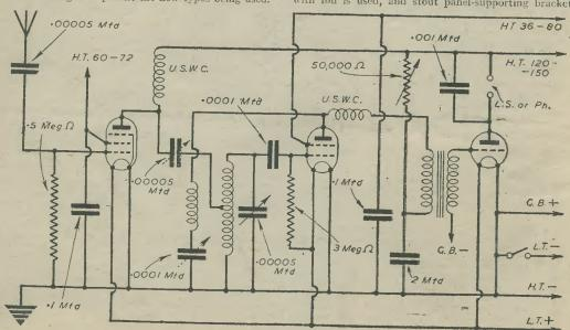
Fig. 1 .- Theoretical circuit of the receiver.
