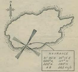
Fig.2.—On a map showing radio navigational aids a typical radio range would be shown as illustrated here, where the radio range is a hypothetical one on an imaginary island in mid-Atlantic. The range is situated at an airfield called "Navrange," and operates on a frequency of 262 kc/s. with the identification letters AB. The "A" sectors are between 020 degrees—127 degrees and 220 degrees—280 degrees; the "N" sectors are between 127 degrees—220 degrees and 280 degrees—020 degrees.
