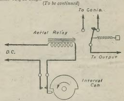
Fig. 12.—The interval cam runs at half the speed of the identification cam, connecting the transmitter output first to one aerial and then to the other while the two-letter identification is sent out. In practice, the contacts of all three cams are interconnected and the cams are operated through a somewhat complex system of gears.
