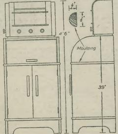
Fig. 1 .- A front and side elevation, with receiver in position.
