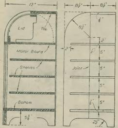
Fig. 2.—Sectional side view, with shape and size of one side, showing the position of the grooves or trenching for shelves, etc.
