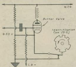
Fig. 11.—The identification cam, which automatically keys the transmitter with a two-letter call sign, operates a pair of contacts which open and close the bias circuit to the buffer valve connected between the R.F. oscillator and the intermediate amplifier stage.
