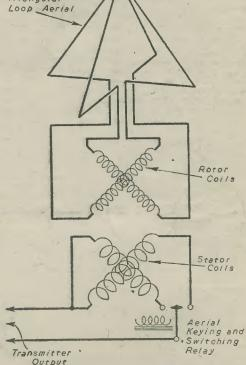
Fig. 6.—The arrangement of a Bellini-Tosi loop aerial system and associated radio-goniometer. The pair of stator and the pair of rotor coils are rigidly mounted at right-angles, while the rotor is free to rotate within the stator; a 360 degree scale is provided to indicate the position of the rotor.
