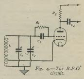
C1-.0005 mfd. preset. C2-25 mmfd. variable. C3-.0003 mfd. C4—Approximately 5 mmfd. R1—50,000 ohms. R2—20,000 ohms.
