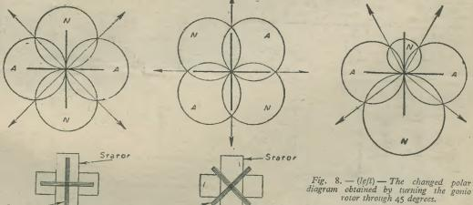
Fig. 7.—The theoretical radiation pattern from the crossed aerial loops when the stator and rotor windings of the goniometer are parallel to each other (gonio scale reading 360-0 degrees).
