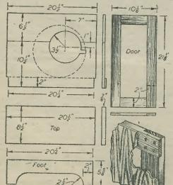
Fig. 3.—Size and shape of motor-board, top, foot and door-frame, with details of the door construction.
