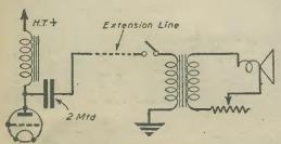
Fig. 2.—A volume control fitted at the extension point.
