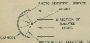
Fig. 1.—The principle of the photo-electric cell.
