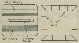
Fig. 6.—Top view of cabinet, Fig. 7.—Frame for winding showing position of aerial a pancake aerial. and carrying handle.
