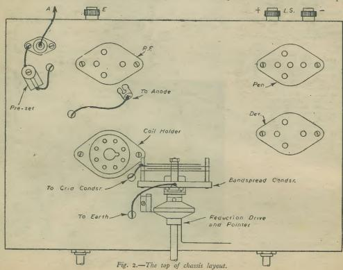
goes to the grid of the R.F. valve. The anode lead goes to tag r of the coil holder, and the band-spread capacitor is connected in parallel with the .00015 mfd. component below the
