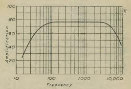
Fig. 4.—Frequency response curve of a typical amplifier.
