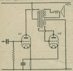
Fig. 1.—The output transformer with additional secondary winding to feed the second value.
