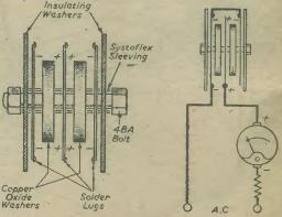
Details of the A.C. meter rectifier.
