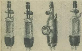
Fig. 3.—Photo-electric cells having a cathode in the form of a rectangular plate, centrally sealed in the bulb and brought out to the screw terminal at the top.
