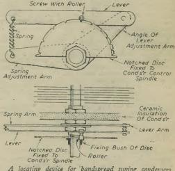
A locating device for bandspread tuning condensers (Mr. P. Redman).
