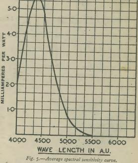
This cell, therefore, can be used for the detection or measurement of radiation from the already specified end of the spectrum. It is well to mention, however, that the sensitivity of this cell can be secured by increasing the positive potential, though extreme care must be taken not to exceed the value laid down by the manufacturer, otherwise a glow discharge will result and so ruin the cell.
