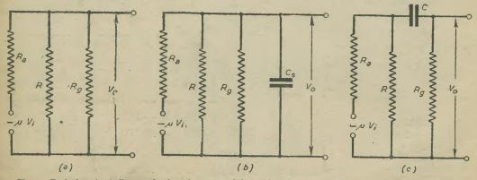
Fig. 5.—Equivalent circuit diagrams for the resistance-coupled amplifier for medium, high and low frequencies respectively.
