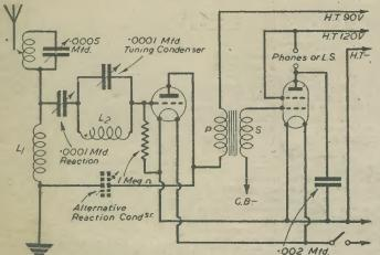
Fig. 6.—Fig. 5 modernised; care should be exercised that L1 and L2 are kept at right-angles.
