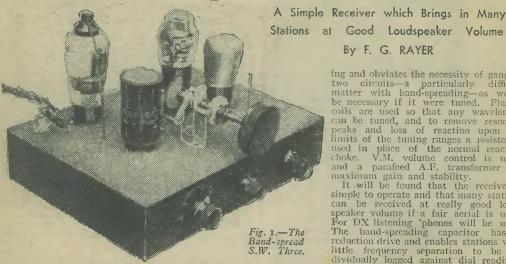
ing and obviates the necessity of ganging two circuits—a particularly difficult matter with band-spreading—as would be necessary if it were tuned. Plug-in coils are used so that any wavelength can be tuned, and to remove resonant peaks and loss of reaction upon the limits of the tuning ranges a resistor is used in place of the normal reaction choke. V.M. volume control is used, and a parafeed A.F. transformer for novinum resistant and etablished
