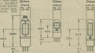
Fig. 2.—Typical designs of photo-electric cell having a rectangular-shaped cathode and rectangular wire loop for the anode.
