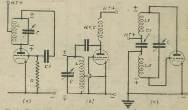
Fig. 6 .- Forms of Hartley Oscillator, which show clearly how the e.m.f. returned to the grid is of opposite phase to the anode voltage.
