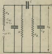
Fig. 3.—The practical resistance-coupled amplifier and its equivalent circuit.
