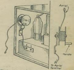
Fig. 6 .- How a frame aerial may be added to an ordinary receiver.
