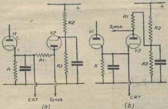
Fig. 21.—Diode separator circuits following immediately after a diode
