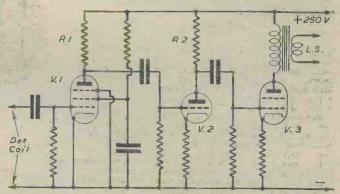
Fig. 2.—Result of eliminating certain of the decoupling components from Fig. 1.
