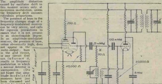
Fig. 4.—The basic circuit of a frequency-changer stage, used by the writer for 24-30 mc/s; decoupling condensers were all .05 mfd. (paper, except for the 8 mfd.) and all were shunted by .0001 mica. Resistance marked \* must be non-inductive. Valves used were 6K8 (triode-hexode) and 6K5 (triode).
