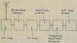
Fig. 1.—This block diagram shows the basic stages of a frequency-modulated superhed receiver.
