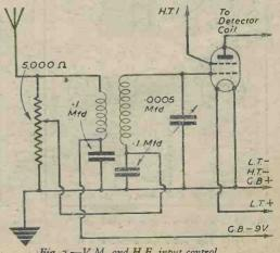
Fig. 2.-V.M. and H.F. input control.
