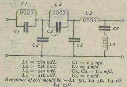
condensers can easily be made up and checked on a bridge.
