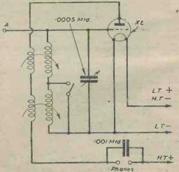
Fig. 3.—The circuit diagram of the pocket receiver.
