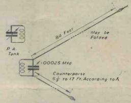
Fig. 2.—The W3EDP aerial, which is very efficient and may be folded to occupy small space without greatly impairing efficiency.
