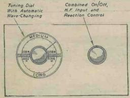
Fig. 5.—Showing simplification of ordinary T.R.F. receiver controls by system described.
