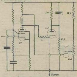
Fig. 26.—Another form of synch separator following an anode bend detector stage.
