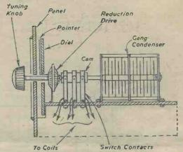
Fig. 6 .- Automatic wave-change switching.
