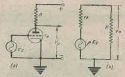
Fig. I.—Can "phase-reversal" be shown in Fig. I (b)?
