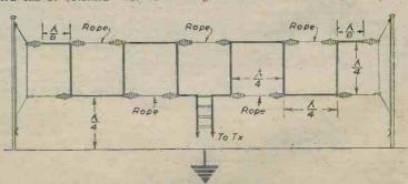
Fig. 5 .- A Bruce folded aerial-ideal if there is sufficient room to accommodate it with two or more wavelengths.
