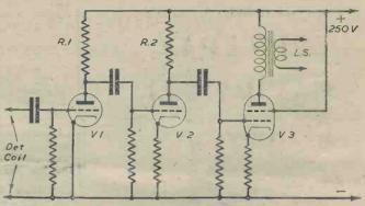
Fig. 3.—A similar circuit to Fig. 2 but with a triode input stage.
