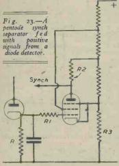
efficient diodes and lead to cleaner separation, but diode circuit is, nevertheless. practical proposition and will give excellent results when carefully designed.
