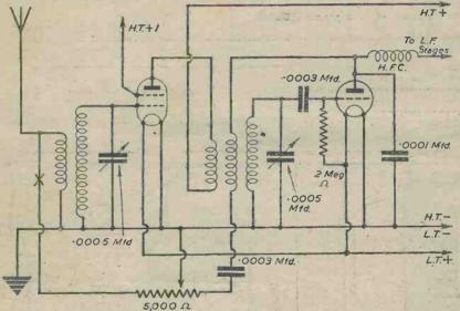
Fig. 1.—Combined reaction and H.F. input control.
