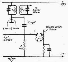
Fig. 6.—Typical circuit showing how the A.V.C. voltage is sometimes obtained from the anode of the last I.F. valve. In this case L2 is not included in the A.V.C. circuit.
