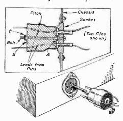
A plug which cannot be knocked out of its socket.
