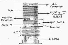
Fig. 1.—A simple dual-range coil.
