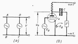
Fig. 2.—The E.M.P.s of two alternators in parallel are virtually in series opposition in the closed mesh ABCD. In the shunt-fed valve circuit (b), Z and ra are in parallel relative to Vo, but µEg still acts upon Z, ra and C regarded as a closed series mesh.
