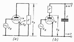
Fig. 1—A simple problem circuit. Are Z and ra in series or parallel?
