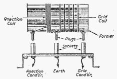
Fig. 8.—Plug-in short-wave coils with reaction windings.
