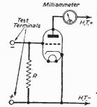
Fig. 1.—Circuit of simplified valve voltmeter which could be used to measure the A.V.C. voltage of a superhet. The resistance R is of a high value and might be omitted in this case.
