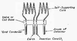
Fig. 7.—Another form of interchangeable U.S.W. coil.
