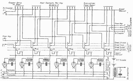
Fig. 1.—General scheme of the organ, illustrated by three octaves of the notes C and C sharp.
