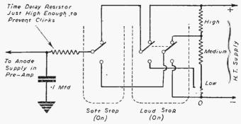
Fig. 2 .- Gaskell's two-stop, three intensity circuit. With Soft off and loud off output is O " low off ,, " medium off m " " high on
