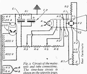
necessary to see that metal electrolytic condensers, with negative casing, are not automatically bolted to an earthed chassis. It is important, too, to notice that electrodes that are normally considered "safe" (valve cathodes, for instance) are now at a high negative voltage with respect to earth.
