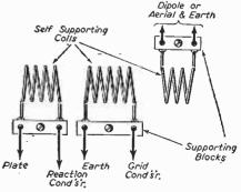
Fig. 6.—Ultra-short-wave coils may be made up as shown here.
