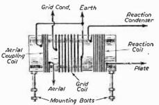
Fig. 5.—A simple short-wave coil.
