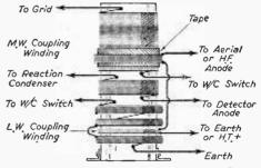
Fig. 2.—A dual-range coil of the H.F. transformer type.
