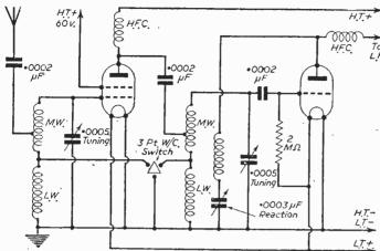
Fig. 3.—Simple circuit incorporating a pair of the coils of Fig. 1.
