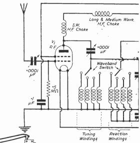
Fig. 1.—Theoretical circuit
