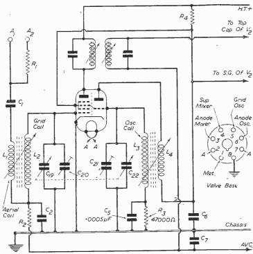
Fig. 1.—Original circuit of the F.C. stage of the Wartime Utility Receiver.
