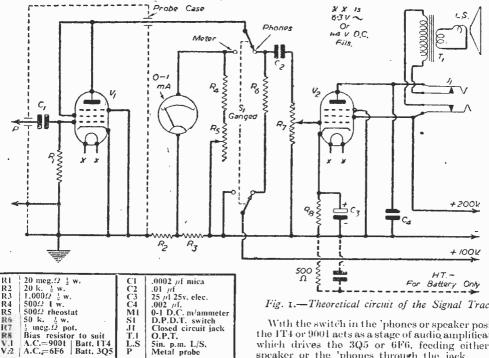
Fig. 1.—Theoretical circuit of the Signal Tracer.
