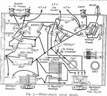
position the grid and reaction windings of one of the coils are connected. Fig. 4 makes this clear.
