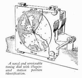
a boss with a grub screw was mounted on the tuning condenser spindle close up to the map.
