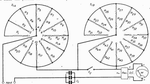
Fig. 2.—Circuit Diagram of the Output Meter described in this article.
