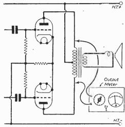
Fig. 4.—Measuring Output of a Push-pull Circuit.
