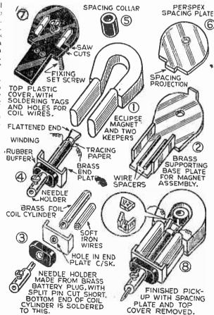
Fig. 2.—Main assembly details.
