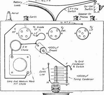
Fig. 2.—Above-chassis wiring details.
