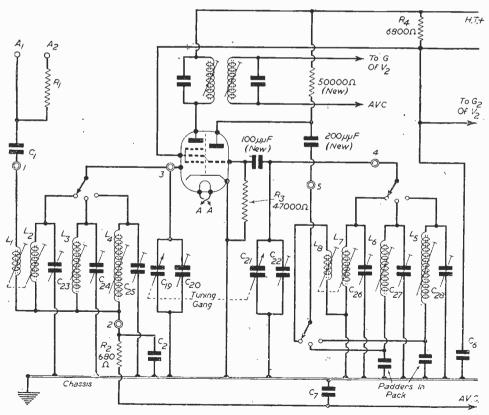
Note:  $\odot$  Indicates Connections To Soldering Tags On Pack. Switches Integral With Pack. Fig. 2.—Final circuit with new components and coil pack fitted.
