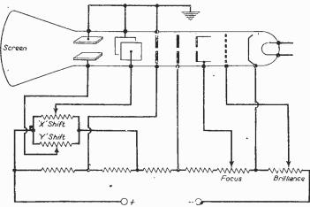
Fig. 1.—C.R.T. shift network, showing method of arranging X and Y shift controls.
